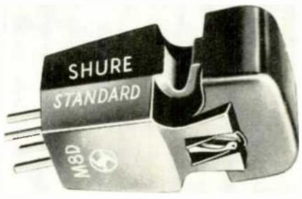
$3.0 \times 10^{-6}$  cm per dyne. Output voltage, 5 mv per channel at 1,000 cps. The cartridge has four terminals, but is adaptable to three-terminal arms. It has standard mounting centers of  $1\frac{1}{2}$ " and  $\frac{7}{16}$ ". Including a 0.7 mil diamond stylus. \$16.50. Shure Brothers, Inc., 222 Hartrey Ave., Evanston, Ill.
