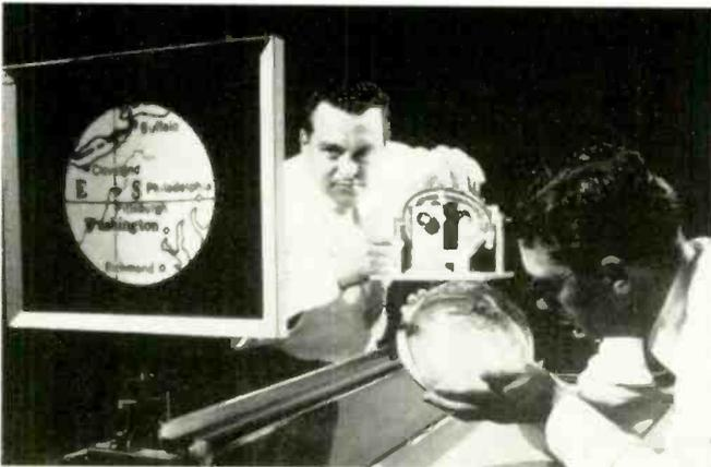
New air navigation system uses a computer to automatically position a map of half the earth in a glass hemisphere. The projection of a 400-mile diameter area (125,000 sq. mi.) on a 7 $\frac{1}{2}$ " screen pin-points the pilot's location. For space navigation, a stellar map would be used. IBM engineers R. W. Kern (l) and J. F. Creedon check out the system.
