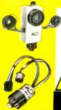
**Model C40 Adapter.** For use only with all previous B&K Model 400 and 350 CRT's. Tests and rejuvenates TV color picture tubes and 6.3 volt 110° picture tubes. Net, \$9.95
