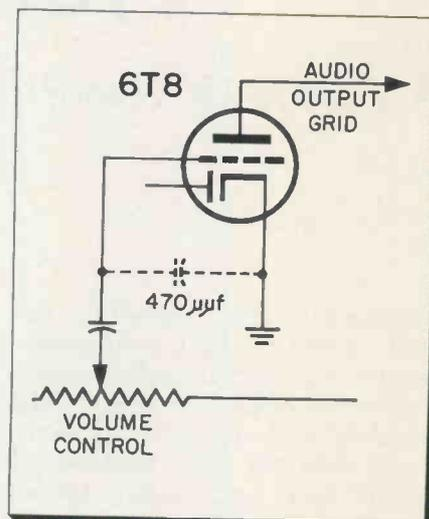
Fig. 2—Reader eliminates audio interference in RCA 21CS7815 color sets by installing a  $470\mu\text{mf}$  capacitor between grid and cathode of the first audio amplifier.
