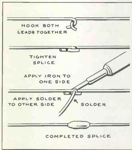
Fig. 2—The hook-splice is frequently helpful when replacing components which have been cut from a crowded terminal tie point.
