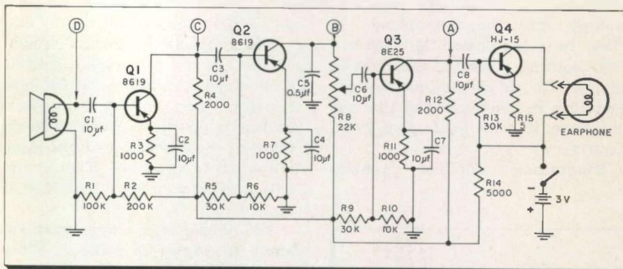
Fig. 4—Conny Model T-2 Hearing Aid that uses a conventionally-wired volume control circuit.
