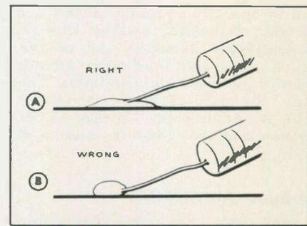
Fig. 4 (A)—A properly made chassis joint has a cohesive contour. (B) "Blob" type will not be electro-mechanically secure.
