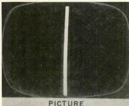
Fig. 1—*Misconception:* Bright vertical line can only occur with a r-f high voltage power supply. *Fact:* This can also happen in a flyback circuit.
