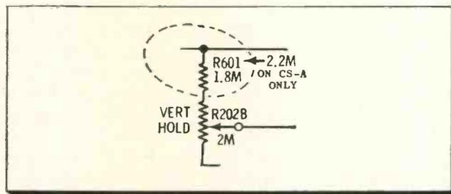
To recenter the vertical hold control's lock-in position on a Motorola TS-435 TV chassis, change the value of the resistor in series with the control from 2.2 megs to 1.8 megs.
