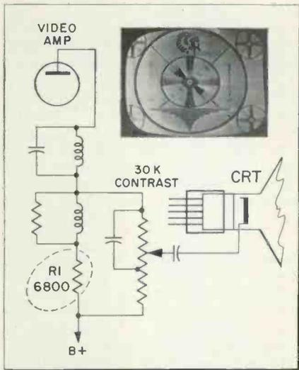
Fig. 4—Misconception: A "milky" picture when the brightness control is turned up is always caused by a defective CRT. Fact: Many TV chassis using the illustrated circuit have been known to cause a milky CRT if the plate load resistor opens.
