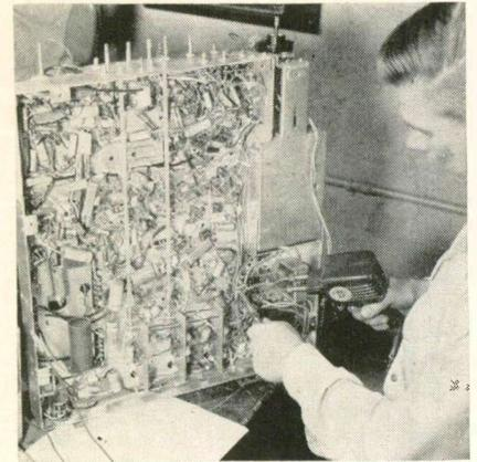
except in special cases), the process should be repeated. If a joint is properly heated, and solder applied directly to the joint, solder will flow into every crevice (through capillary action) and the highly desirable true alloyed joint will result.
