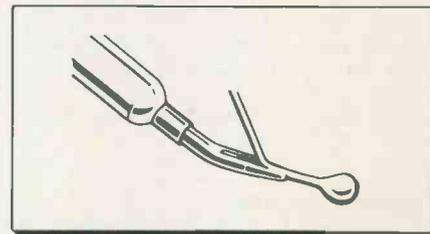
Fig. 3—An offset slotted iron triplet can be used to draw off excess solder from a terminal point. Solder flows into triplet notch.
