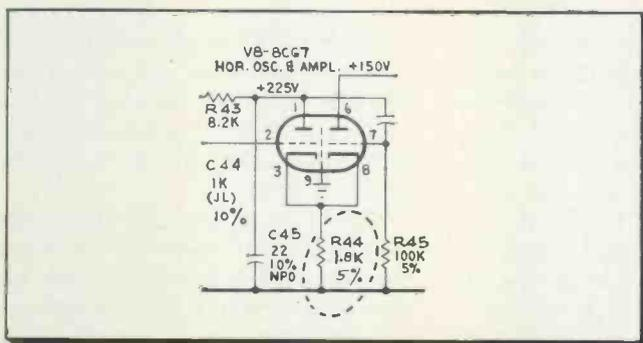
To eliminate a "Christmas Tree" effect in some Packard Bell V8-7 & -9 TV chassis, the circled 8CG7 horizontal oscillator's cathode resistor has been changed from 2200 ohms to 1800 ohms.
