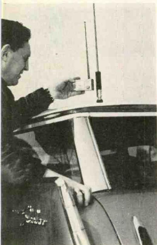
Technician Cooper holds field strength meter near base-loaded antenna to check out transmitter in Jacques' "wagon."
