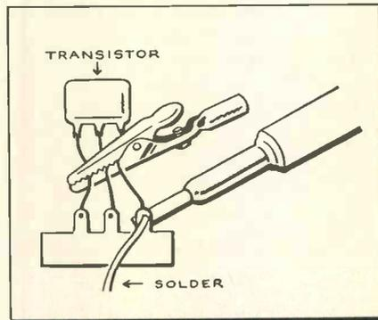
Fig. 1—When soldering-in a transistor, diode or small wattage resistor, an alligator clip is placed on the lead being soldered. Clip is a heat sink to dissipate excess heat which may damage component.
