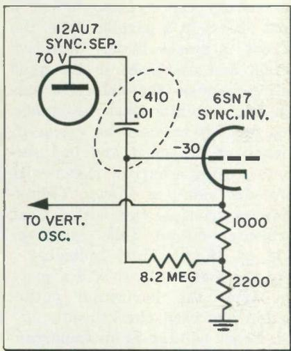
Fig. 1—Intermittent loss of horizontal sync and weak video in an Admiral 21F1 TV set was caused by a leaky sync capacitor.
