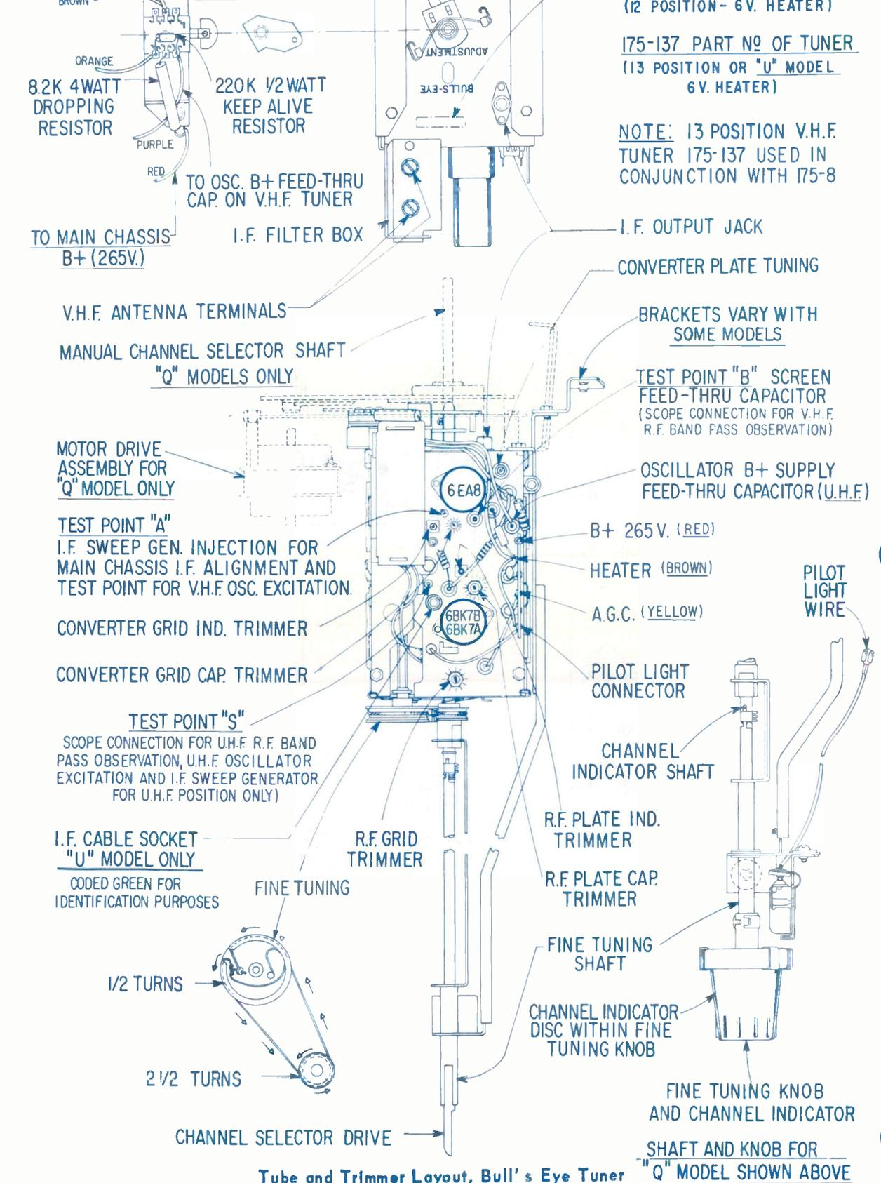
**Tube and Trimmer Layout, Bull's Eye Tuner "Q" MODEL SHOWN ABOVE**
