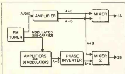
vised whereby stations could broadcast both stereo signals on the same carrier. One of the stereo signals modulated the carrier directly, the other signal was used to modulate a subcarrier which then modulated the main carrier. The general term multiplex is used to describe any communications system where more than one signal is transmitted on the same carrier. Accordingly, stereo broadcasting is often called a stereo multiplex system.
