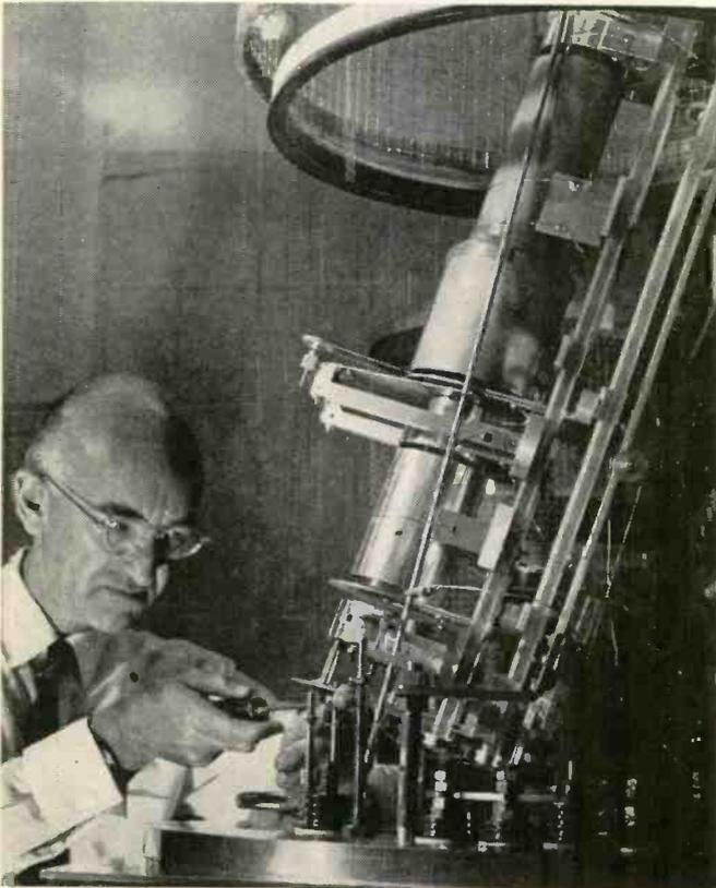
This giant cathode ray gun, similar to those found in TV picture tubes, is a tool for studying electron beams. Developed by Westinghouse advisory engineer Dr. Hilary Moss, the gun is used to learn how closely beams can be focused to give images of the greatest density.
