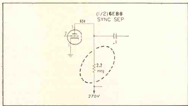
A critical vertical hold control condition in excessive noise areas on some Magnavox series 34 TV chassis, can be corrected by reducing the value of a plate resistor in the sync separator ( $\frac{1}{2}$  6EB8 tube) from 2.2 megs to 1.8 megs.
