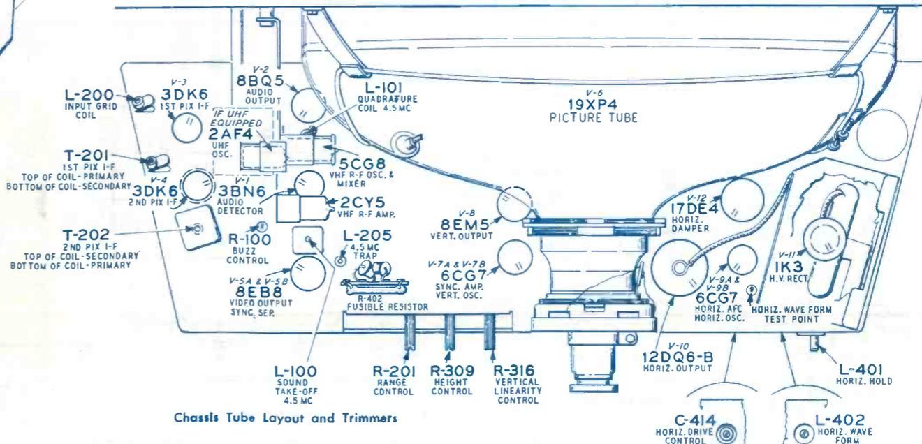
Chassis Tube Layout and Trimmers
