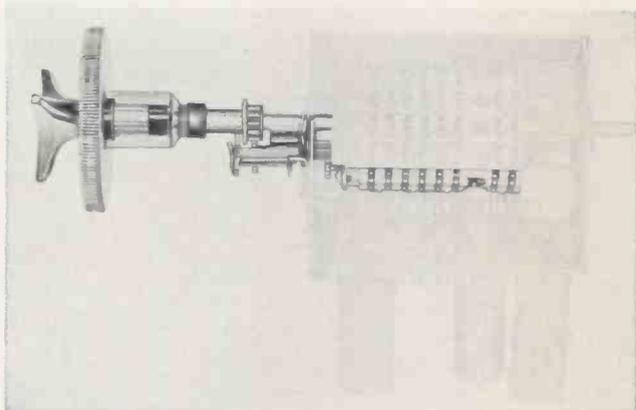
Zenith's turret tuner uses the front panel selector knob to adjust each channel's oscillator slug. The "fine tuner" engages each slug through a shaft gear arrangement when rotated.
