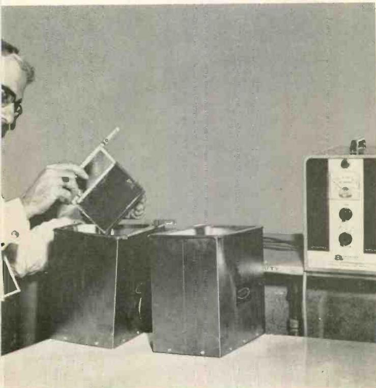
Saphier pushes button in dark room and electronic "computer" controls exposure when making photographic enlargements.
