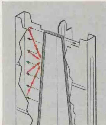
In ordinary rectifier tubes, filaments burn out when they overheat from a rise in reverse current. CBS eliminates this "back emission" in the 5U4GB with larger plates of non-emissive material that permit cooler operation and longer tube life.
