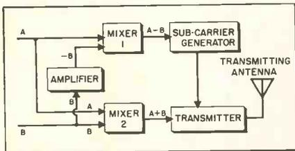
Fig. 1—Block diagram of the mixing circuits employed at a stereo multiplexing broadcasting station, showing the  $A + B$  and  $A - B$  type Crosby FM-FM transmission system.
