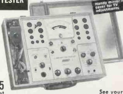
AS A TUBE TESTER... will check emission, inter-element leakage and gas content of all tubes.
