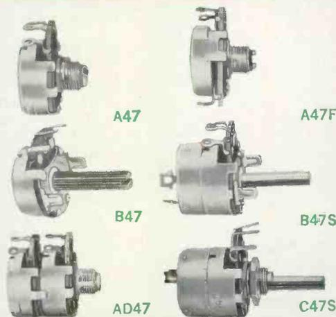
The ABC's of Servicing! Series 47 carbon controls are ½ watt units available in all popular values and tapers for volume control, tone control, and other radio and television functions.
