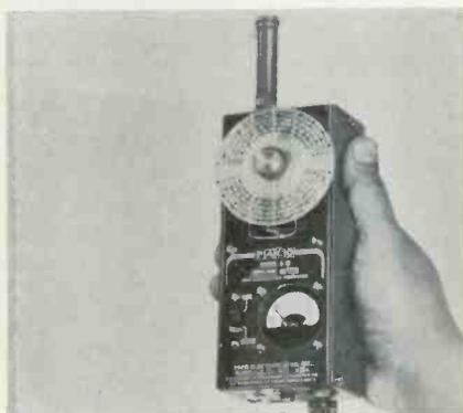
tions such as determining "Q" of L/C circuits and for "cold" alignment of filters and traps. Equipped with large, easy-to-read thumb-actuated dial. Kit, complete with set of 8 plug-in coils and assembly manual, \$31.95. Wired, \$49.94. Paco Electronics Co., 70-31 84th St., Glendale 27, L. I., N. Y.
