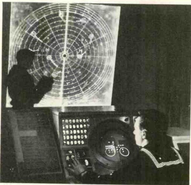
The old, slow grease-pencil method of plotting aircraft at top contrasts with new Hughes display console in foreground. Navy radarman examines positions of airborne, surface and submarine targets on detector-tracker.
