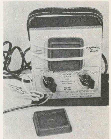
Fig. 2—Test instrument's meter face is protected by a rubber caster held in place by rubber bands.
