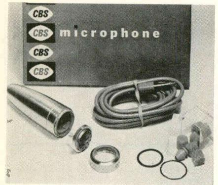
meet particular requirements. The microphone is designed around a special ceramic element which develops unusually high output and is unaffected by heat or moisture. Sensitivity, 1000 cps 52 db below 1v/microbar. Recommended load, 5 megohms. Frequency response, 30-10,000 cps. CBS Electronics, Danvers, Mass.
