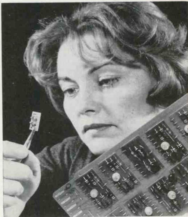
Four of the RCA midget tunnel diode wafers at left will perform the same computer switching job as the large circuit board shown—but 1000 times faster. The device permits electronic switching at speeds approaching 186,300 mph, the speed of light.
