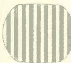
**Color-Bar Pattern...** Ten bars of color including R-Y, B-Y, G-Y, I and Q signals spaced at 30° phase intervals for checking phase and matrixing, and for automatic-frequency and phase alignment.
