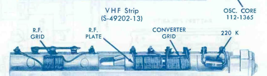
\*USE ONLY ZENITH REPLACEMENT TYPE LEAD LENGTH IS IMPORTANT FOR PROPER INDUCTANCE
