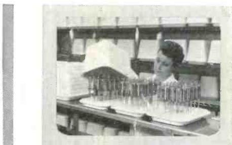
Finished guns after ultrasonic cleaning in a super wetting agent are carried to the assembly line in these covered plastic cases—further protection against contamination.
