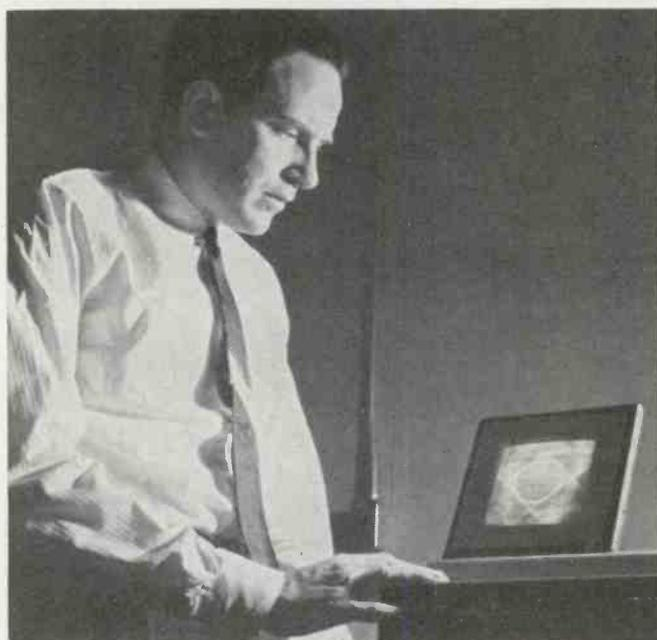
Electronic Panel less than one-half inch thick, invented by Stephen Yando of GT&E Labs., utilizes a new principle to produce a moving, lighted image. In the device shown above, composed of a piezo-electric ceramic material, a coating of electroluminescent material is actuated by a moving electric charge to produce a luminous display.
