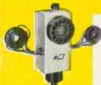
**Model C40 Adapter.** For use only with all previous B&K Model 400 and 350 CRT's. Tests and rejuvenates TV color picture tubes and 6.3 volt 110° picture tubes. Net, \$9.95
