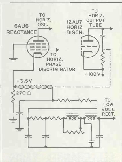
Fig. 1—Wiring error caused feedback of sine wave voltage to control tube's cathode. A-c voltage resulted in poor horizontal hold range.
