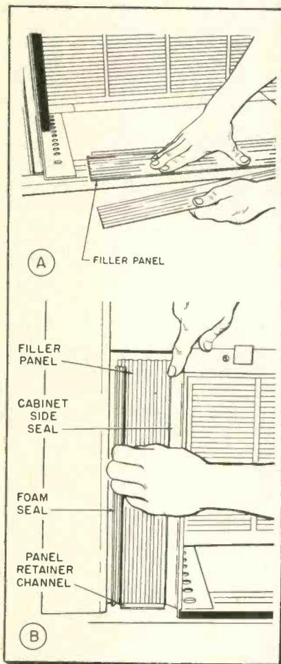
Fig. 6 (A)—Filler panel is broken on scored edge against a flat surface. (B)—Cut panel edge is inserted into the rubber side seal groove by flexing the beaded lip of the rubber seal.
