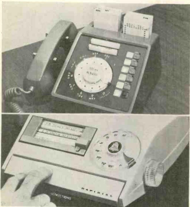
Push-button telephones dial numbers automatically with punched cards or magnetic tape. (Top) Bell Telephone Systems' card dialer. (Bottom) "Rapidial" has numbers pre-recorded on magnetic tape. Up to 290 names and numbers can be handled. Knob is set to name, receiver lifted and dialing bar pressed. Phones are expected to benefit sales and reservation personnel, brokers, buyers, or any others who make frequent same-number calls.
