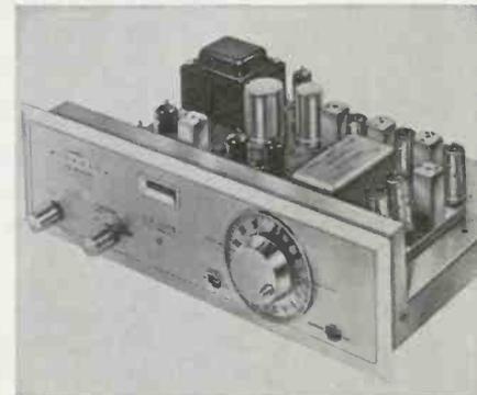
detector give the new model a remarkable usable sensitivity of 2.5 μv, measured by stringent IHFM standards. It has 10 tubes and 11 diodes. Can receive either monophonic FM or stereo FM multiplex programs. Special circuitry for stereo tape recording is included. \$199.95, east of the Rockies. H. H. Scott, Inc., 111 Powdermill Rd., Maynard, Mass.
