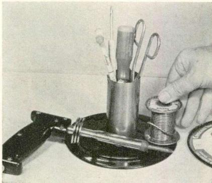
Fig. 1—Handy tool holder is made from discarded wire spool by removing one end.
