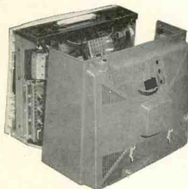
**OFF** The back *and the sides* of the cabinet come off as one unit, exposing the chassis for maximum accessibility.
