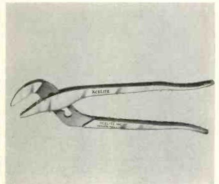
erful leverage in each of 4 gripping positions. Simple, lever-action movement of the handle adjusts serrated jaws. Mirror finish plate is rust resisting. Measuring only ⅝" at its thickest point, 7" model adjusts to 1⅛" opening. Large 10" model, ½" thick, max. jaw opening, 1½". Xcelite, Inc., Thorne Ave. & Bank St., Orchard Park, N. Y.
