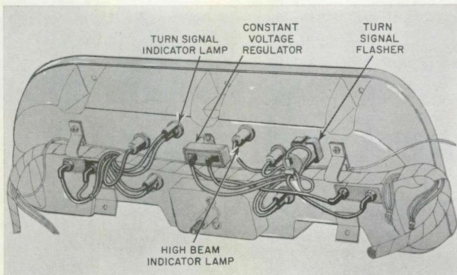
Fig. 1—Constant voltage regulator, mounted on 1960 Mercury cars, can interfere with radio reception due to poor electrical contact or lack of a filter choke.
