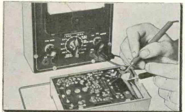
Transistor radio current drain can be measured by inserting a piece of paper between ground contacts of a radio's battery. Place test leads across paper, as shown.
