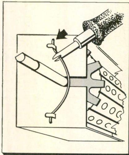
Fig. 3—Slightly spread forked soldering aid holds on to "jumpy" turret tuner retaining springs.
