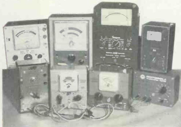
Fig. 4—The ET Editorial Staff used 52 low-medium-high power transistors and two transistor radios to evaluate testers' operation.
