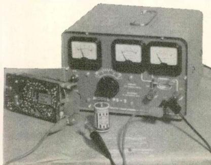
Fig. 5—An Electro Products Labs. Model PS-2 power supply was used to substitute for a transistor radio's battery. The supply provided us with low-current (0-75 ma) and variable voltage. It can also provide high current for 6 or 12 volt auto radios.
