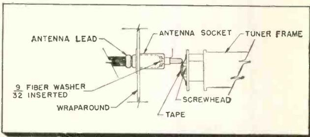
A fiber washer inserted at the antenna socket, or friction tape placed over screw heads, can prevent a dead or noisy Cadillac auto radio.
