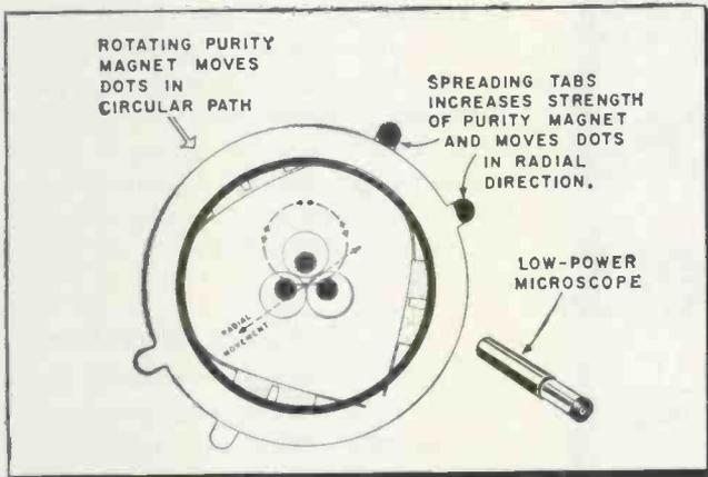
Purity adjustments at center of CRT are made by adjusting purity magnet tabs. A low power microscope is used to check beam's centering on its proper color phosphor dot.
