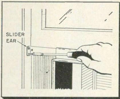
Fig. 7—Two screws attach slider ears to window stop moulding on right and left sides of the conditioner.
