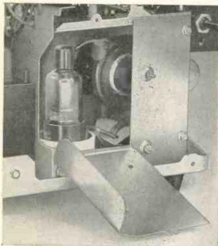
**DOWN** The high-voltage cage trap-door drops down for easy rectifier tube replacement. The whole panel is removable.
