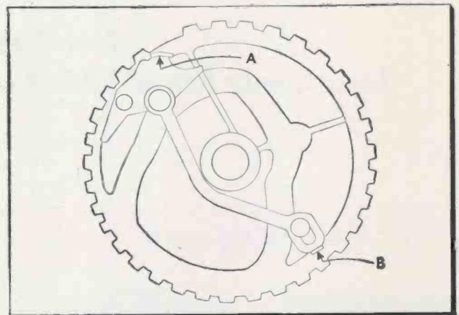
Proper record cycling is obtained by adjusting tabs A & B after repairing cam gear in a Webcor diskchanger.
