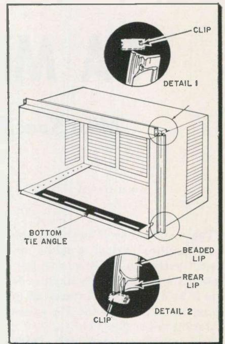
Fig. 4—Details of rubber side seal installation. Beaded lip of seal must be toward the cabinet front.
