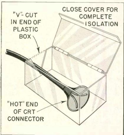
iced without a CRT attached. This creates a psychological hazard—keeping an eye on the HV lead. The high voltage anode lead can be easily isolated with a modified plastic box.
