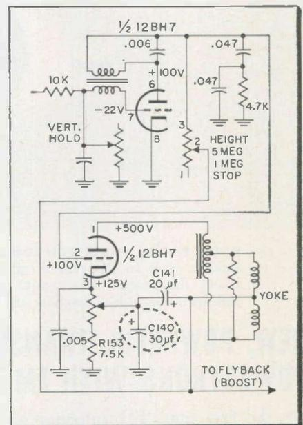
Fig. 2—Open  $30\mu\text{f}$  vertical decoupling capacitor "killed" vertical sweep in a Crosley 404 TV chassis.
