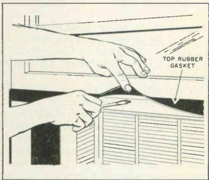
Fig. 8—A permanent installation requires a screw to be driven through the top-bar center hole into the window sash.
