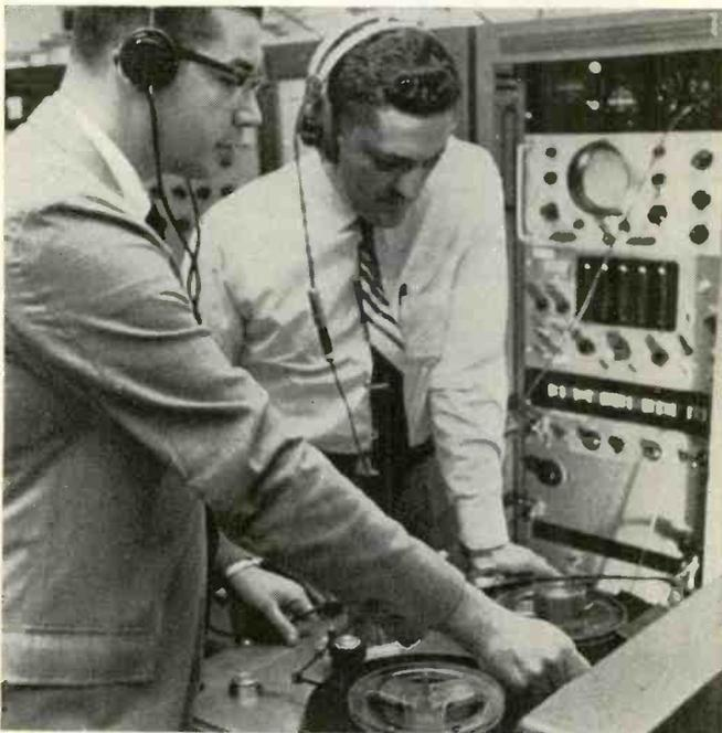
Bell Labs engineers Gerstman and Kelly listen to tape recording of speech synthesized by a digital computer. Punched cards coded for speech sounds are processed to actuate nine control signals corresponding to voice pitch, intensity, frequencies and timing. The machine will also sing (but Doris Day does a better job). Project purpose is to improve communication techniques.
