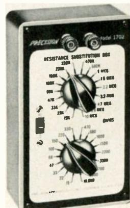
Model 1720 resistance substitution box permits direct substitution of 36 different resistance values through the use of either of two clearly marked rotary switches. Standard EIA resistance values in this unit range from 15 ohms to 10 megohms. Wattage dissipation of all resistors, 1 watt  $\pm 10\%$  tolerance. Dimensions  $6\frac{1}{2}$ " x  $3\frac{3}{4}$ " x  $2\frac{3}{4}$ ". Shipping weight, 2 lbs. Price, \$15.95. Precision Apparatus Co., 70-31 84th St., Glendale 27, L. I., N. Y.
