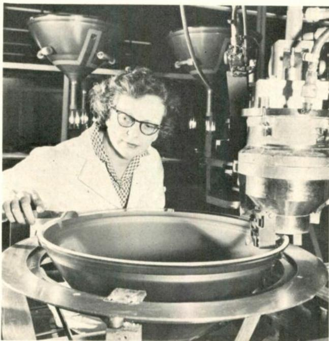
Solder application machine helps accelerate production of color CRT's at RCA's \$10 million Lancaster, Pa. plant, where \$1.5 million expansion program is underway to meet anticipated 250% increase in 1962 demand. The machine spreads a thin ribbon of special glass-sealing solder to the edge of a 21-inch type CRT envelope while it is rotating.
