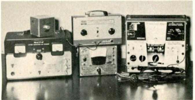
Test instruments shown, left-to-right, are: Seco Model 510 Attenu-load, Precision Model P-28 Battery Eliminator and Charger, GC Model 36-524 Component Selector, Seco Model 510 CB Transmitter Tester, and Sencore Model SS-117 Sweep Circuit Analyzer.
