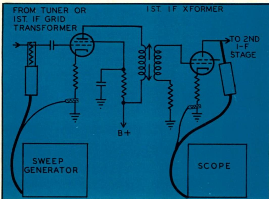
Fig. 3—A sweep generator and scope can be used to locate defective i-f transformers.
