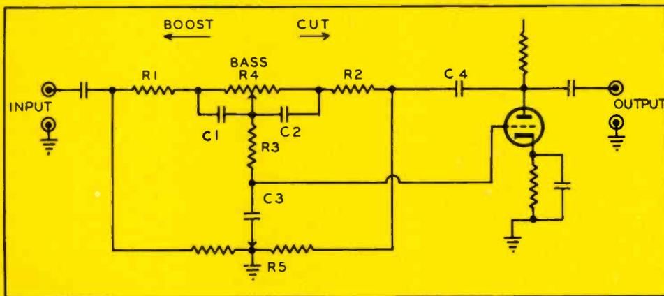
Fig. 6—Basic circuit of Baxendall feedback type tone control network.
