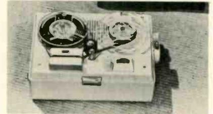
imum recording time of 68 minutes. Has "fast forward" speed-up device, single dial "one-control system" and level meter. Operates on four flashlight cell batteries. Printed circuit eliminates wiring breakdowns. Output, 500 mW. Takes 3" recording tape. 2 1/2" PM speaker. Complete with accessories, including dynamic microphone, monitor earphone, reel, tape, extension cord, leather carrying case. \$199.95. Sampson Co., 2244 S. Western Ave., Chicago 8, Ill.
