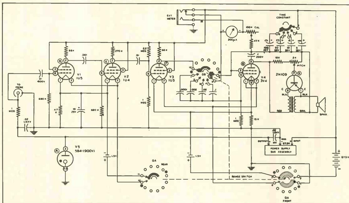
Fig. 4—Diagram of amplifier, range and indicating section of Heath Model RC-1 portable radiation counter.
