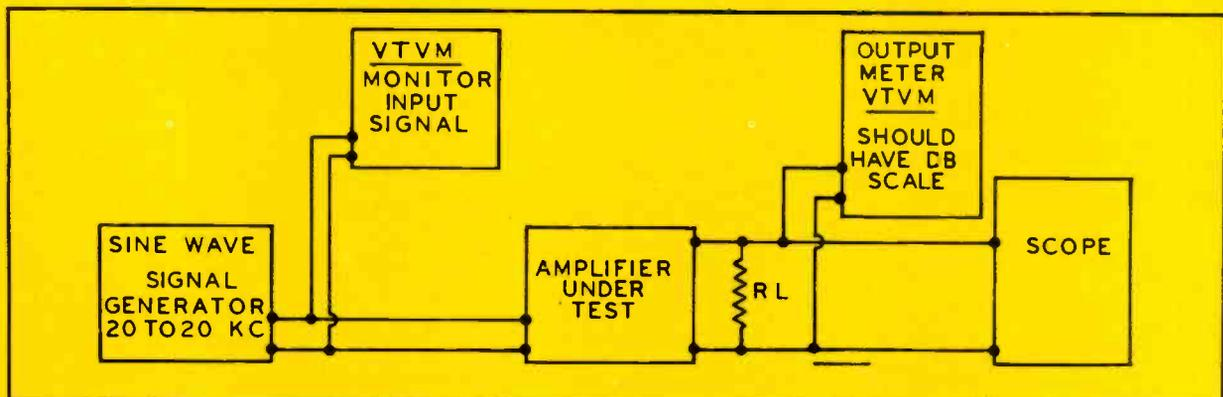
Fig. 2—Test set-up required for checking tone controls. RL is not used when the output is from a preamplifier.
