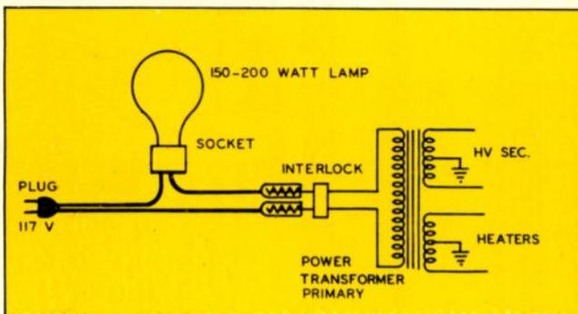
Fig. 2—If a load-check meter is not available, an ordinary lamp can be used to isolate a defective power transformer.
