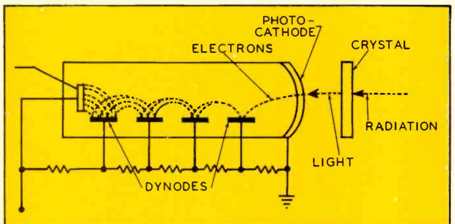
Fig. 5—Phosphor crystal converts radiation to light. Light sensitive photo-cathode converts light into electrons which are progressively increased by the photo-multiplier tube anodes.
