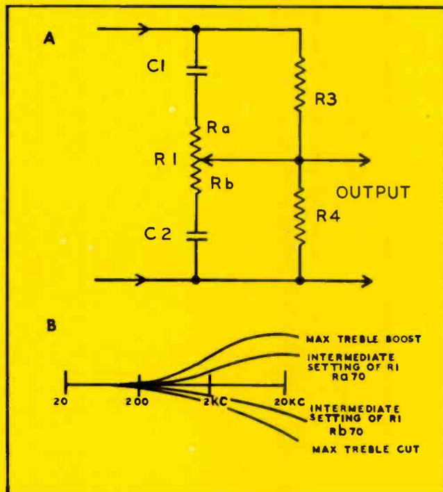
Fig. 5 (A)—Bass control network. (B)—Curves resulting from bass control action and curve for intermediate control setting affects center frequencies.
