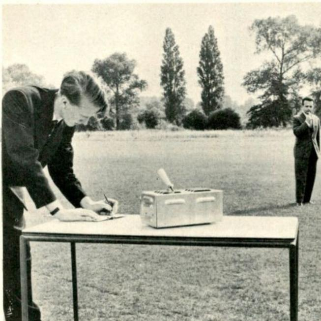
A "foghorn for the blind," has been developed by Standard Telephones and Cables Ltd., ITT British affiliate. Sound from a special, transistorized, high-frequency dog whistle, blown by the blind person, is selectively picked up by a microphone on the device and causes a self-contained bell to sound. The direction and intensity of the bell's sound enables the blind person to estimate his position in relation to the known location of the device. The range of the device is about 60 yards.
