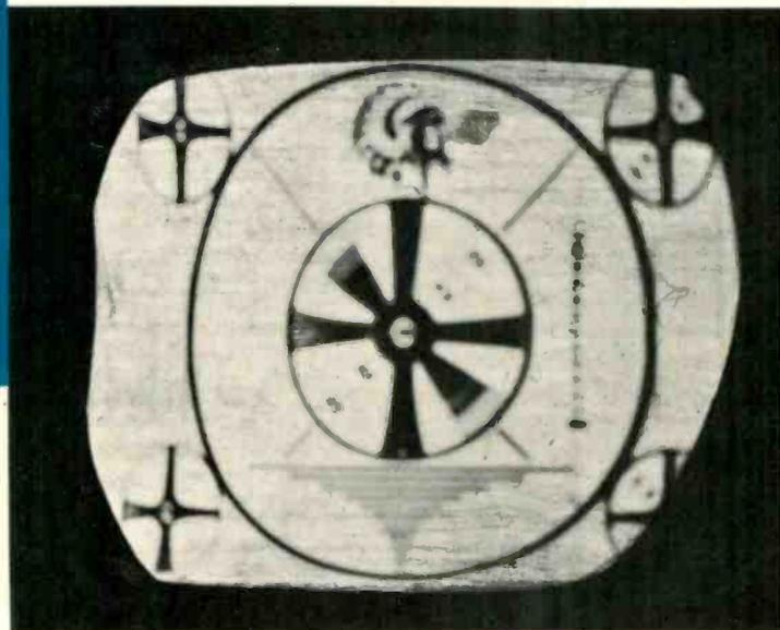
Fig. 1—Picture on TV screen after one leg of rectifier winding opened on transformer. Shrinkage and neck shadow were accompanied by a substantially darker picture.
