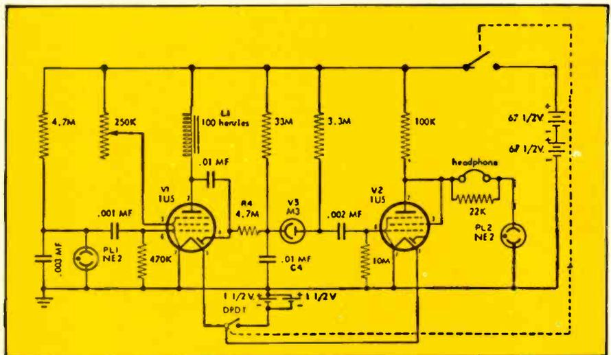
Fig. 3—Schematic of EICO's Model 803 portable radiation detector employs headphones and neon lamp for aural and visual radiation indications.
