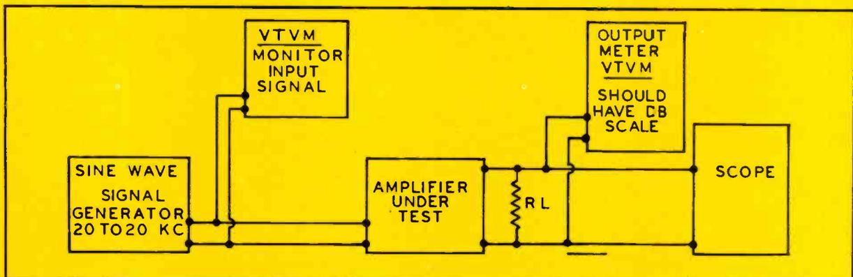
Fig. 2—Test set-up required for checking tone controls. RL is not used when the output is from a preamplifier.
