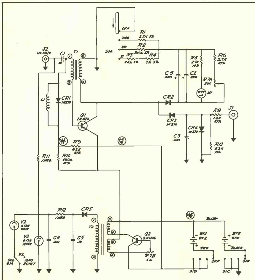
Fig. 7—Schematic diagram of the Model 489 Victoreen radiation counter which is designed to use either a Geiger-Mueller or a scintillation probe.
