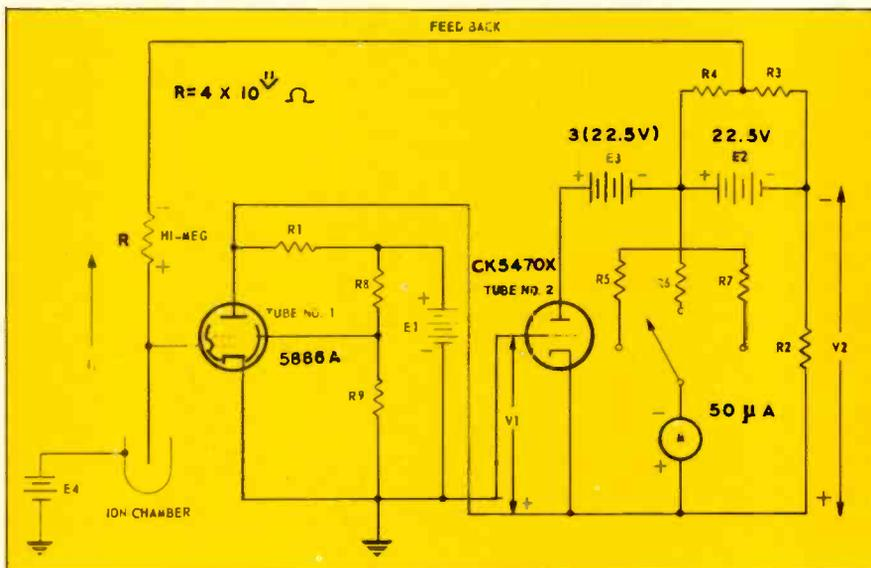
Fig. 2—Basic schematic of a portable radiation detector using a microammeter.
