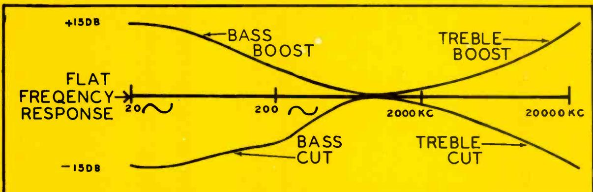
Fig. 1—Graphic illustration shows the five functions of a typical tone control.
