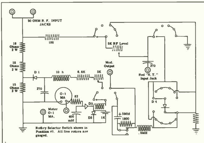
Schematic of Seco's Model 510 Citizens Band transmitter tester.
