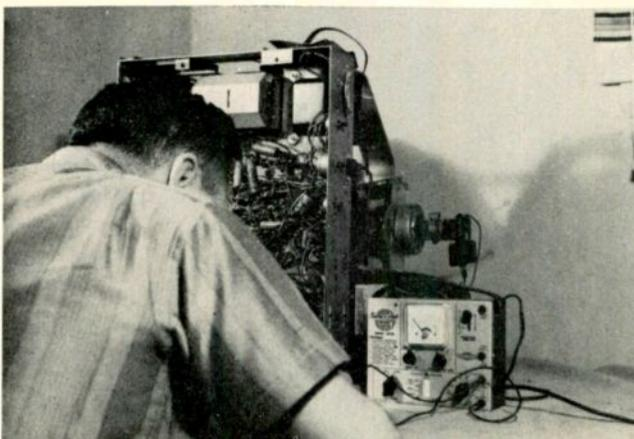
Fig. 4—Sweep-circuit tester is used to check a vertical output transformer by signal substitution.
