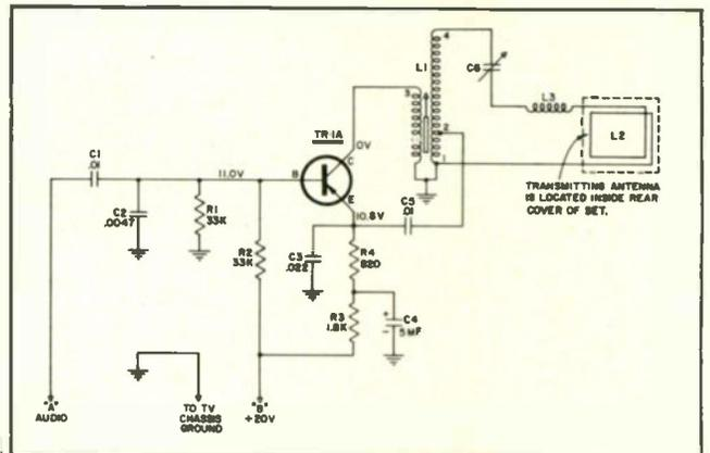
Circuit of Westinghouse transistorized "Mobile-Sound" transmitter is amplitude modulated by a TV set's audio signal. Unit "transmits" the TV set's sound to any nearby a-m broadcast receiver.
