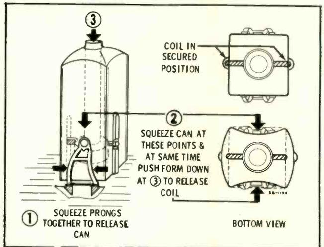
Coil shields in Motorola TS 581 series chassis can be removed for coil component replacement by following the steps outlined here.
