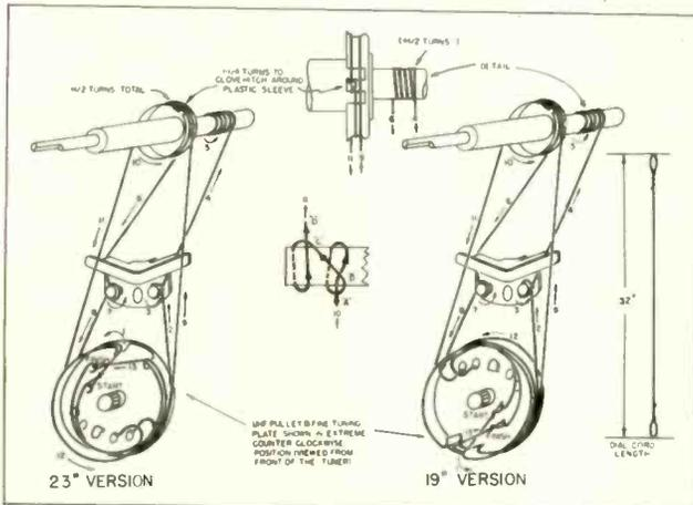
UHF tuning problems in General Electric "MW" TV chassis caused by dial cord slipping on fine tuning plate, can be cured by revisions.
