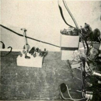
Novel tool holders made from Styro-foam material keep small tools handy.
