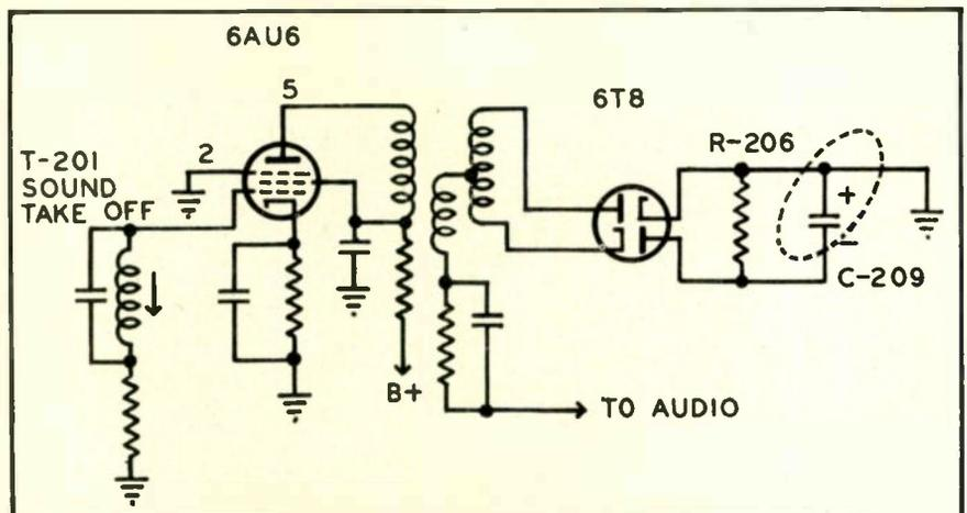
Intermittent static and varying sound was caused by defective capacitor C-209.
