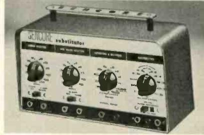
resistors, capacitors, electrolytics and rectifiers. Each section offers a complete range, can be used independently, and
