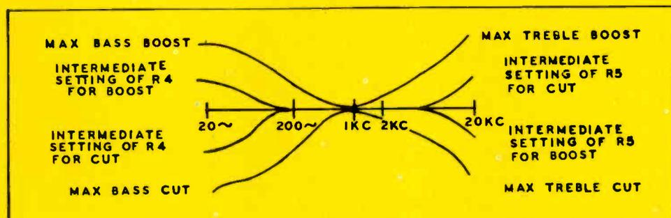
Fig. 7—Curves resulting from settings of Baxendall tone control network. Only tones at ends of band are affected.
