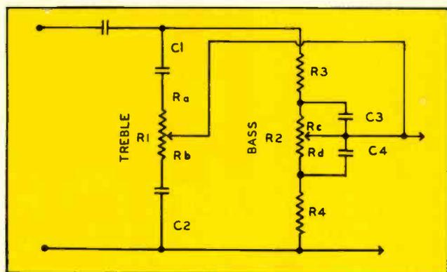
Fig. 3 — Functional diagram of "Losser" type tone control network.
