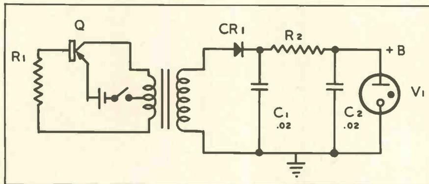
Fig. 6—Simple radiation detector power supply employs a transistor oscillator and a transformer to boost voltage.
