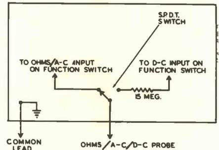
VTVM probe-lead modification employs a s.p.d.t. switch to simplify meter use.
