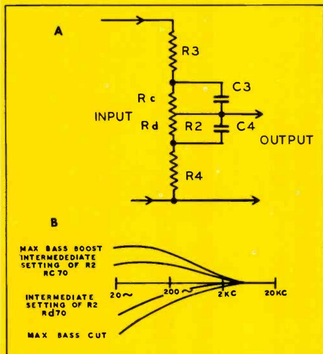
Fig. 4 (A)—Treble control network. (B)—Curves resulting from treble control action. Note that curve for intermediate setting affects center frequencies.
