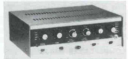
gold and contrasting brown, it has standard headphone jack on front panel to accommodate most stereo phones. Output is 30 w, 15 w per channel. Frequency response is ±0.5 db 30 to 25,000 cps, and harmonic distortion is less than 1%. Tube compliment is 2 — 12AX7, 4 — 6BM8 and 1 — 6CA4. Size is 12¾ in. wide x 4¾ in high x 10½ deep. Price is \$69.95. Olson Electronics.
