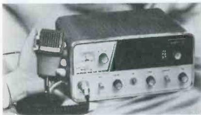
gulations. All 23 citizens band channels can be selected with a single control for both transmit and receive. Equipped with a dual power supply the Range Grain unit can be either as a mobile or base station. It weighs 13 lb and is 11 in. wide
