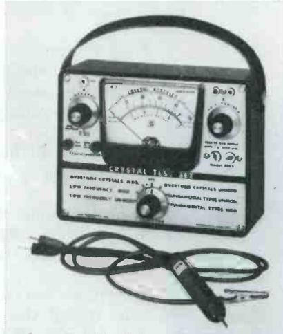
audio output across voice coil, and beat note in RF comparisons. It will generate a crystal controlled RF signal with 400 cps tone modulation and will serve as a 0.05 v audio frequency signal source. It retails for \$48.95 net. Seco Electronics Inc.
