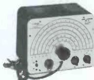
Lafayette's TE-20 is a general purpose signal generator operating on fundamentals and harmonics. \$27.95.
