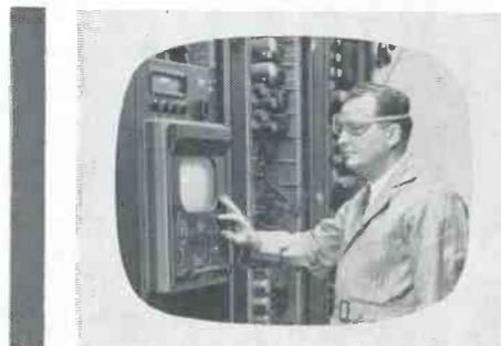
**Precision Signal Generator** sends out the test pattern shown on the screen above. Fidelity of reproduction of this virtually perfect signal (resolution: up to 2,000 lines!) is an accurate index of the picture tube's performance after life testing.
