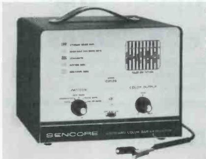
dialing any of the five patterns. Signal output is adequate to over-ride most local channels. Other low channels can be selected if desired by simple slug adjustment in rear. Stability is said to be insured by crystal controlled circuits, factory pre-aged vacuum tubes and standby position on the on-off switch. The CG126 weighs less than 10 lb. and measures only 11 x 8 x 6 in. providing portability for home or shop service. The CG126 color bar dot generator sells for \$99.50. Sencore.
