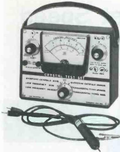
*SECO Crystalign Meter Model 500A at \$48.95* — The Model 500 is actually a two-way radio tester and combination crystal checker.
