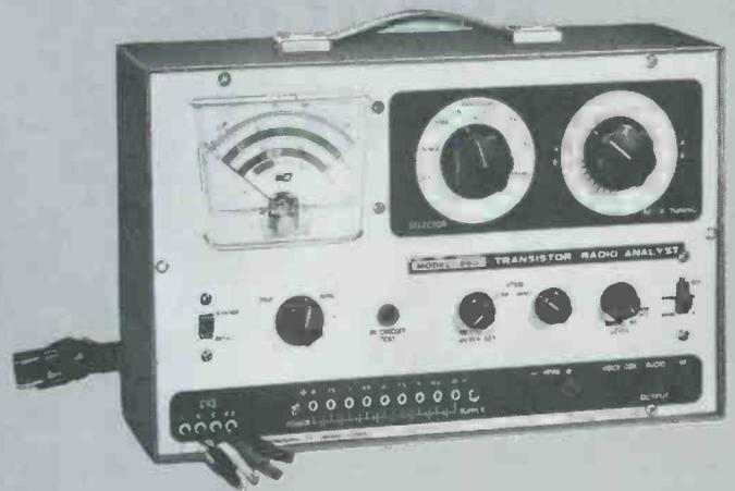
The transistor radio analyst by B & K is one of the special types designed for a specific repair area.
