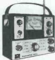
A precision instrument designed to assist the technician in installation and servicing of low power transceivers. Measures: RF power (absolute) 0-5 w.; 0-120% amplitude modulation; VSWR; Produces a 100mw carrier (with or without amplitude modulation of a 1000 cps tone) for checking receivers; Use as a field strength meter.
