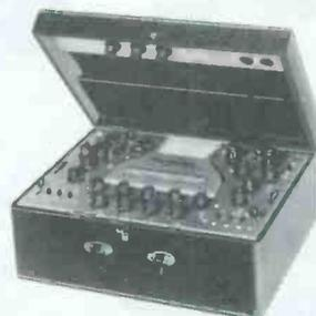
Heath's TT-1A mutual conductance tube tester is available only in kit form. Unit checks all common tubes, including thyratrons. \$149.95.
