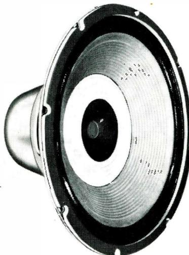
apex of the low-frequency cone. The design of the Model K-120 speaker places both surfaces in the same plane, reportedly minimizing phase and distortion problems, delivering exceptionally smooth response through the crossover point. The speaker has a rated frequency response of 30 cps to beyond audibility and a power-handling ability of 15 w of music. Rated output impedance is 8Ω. Minneapolis Speaker Co.
