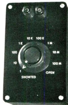
zeroing meters. The unit was designed for speedy checkout and calibration of ohmmeters or ohmmeter sections of multimeters in schools and industrial calibration labs. Accuracies available are: 1 percent, 0.1 percent and 0.05 percent. The 1-percent calibrators use carbon resistors, while the 0.1-percent and 0.05-percent units are made with wirewound resistors. The unit measures 3¾ x 6¼ x 3 in. Panco Products.
