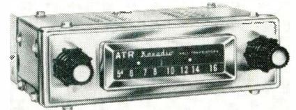
control, superheterodyne circuit, automatic volume control, three-section tuner and hand wiring (no printed circuitry). The unit utilizes seven semiconductors, which include five transistors and two diodes. The radio has a built-in speaker and an external speaker jack. The unit measures 5½ x 6½ x 2 in. and weighs 4 lb, reportedly permitting under-dash mounting with standard trim plate kits. \$29.95. ATR Electronics, Inc.
