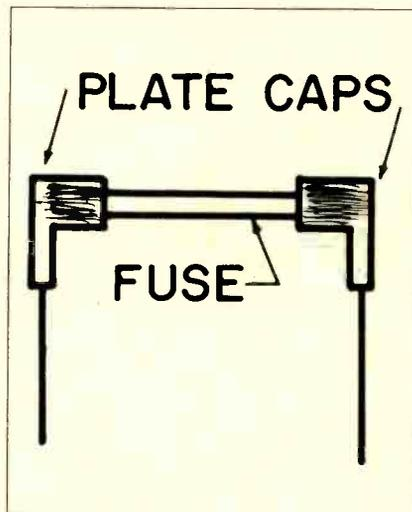
Salvaged tube grid-caps used to mount fuses above chassis.
