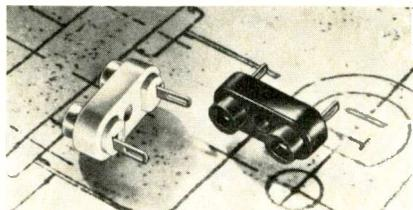
been introduced. The socket, No. 9748-16, is dimensionally identical to the TS0205C01 ceramic socket and accepts standard HC6/U crystals. It is suited for use where mechanical shock and vibration are problems, and is excellent for many commercial applications such as citizens' band transceivers, it is said. Dimensions are: length, 0.859 x 0.312 x 0.375 in. Contacts are spaced on 0.486 in. centers. A 0.125 in. hole is provided for mounting with a single screw. Eby.
