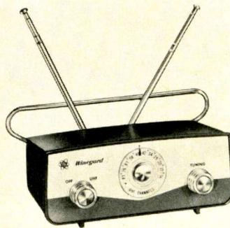
Models are also available without built-in antennas. All models are furniture styled in polystyrene cases in autumn brown trimmed with brushed gold and feature 3 gang capacitive tuning elements, 6DZ4 oscillator tube, isolated power supply with silicon rectifier, 1N82A diode and completely enclosed cabinets. Specifications indicate all models exceed FCC radiation requirements. Six models are priced from \$29.95 to \$69.95. Winegard.
