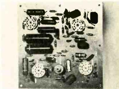
Sound-sync circuit board before installation on the chassis.
