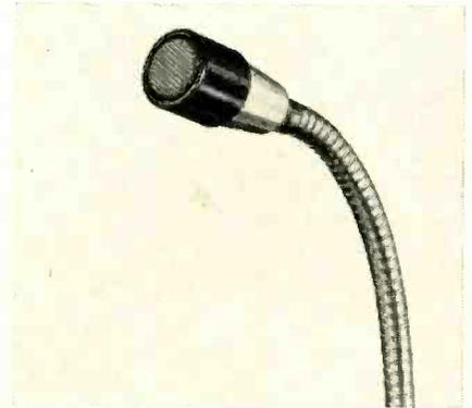
the use of unusually long cables without affecting response or level, it is said. Specifications gave frequency response as 40 to 10,000 cps with rising characteristic to 4500 cps; output level, -56.0 db (0 db = 1 mw per 10 microbars); net weight: 5 oz. Price, \$32.50. Shure.
