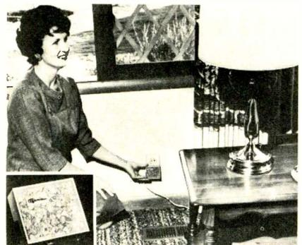
wall outlet and when lamps are plugged in, provides the home with automatic lighting. Lights are automatically switched on at night and off in the daytime, according to the maker. It can also provide automatic lighting for store windows, office, etc. Ramic.
