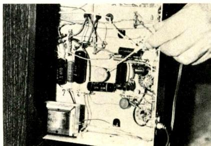
Insufficient width can be corrected by installing a capacitor across horizontal yoke above or below chassis.
