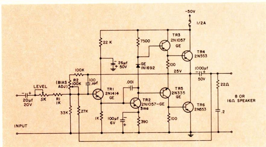
Fig. 1—Diagram of a transistorized audio amplifier.
