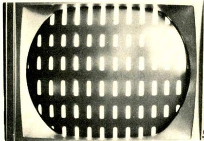
"Dot" pattern using the internal generator. Brightness and contrast control dot size which are shown at maximum.
