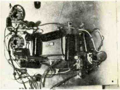
Horizontal and high voltage section comes assembled with a bundle of loose-ended wires.
