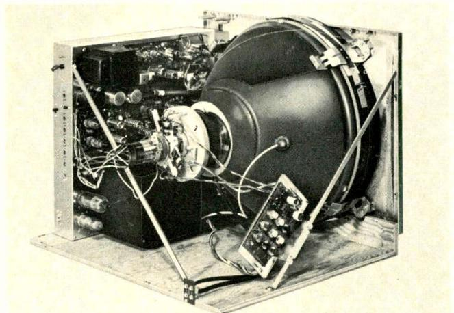
Rack mounted '63 model. Convergence controls are permanently mounted on brace as shown. The '64 models all employ the wall mount within the cabinet.
