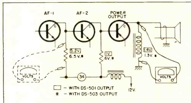
Delco auto radio transistor checks for dead radio.
