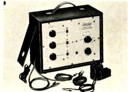
crosshatch pattern and the smallest dots available in anything but laboratory equipment, the maker said. A gated color-burst provides correct color alignment signals as well. Specifications indicated that the generator provides complete convergence signals — vertical bars, horizontal bars, crosshatch and dots — less than two lines wide and one line thick; a gun-killer for convergence and to facilitate purity adjustments; and a single-bar, crystal-controlled color-burst signal. Hickok.
