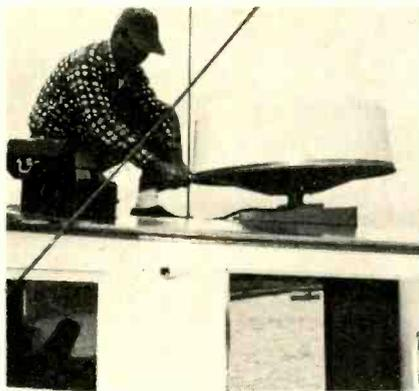
Technician installs radome on Raytheon radar antenna atop small cruiser.
