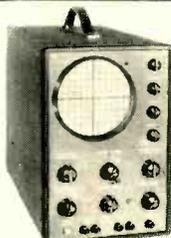
**EICO 427 ADVANCED GENERAL PURPOSE 5" SCOPE** High sensitivity scope has all the facilities and quality demanded for servicing audio, communications and industrial equipment. Vert. amp. flat from DC to 500 kc, -6 db at 1 mc; 3.5 mv rms/cm sensitivity. Horiz. amp. flat from 2 cps to 450 kc; 0.18 v rms/cm sensitivity. Automatic sync. Sweeps from 10 cps to 100 kc. Kit \$69.95; Wired \$109.95.
