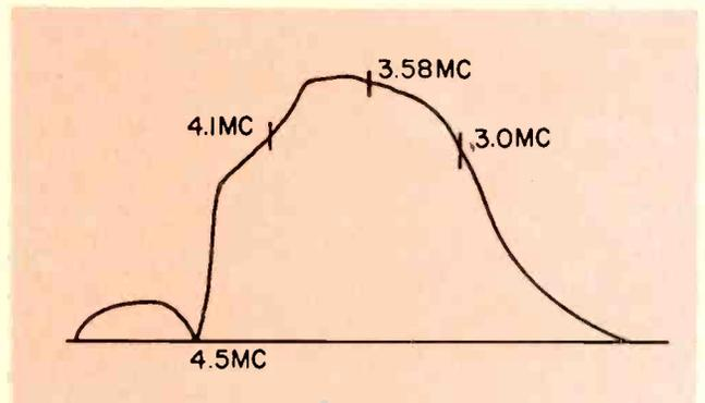
Fig. 3—Appearance of average color amplifier response curve.
