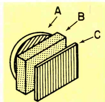
Fig. 1—Filter system shows rotating polaroid (A), dispersion filter (B) and the stationary polaroid filter (C).
