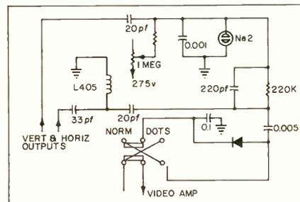
Circuit used in the built in dot generator is a simple neon oscillator triggered from horizontal and vertical pulses.
