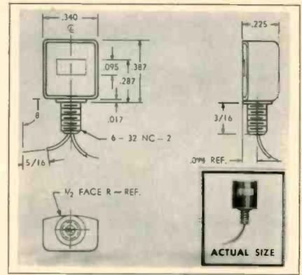
3K17, the head is especially designed for micro-miniature tape recording uses. The head is approx-
