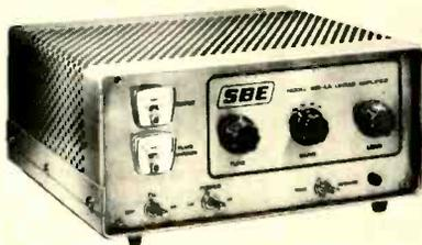
duced. The SB1-LA covers four bands: 80, 40, 20 and 15 meters. It was developed primarily for use with SB-33 transceiver but can be used with any single sideband unit. Its small size (11¾ x 5½ in.) makes it particularly appropriate for mobile use. The unit requires no input tuning. The amplifier operates as a Class AB-1 system for low distortion. It will be offered through electronic parts and communications equipment distributors at a suggested price of \$279.50. Sideband Engineers.
