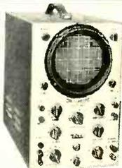
**EICO 460 WIDEBAND 5" SCOPE** For color & black-and-white TV servicing. Easily reproduces 3.58 mc color TV synchronizing burst. Vert. amp. flat from DC to 4.5 mc, usable to 10 mc; 25 mv rms/inch sensitivity. Horiz. amp. flat from 1 cps to 400 kc; 0.6 v rms/inch sensitivity. Automatic sync. Sweeps from below 10 cps to 100 kc. Kit \$89.95; Wired \$129.50.
