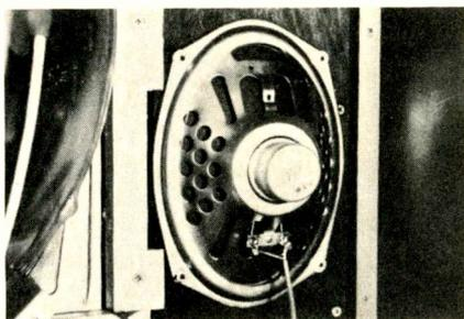
Special shielded speaker is used in cabinet model so convergence and purity are not upset by stray magnetic field.
