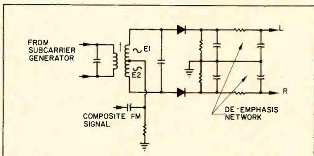
Fig. 3—Two-diode FM stereo demodulator schematic.
