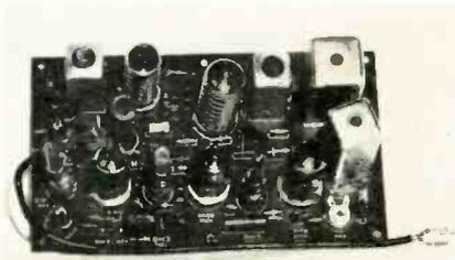
As is the tuner, the IF strip comes assembled and completely aligned. The tuner and IF are aligned together for optimum performance.
