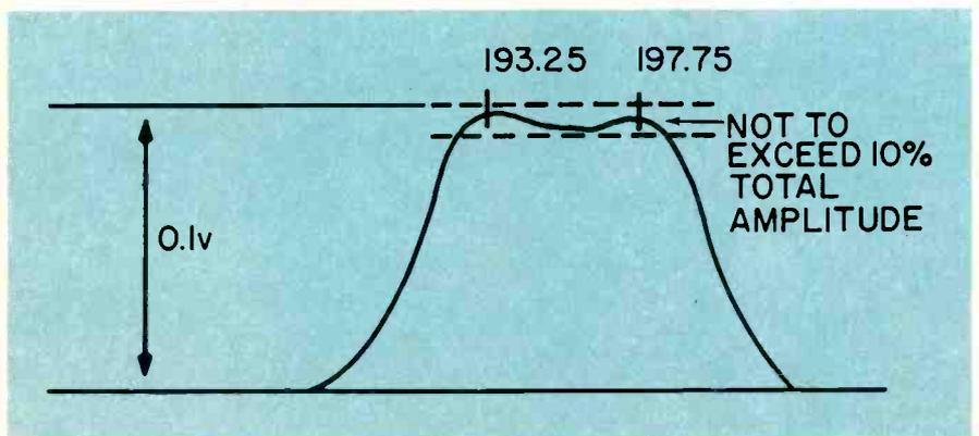
Fig. 1—Channel 10 RF response curve at the channel selector output.
