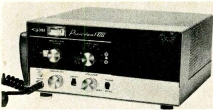
spot switch is included for exact frequency tuning. An illuminated "S" meter reads incoming signal plus relative output indications.
