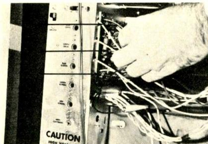
Two permanently installed clip leads are used to kill CRT guns. Three 100K resistors pointed out by arrows are test points.
