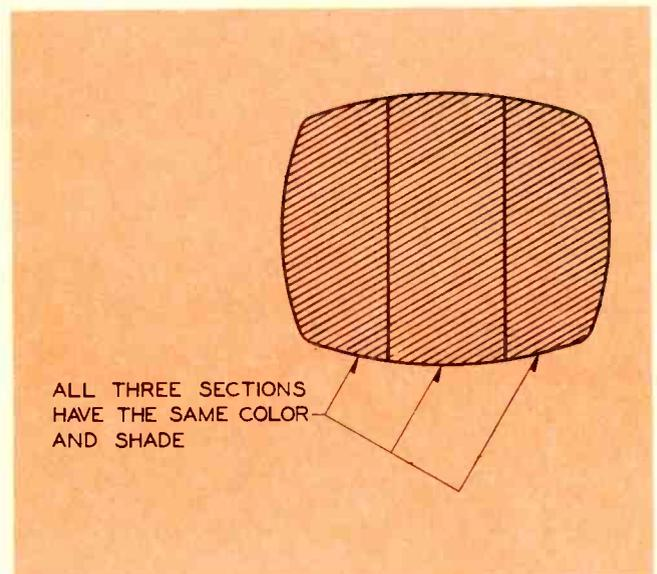
Fig. 2—Center area of screen will be the same brightness level as the two outside areas when the demodulator is adjusted properly.
