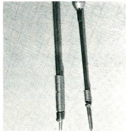
Solder is used as an aid to hold screws.
