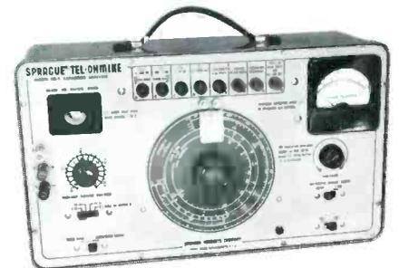
Sprague capacitor analyzer.
