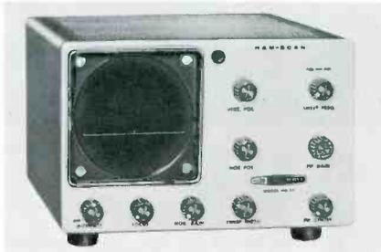
to be a useful accessory that will greatly increase the versatility and enjoyment of all amateur radio and CB operations. It is designed to operate with all receivers in service today and permits visual observation of band activity up to 50 kc above and below the frequency to which the receiver is tuned, the maker claims. Heath.
