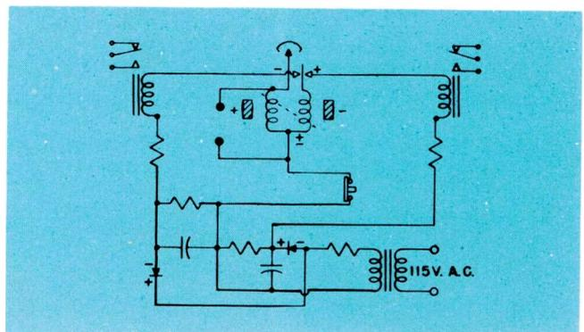
Fig. 3—A double contact circuit with manual reset.
