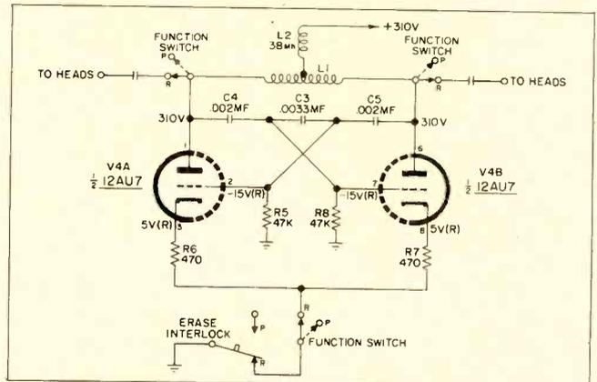
Westinghouse tape recorder bias-erase oscillator schematic showing erase-interlock and function switch.
