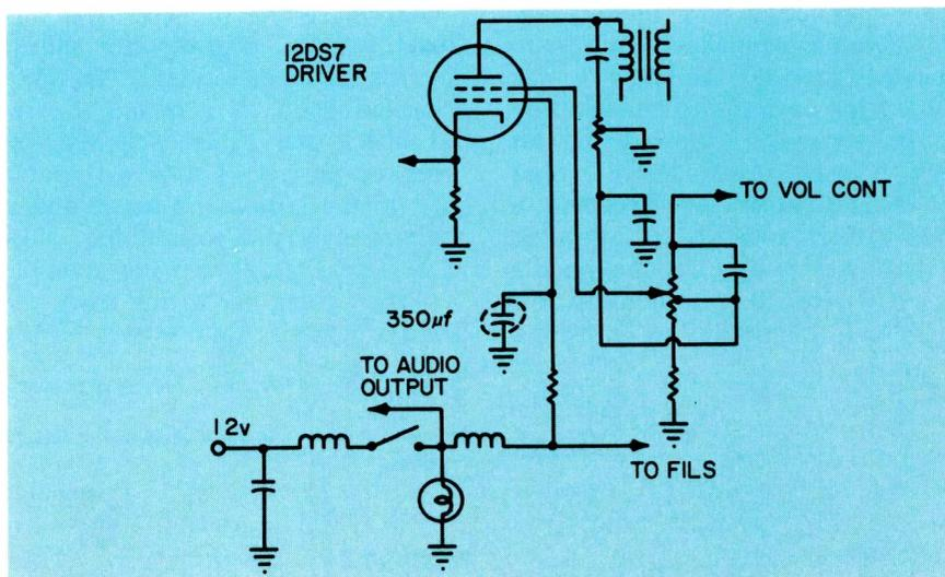
Fig. 2—A 350  $\mu\text{f}$  electrolytic, which checked good on a capacitor tester, caused a high pitched whistle all across the dial in a Buick auto radio.
