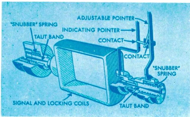
Fig. 1—Construction of a typical meter relay.
