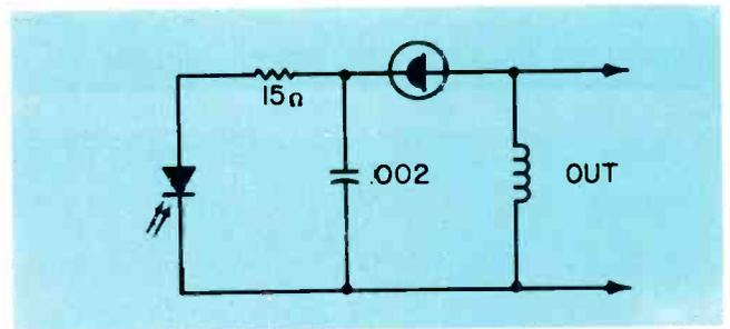
Fig. 3—Tunnel diode oscillator activated by photoelectric cell.
