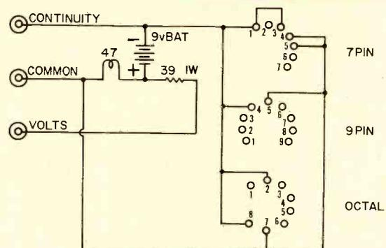
Fig. 2—Wiring schematic for special tester.
