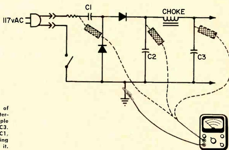
Fig. 1—The condition of filter capacitors is determined by measuring ripple voltage across C2 and C3. The ac line input filter, C1, is checked by determining the voltage drop across it.
