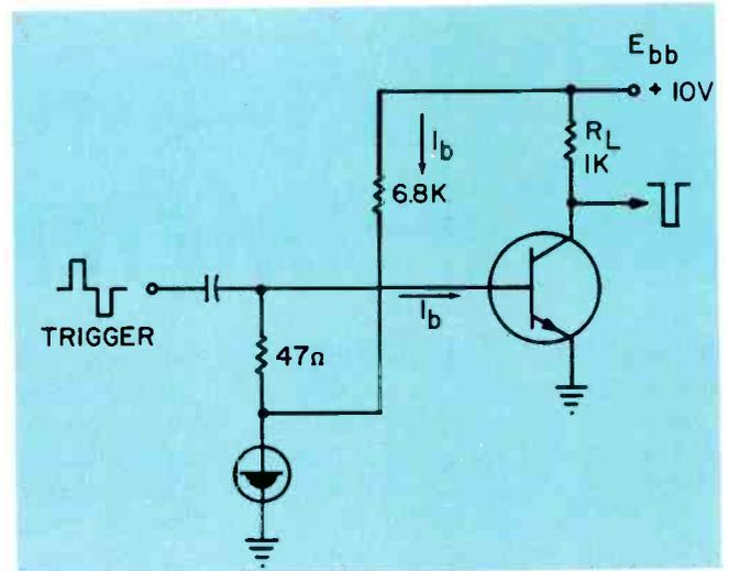
Fig. 2—Tunnel diode and NPN transistor in bistable circuit.
