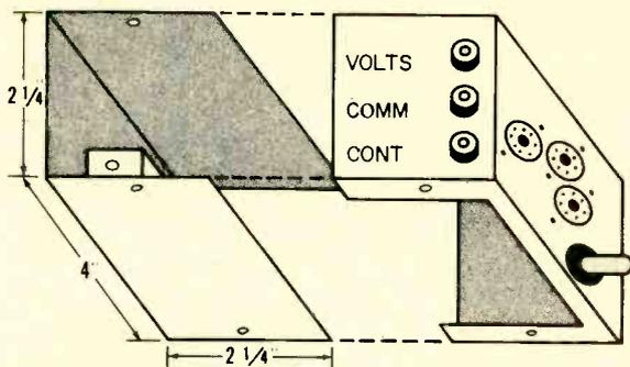
Fig. 1—Switch, sockets and pin jacks in special tester are mounted on 'Minibox.'
