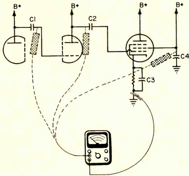
Fig. 2—Coupling and by-pass capacitors are checked with ac VTVM.
