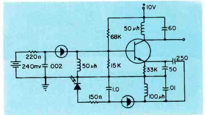
Fig. 4—Light operated modulator circuit is RF oscillator and audio oscillator.
