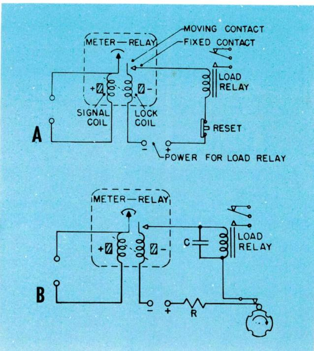
Fig. 2(A) — Basic meter relay circuit with manual reset.
