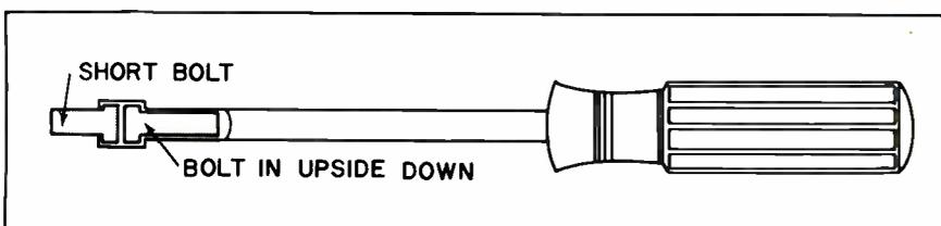
A screw inserted backwards in a nut driver makes it easier to start short screws in out-of-the-way places.
