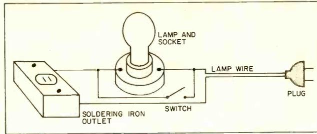
Fig. 1—A 'manual' thermostat can bring your straight bench iron up to working temperature within a few seconds by closing the switch shunting the lamp. Switch is left open when iron is not in use.
