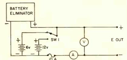
Fig. 5—Hookup for regular battery eliminator supply or trickle charger. The battery not in use is always on charge.
