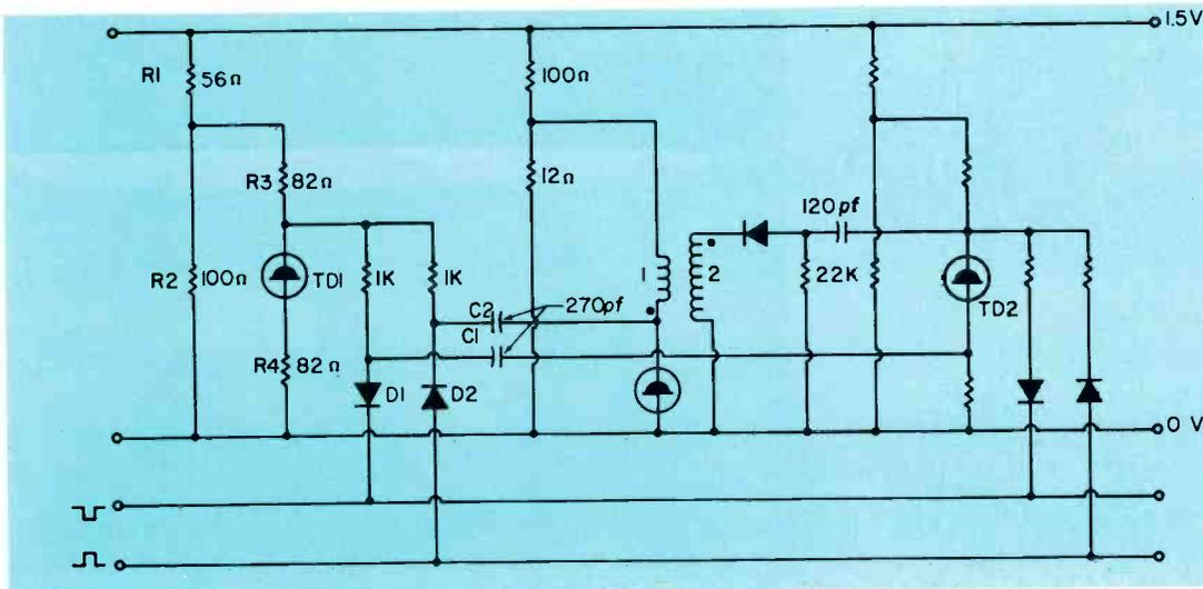
Fig. 5—Shift register circuit using tunnel diodes and backward diodes.
