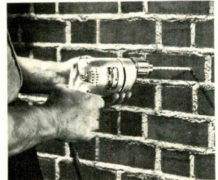
Carbide masonry and brick bits are handy for antenna installations and where it is necessary to mount fixtures or outlets on brick or cement surfaces.
