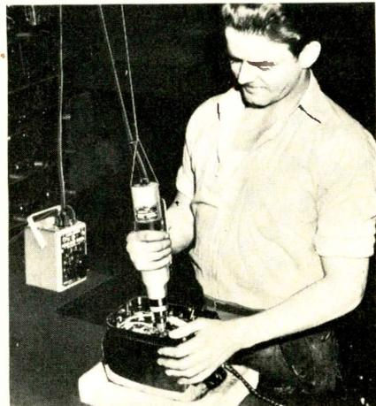
Power screwdriver mounted over bench speeds assembly and disassembly work in many TV-radio, Hi Fi shops.
