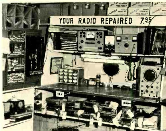
Fig. 3—Test and repair bench for auto radios is organized for maximum efficiency.
