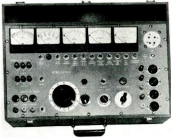
mits quick comparisons with tube chart, gives automatic indication of critical grid volts (trigger points), automatic indication of critical grid current on thyatron tubes and operational test of semiconductors. Accommodates all common industrial tubes from 0.1 through 16 amp, the maker said. Price \$1,285 net. Aleetric.
