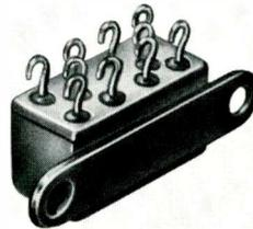
pulse to shift its bistable contacts, is announced. The contacts will maintain either of their two positions without consuming power, and will operate satisfactorily under severe environmental conditions, the announcement said. It has 2 Form C DPDT contacts rated at 2 amp, 28 vdc resistive load. Contact resistance is 0.05Ω maximum, or 0.100Ω after 100,000 operations, operating time is 3 ms at nominal voltage at +25°C, specifications indicated. Branson.
