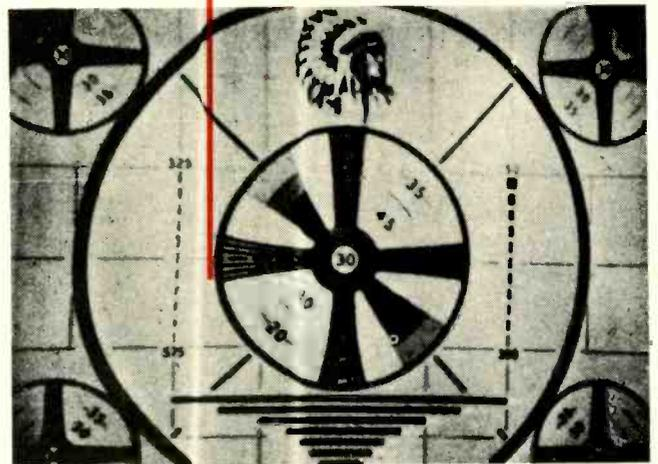
Flyback ringing may be confused with yoke ringing if careful attention is not paid to the intensity and kink in the yoke-caused line. Do not confuse the fold which may take place in the flyback line with the kink in yoke-caused trouble.
