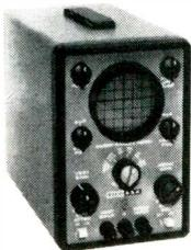
**EICO 430 PORTABLE GENERAL PURPOSE 3" SCOPE** Remarkably fine compact scope. Excellent for servicing audio, communications, and industrial equipment. Ideal as a ham shack monitor. Flat-face 3" CRT with mu metal shield eliminates affects of external fields. Vert. amp. flat from 2 cps to 500 kc, —6 db at 1 mc; 25 mv rms/cm sensitivity. Horiz. amp. from 2 cps to 350 kc, 0.25 v rms/cm sensitivity. Sweeps from 10 cps to 100 kc. Kit \$69.95; Wired \$99.95.
