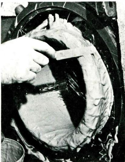
Open motors deliver performance similar to totally enclosed motors when the windings are encapsulated with RTV (room temperature vulcanizing) liquid silicone rubbers.
