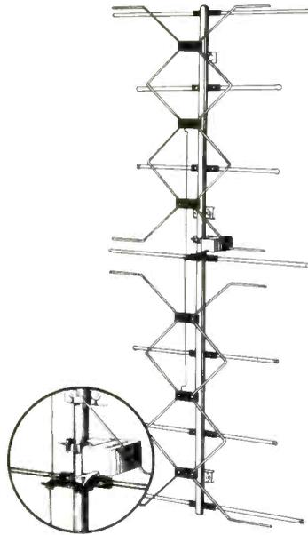
The announcement said that features include UHF preamplifier using two transistors, a single 300  $\Omega$  transmission line for 18 v power to booster and bring amplified UHF signal down to power supply at TV set and rust proof aluminum terminals. \$53.95 complete. Gavin.
