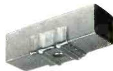
Boom reinforcing back up brackets at elements add triple strength to the riveted assembly, mounted on a rigid, non-crushable 1" heavy duty square boom. Boom rolled square from 1 1/4" diameter round aluminum for increased strength.
