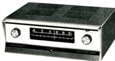
matic frequency ON-OFF switch, an ON-OFF-FM-stereo selector and a flywheel tuning control. The 7-tube circuit has a 12-tube function which includes built-in FM multiplex. Sensitivity  $2\frac{1}{2}$ ,  $\mu\text{v}$  for 20 db quieting, a monophonic frequency response of  $\pm 1$  db from 30 to 20,000 cps, stereo response  $\pm 2$  db from 50 to 15,000 cps; harmonic distortion 1 percent or less at 1 kc; channel separation 25 db or more at 1 kc, the specifications indicated. Price \$49.95. Heath.
