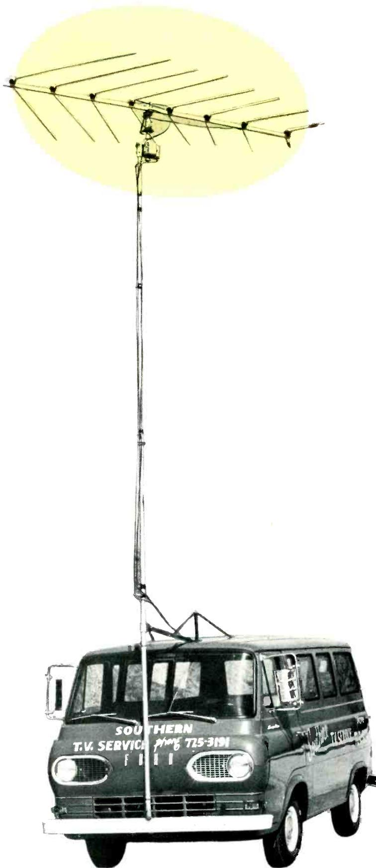
Motorized antenna elevated in receiving position on truck front
