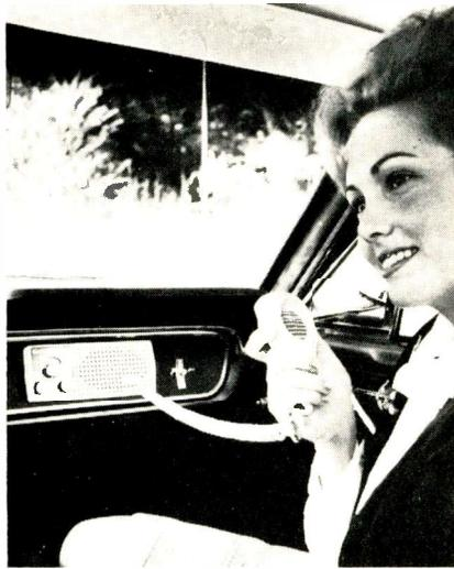
Transistorized CB set is only about half the size of comparable tube types.
