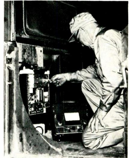
Field technician using portable test set to net receiver of a vehicle mounted radio.
