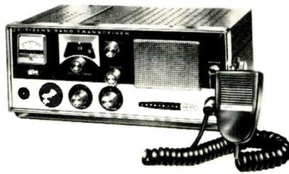
able with a receiver sensitivity of  $1 \mu\text{v}$ . 5-w input to transmitter with pi-network output to match 30-100
