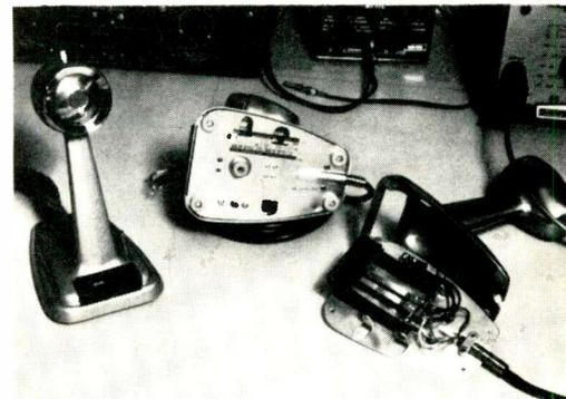
Fig. 7—The center rubber foot shown in base plate is a 'lift' switch.
