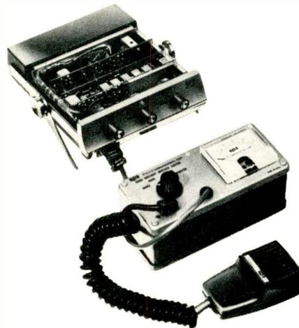
Fig. 5—Modular-constructed silicon transistor CB radio in troubleshooting position with service meter connected to set and microphone plugged into meter.
