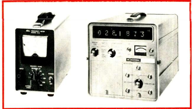
LEFT: Waters Model 343 frequency meter is transistorized and portable.
