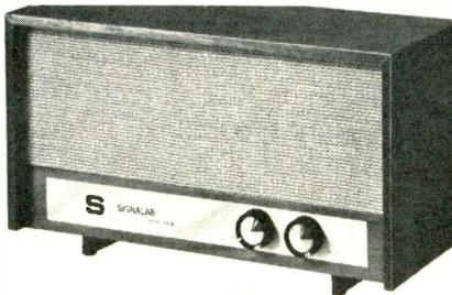
Squads, etc., receiving both mobiles and base. This receiver is available in any frequency from 25-50 Mc, or 150-170 Mc. The monitor receiver is housed in a walnut wood cabinet 15 x 6 x 8 in. Signalab.
