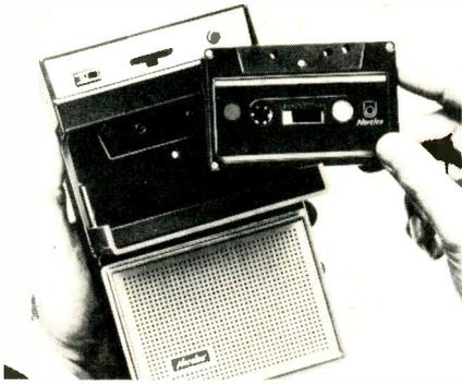
cluding one demo tape) and patch cord. The unit operates at 1 7/8 ips and can record from a radio, TV, phonograph, telephone, as well as its own microphone according to the maker. Transistor Complement includes: 1: AC126, 4: AC125, and 2: AC128. Size: 7-2/3 x 4 1/2 x 2-1/6 in. Norelco.
