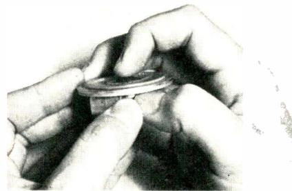
Fig. 5—Voice-coil drag can be detected by holding the interior as shown here and pushing the diaphragm in gently and then releasing it slowly.
