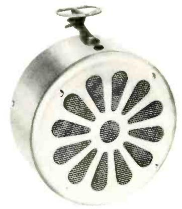
and baffle combinations containing an extended range 8-in. cone speaker. The speaker housing has an adjustable mounting bracket, designed for universal installation on walls, ceilings, poles and under roof overhangs. Specifications are: Power, 8 w. Impedance, 8Ω. Magnet, 3.16 oz. Alnico V. Dimensions 9 in. dia and 5 in. deep. Atlas.
