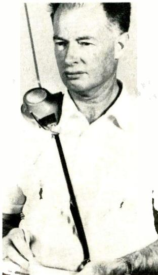
microphone, speaker and antenna in one housing. It was said that 25 of the units were used at the Cow Palace in San Francisco during the Republican Party convention. Features include noise elimination circuitry, push to talk button, and all aluminum construction, weight approximately 1 lb, complete with battery and leather case. Units were said to be exceptionally useful in inventory, production and traffic control. Mar-co.
