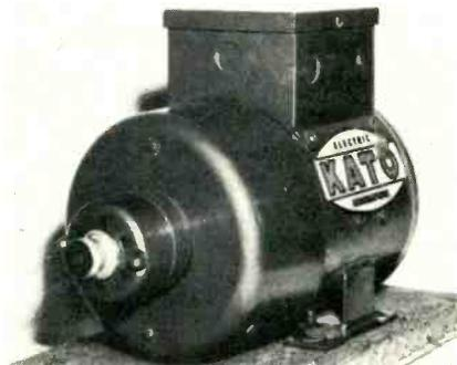
capacity of 350 w, 115 v, single phase. The unit has solid silver collector rings and silver commutator bars. Converters are available from 100 w to 10,000 w. The approximate weight is 24 lb. Size: 13¾ x 7¼ x 7 in. Kato Engineering.
