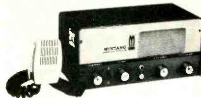
quency. The receiver is super-heterodyne with a tuned RF stage for maximum sensitivity 0.3 μV usable, the announcement said. Metrotek.
