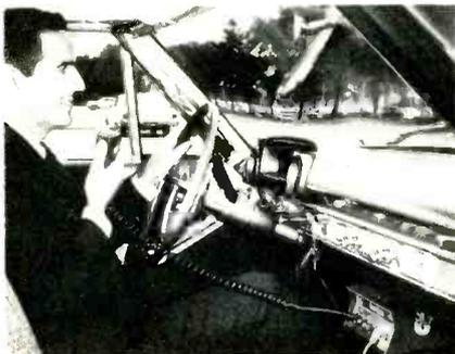
lation indicator shows that signal is being transmitted and voice is modulating properly. Squelch control eliminates background noise — also silences receiver until signal comes in, according to specifications. Slide switch converts unit to 3-w public address system, using auxiliary speaker. Earphone jack on front panel permits private listening with low-impedance earphones. Transistorized universal ac/dc power supply operates on both 117 vac and 12 vdc. B&K/Mark.
