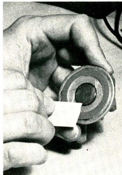
Fig. 6—Iron particles on the front of the diaphragm should be carefully removed with a piece of masking tape.
