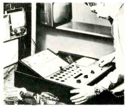
— including Nuvistors, Compactrons, 10-pins, Novars, Magnovals and Japanese, French and German tubes, the manufacturer reports. The tester can be used as a counter checker or self-service tube seller in your shop. Sencore.
