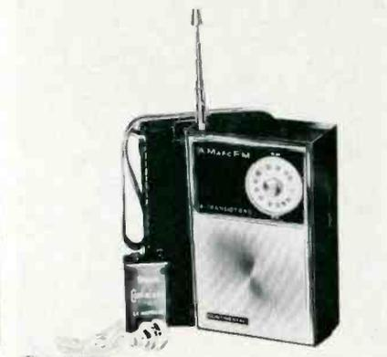
tured design, decorated with a chrome grille. The dimensions are 4 $\frac{3}{8}$  x 2 $\frac{3}{4}$  x 1 $\frac{1}{4}$  in. The chassis has 9 transistors and 5 diodes. Continental.
