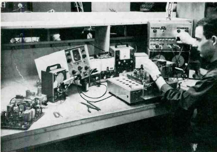
Test equipment at a factory TV IF alignment station includes kits and custom-built equipment.
