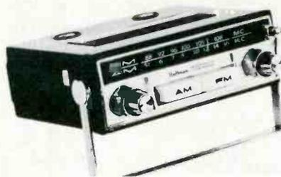
be unshathed from its mounting bracket and used as a battery-powered portable is introduced. The model 769 is 5 x 5 $\frac{3}{4}$  x 2 in. with a 2 $\frac{3}{4}$  in. speaker. It contains nine transistors, six diodes and one thermistor. Hoffman.
