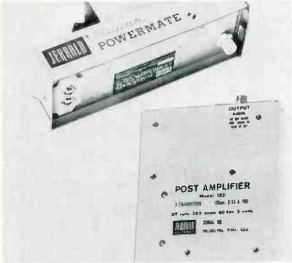
combined to form a powerful home TV reception device, according to the maker. The SPC is a boom mounted two transistor preamplifier and the 132 is a combination remote power supply and three transistor post amplifier. A single coax cable between the SPC and 132 units transport power up to the preamp and signals down to the post amplifier. Jerrold.
