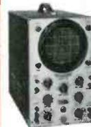
DC WIDEBAND 0-4.5 MC FOR COLOR & B & W TV SERVICE & LAB USE. PUSH-PULL DC VERTICAL AMP. BAL. OR UNBAL. INPUT. AUTOMATIC SYNC LIMITER AND AMP.
