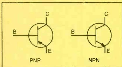
Fig. 2—PNP and NPN transistor symbols.
