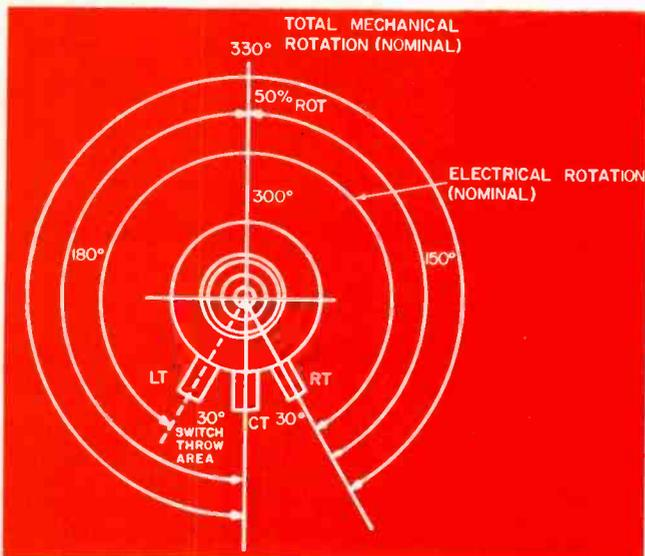
Fig. 1 — Electrical and mechanical rotation definitions for the popular 15/16 in. dia composition controls. The 50 percent electrical rotation point is 180 deg nominal from the CCW end or 150 deg nominal from the CW end (shaft end view).
