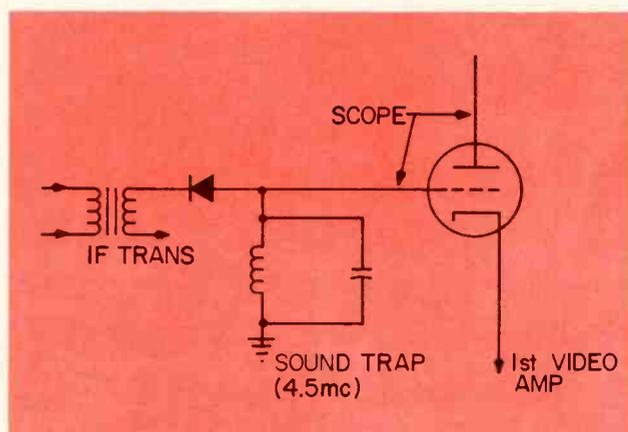
Fig. 2 — The 4.5 sound trap can be easily adjusted by observing the waveform on a scope at some point beyond the trap.
