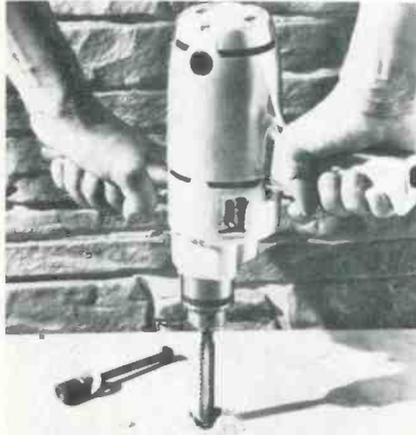
trol are combined to provide four speeds of 630, 730, 2200, and 2400 rpm with no load. Speed changes are made with a gear shift control located on the back of the handle. It measures 11 x 8½ x 3½ in. Weight without cord is 6½ lbs. Three-wire cord is 6 ft long. Wen.
