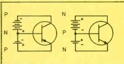
Fig. 5—Basic biasing of PNP and NPN transistors.
