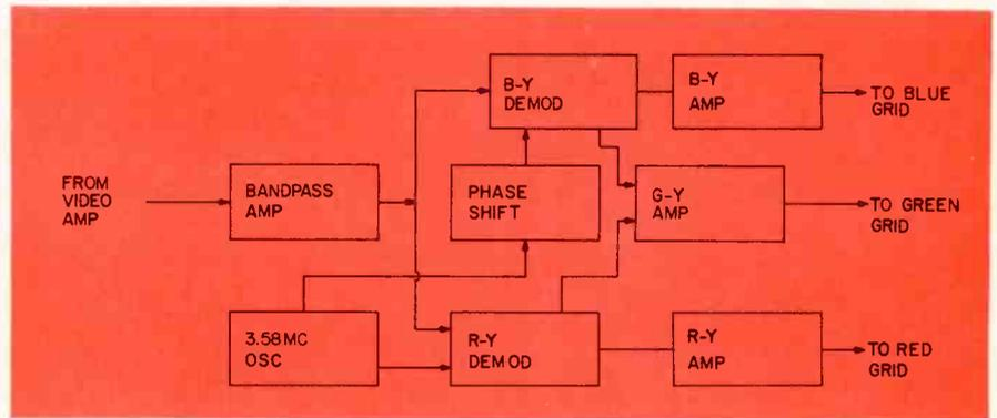
Fig. 1—Block diagram of chroma circuits of a typical color set.
