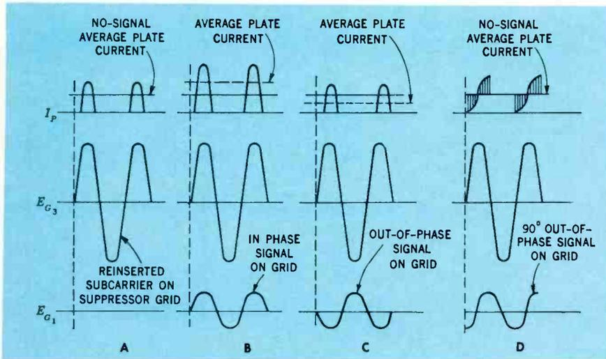
Fig. 7—Average plate current for various phase relationships of the two signals applied to a demodulator circuit.
