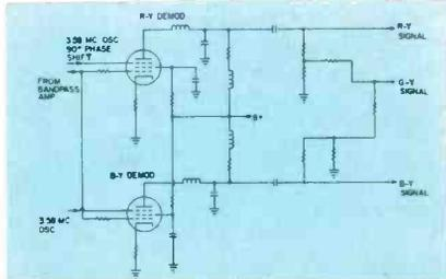
Fig. 9—A typical B-Y, R-Y synchronous demodulator.
