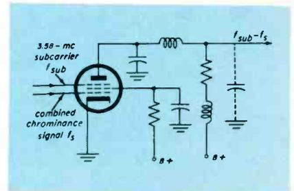
Fig. 6—Simplified diagram of a synchronous demodulator.
