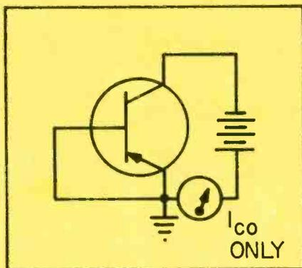
Fig. 8—Even with voltage on the collector it is reverse biased. Leakage current flows through the collector with the base at the emitter potential only.
