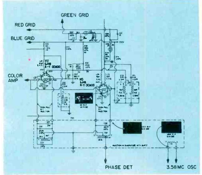
Fig. 11—High level demodulator used in Zenith 25MC30 color chassis.
