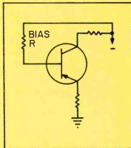
Fig. 9—Simple biasing system.
