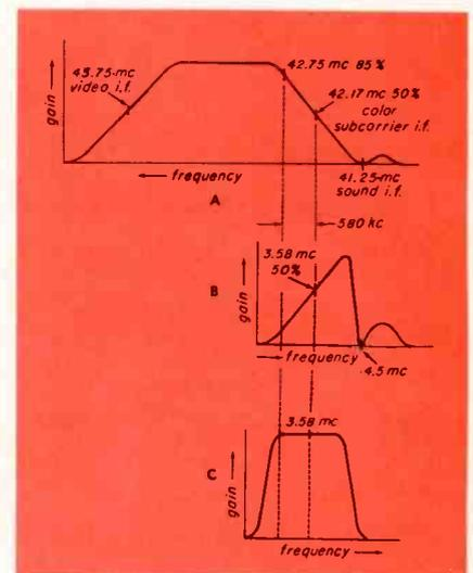
Fig. 2 (A)—IF response curve of a typical color receiver. (B)—Response curve of a color TV bandpass amplifier. (C)—Over-all chroma response of a color TV set.
