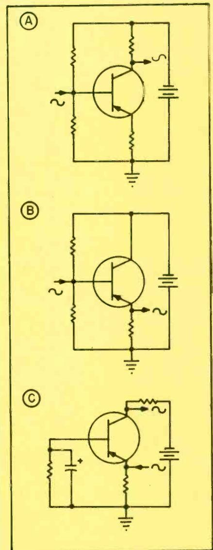
Fig. 12 (A)—Common emitter, (B)—common collector and (C)—common base transistor circuits.
