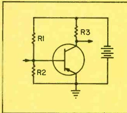
Fig. 6—Common emitter circuit.
