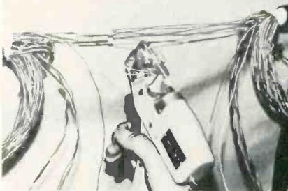
are inserted into the jaws of the gun without twisting and stripping the insulation beforehand. Operation of one trigger actuates an electric motor which twists the conductors together for a set number of turns. Operation of a second trigger applies battery potential to the twisted conductors which burns off the insulation, cuts off surplus conductor and welds the two conductor ends together. Jonard.
