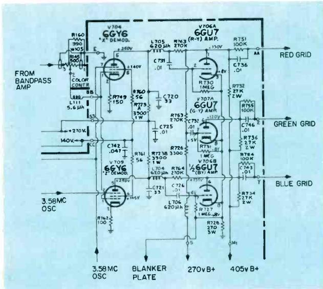
Fig. 10—Demodulator and color difference circuitry used in RCA CTC 16 color chassis.
