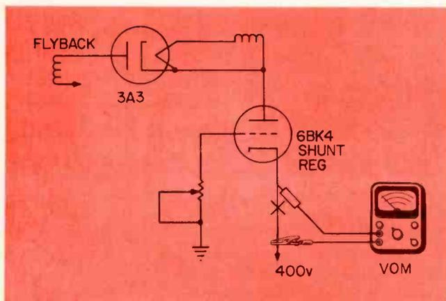
Fig. 1 — Current check on shunt regulator is important for 6BK4 shunt regulator tube.
