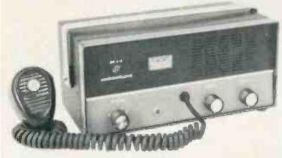
six of the available CB channels. A front panel switch determines the channel in use. A dual power supply is provided with 117 vac input for fixed station applications and 12 vdc for mobile applications. Hammarlund.
