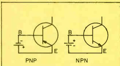
Fig. 3 (above) Fig. 4 (below) shows how PNP and NPN transistors are biased.
