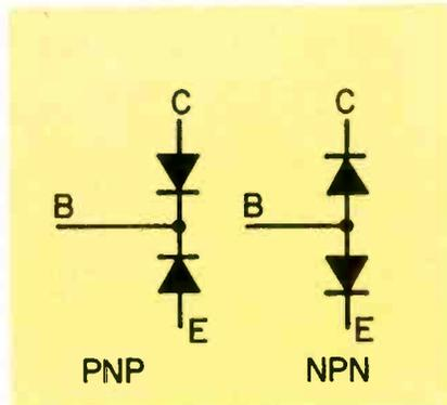
Fig. 1—A transistor is equivalent to diodes wired back to back.
