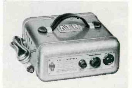
inverter is used for operating most 11 in. to 13 in. portable TV sets in automobiles, boats, mobile homes, buses, trucks, trains and planes. ATR.
