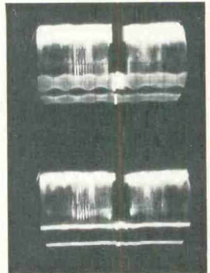
Fig. 3 (Top) — 4.5 Mc trap misadjusted, showing RF in waveform. A test pattern with a 400 cps tone was used as a signal. (Bottom) — The same signal with the trap properly adjusted for minimum 4.5 Mc RF.
