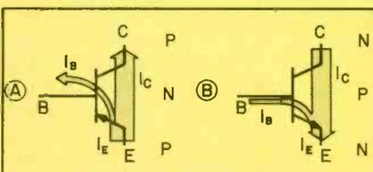
Fig. 7 (A)—A large percentage of the emitter current flows in the collector circuit of a PNP transistor. (B)—Similar flow in an NPN transistor.
