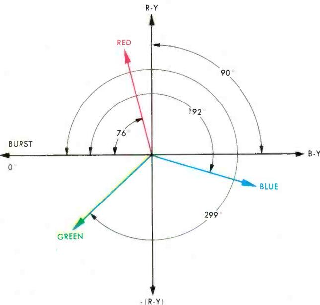
Fig. 5—Rotating vector diagram showing relationships of the three basic colors to R-Y and B-Y axes and phase angle relationships of the three basic colors from burst reference.
