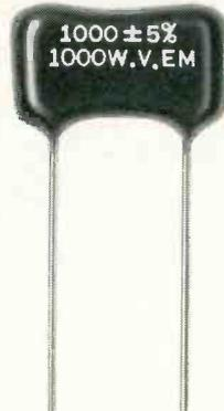
**ELMENCO** High Voltage Dipped Silvered Micas are solidly impregnated with corona resistant material. They operate to 125°C compared with 85°C for older molded silvered types. Greatly reduced size and radial leads make them ideal for printed circuit use. Extra reliability is assured through maximum moisture resistance. Capacitance, tolerance and working voltage are stamped on every unit.
