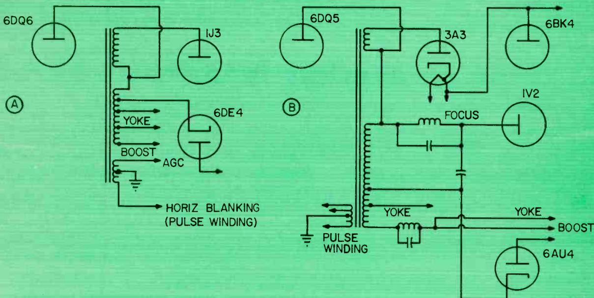
Fig. 1 (A) — Black-and-white flyback system. (B) — Color flyback system. Note similarity of both. Focus and regulator circuits are different in color sets.
