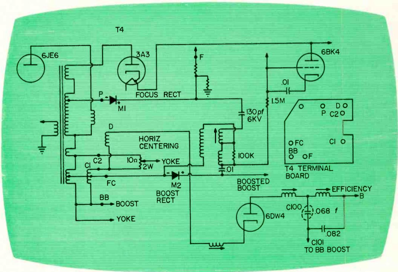
Fig. 2 — Schematic of focus and boosted boost section of Packard Bell 98C7D chassis. C100 was shorted out.
