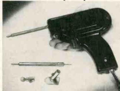
able, plus a kit with tip accessories. The standard tip is designed for splicing heavy electrical wires, appli-
