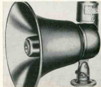
impedance taps, and 70.7 and 25 v power taps. HU15NT specifications are: Power, 25 w. Impedances, 45, 90, 180, 325, 670, 1000, 2000, 4000, 8000  $\Omega$ . 70.7 v line power taps, 15, 7.5, 2.5, 1.25, .65 w. 25 v line power taps, 14, 7, 3.5, 1.9, .92, .3 w. Frequency response 250-13,000 cps. Audio level, 123 db measured four ft on axis at rated power. Dispersion, 100 deg. Dimensions, 9 $\frac{3}{4}$  x 9 in. Write: Atlas Sound, 1419-51 39th St., Brooklyn, N. Y. 11218.
