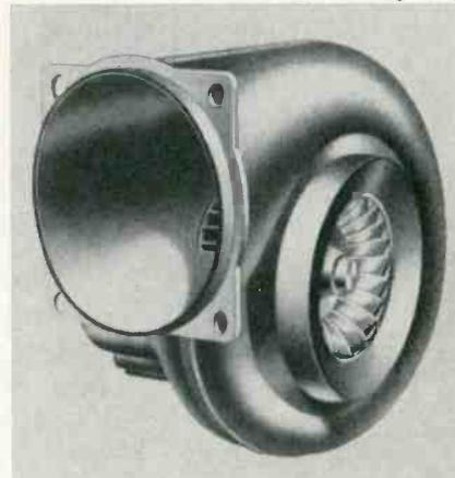
of the blower is 550 cfm at free delivery, and 200 cfm at 3/4 in. wg. Operating temperature range is -20°C to 85°C. Write: Rotron Mfg. Co., Woodstock, N. Y.
