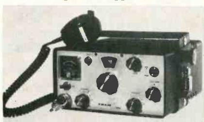
The XL100 has 13 tubes and 9 diodes. It has provision for locking the unit to the mounting bracket, and a key locking power-on switch. Write Tram Electronics, Inc., Lower Bay Rd., Box 187, Winnisquam, N. H.
