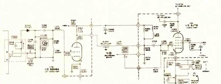
Fig. 4—Schematic of video detector, 1st video amplifier and final output amplifier.
