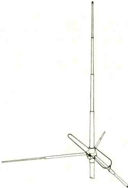
pattern, according to the announcement, is 360 deg circular. A coaxial female connector is incorporated into the weather-proof radial support assembly. VSWR is reported to be 1.5:1 or better and gain at 3.4 db over a quarter-wave ground plane. Mosley.
