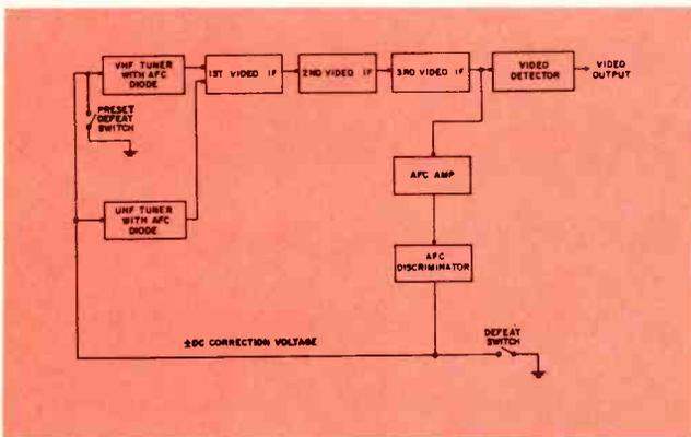
Fig. 6—Block diagram showing origin and application of AFC correction voltage Magnavox T904 color chassis.
