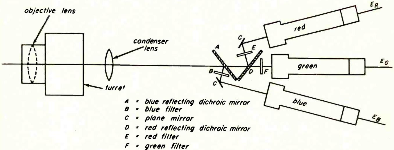
Fig. 4—The compatible color TV transmission system.
