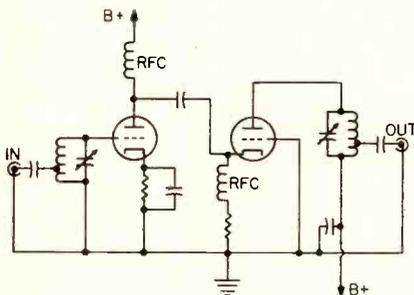
Fig. 2—Basic cascode amplifier circuit.
