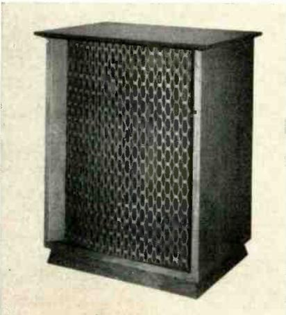
is adaptable for small rooms. The enclosure houses a 12 in. bass speaker, an exponential horn and a compression high-frequency driver. A two-section 3000 cps crossover network is also provided. The unit is rated at 20w, impedance 8 or 16 Ω and has a frequency response of 40 to 22,000 cps, the announcement said. Size 26 x 19 x 14 in. List \$231. Altec.
