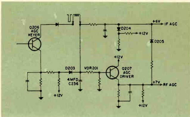
Fig. 12—Action of diode D205 in Magnavox T908 chassis.
