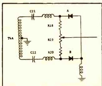
Fig. 2 (left)—Simplified schematic of synchronous demodulators in the G-E CB chassis.
