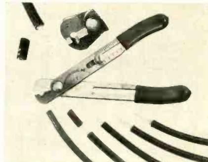
quality spring steel and the cutting edges are honed and heat treated to give long service life, according to the maker. Price \$1.98. Hunter.
