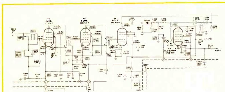
Fig. 3—The three stage video IF of the DO2 has frame grid tubes.
