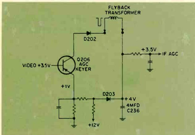
Fig. 10—Simplified schematic AGC keyer stage in solid state Magnavox TV.
