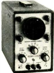
**New Model 435** — DC Wideband Scope. Top-quality DC 4.5mc scope with 3" flat-face CRT. Zener calibrator. Outputperforms 5" scopes three times its size, facilitates on-location color TV and other servicing. \$99.95 kit, \$149.95 wired.
