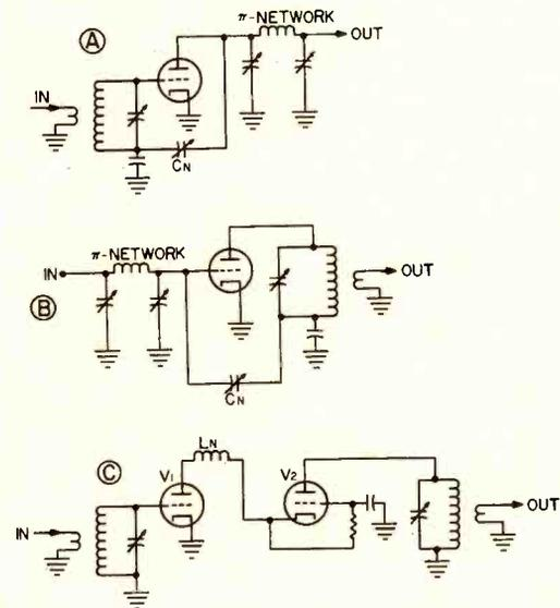
Fig. 4—Commonly used compromise neutralizing circuits. (A)—Bridge neutralization, divider on grid side. (B)—Bridge neutralization, divider on plate side. (C)—Series-neutralized cascode.
