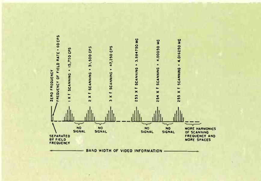
Fig. 2—Color signals are 'sandwiched' in between monochrome signals.
