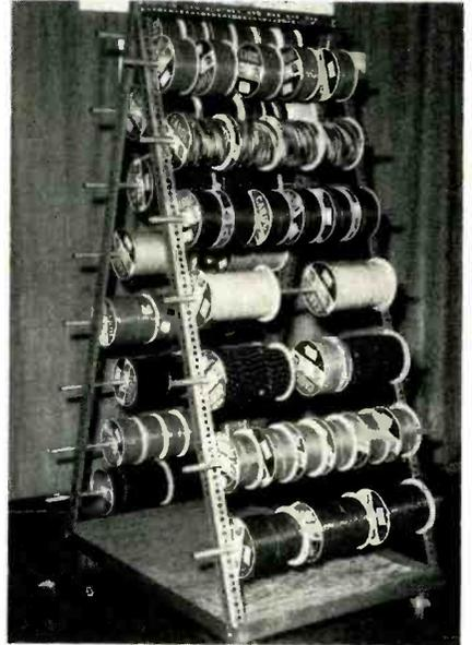
ball bearing wheels, according to the announcement. Empty spools can be replaced by one man. The model SP is 30 x 42 x 75 in. Net weight, 55 lb. Additional information including literature and prices furnished on request. Allcart.
