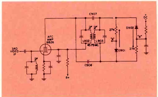
Fig. 7—AFC amplifier and discriminator, Magnavox T904.
