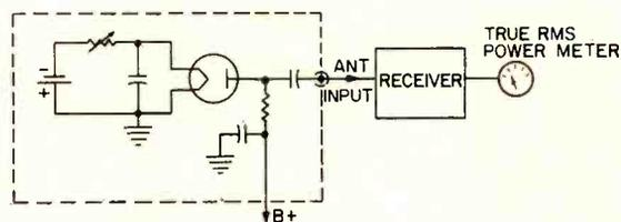
Fig. 5—Simplified noise generator and noise figure measuring circuit.
