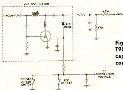
Fig. 8—AFC diode in Magnavox T904 tuner acts as variable capacitor when varying dc correction voltage is applied.
