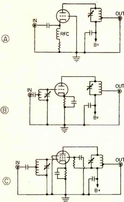
Fig. 1—Three amplifier types used in communications receivers. (A)—Grounded-grid triode. (B)—Grounded cathode triode. (C)—Grounded cathode pentode.
