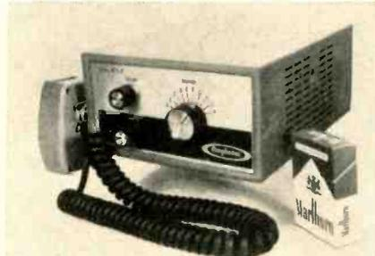
bile-base station transceiver and operates from 117vac or 12vdc. Complete specifications available on request. Amphenol.
