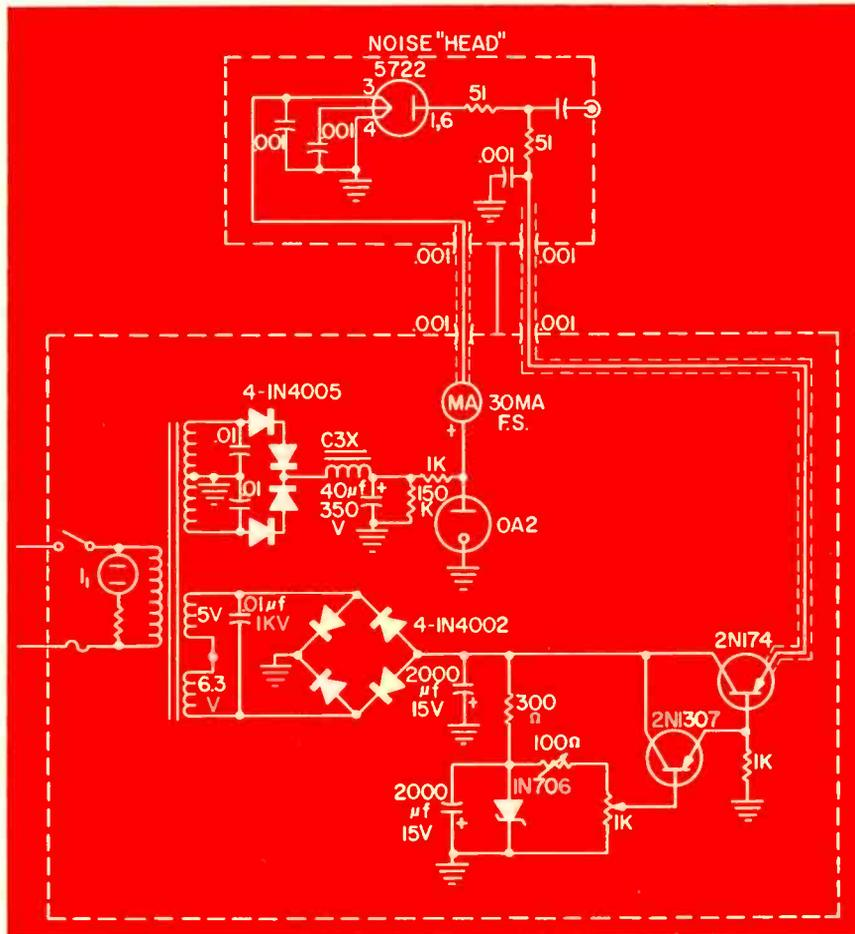
Fig. 6—Practical noise generator suitable for 25 to 450Mc.
