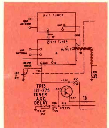
Fig. 5—AGC tuner delay stage in Zenith solid state chassis, 1M30T20.
