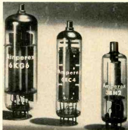
TV since they can deliver top-performance at B+ voltages of 240 to 270 v. The tubes currently available are the 6KG6 horizontal output pentode; 6EC4 damper diode and 3BH2 high voltage rectifier diode. Amperex.
