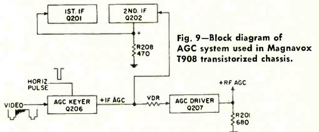
Fig. 9—Block diagram of AGC system used in Magnavox T908 transistorized chassis.
