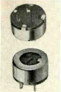
A line of economical - type trimmers, with hot molded carbon elements, is announced. Construction consists of the stable hot molded base and resistor with a carbon contact brush, pressure spring and cover. Adjustment is made by screwdriver. Size is  $\frac{1}{2} \times 5/16$  in. They are rated at 0.25w at 70°C, 300acwv. Values from 100Ω to 1M. Clarostat.
