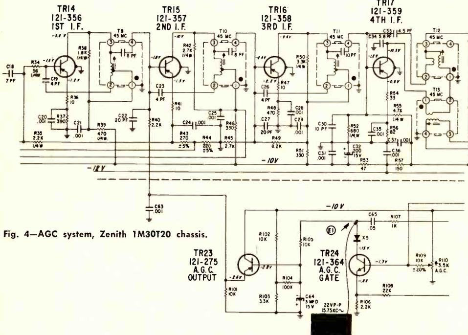
Fig. 4—AGC system, Zenith 1M30T20 chassis.
