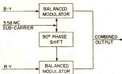
Fig. 5—Block diagram of balanced modulators.
