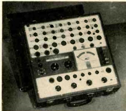
10-pin tubes, 12-pin compactrons, etc. — is announced. Known as the model 707, the dynamic mutual conductance tester permits checking other types in an emission circuit. B&K.
