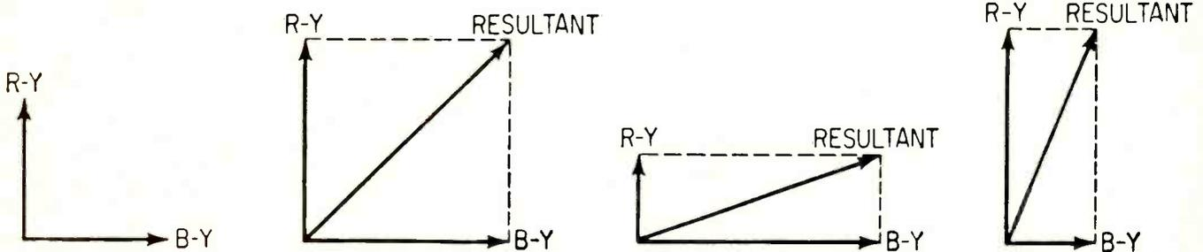
Fig. 6—Angular position and amplitude of the resultant carrier for various amplitudes of B-Y and R-Y. (A)—R-Y and B-Y vectors. (B)—Resultant when both signals are equal in strength. (C)—Resultant when B-Y is stronger. (D)—Resultant when R-Y is stronger.
