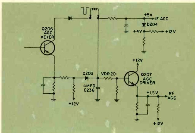
Fig. 11—Simplified drawing of T908 AGC system with driver stage added.
