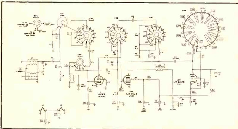
Fig. 1—Sylvania VHF tuner schematic.
