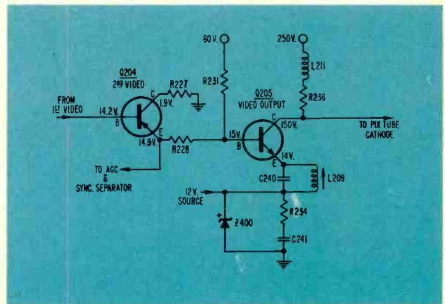
Fig. 13—First video amplifier stage, Westinghouse chassis V2483-1.
