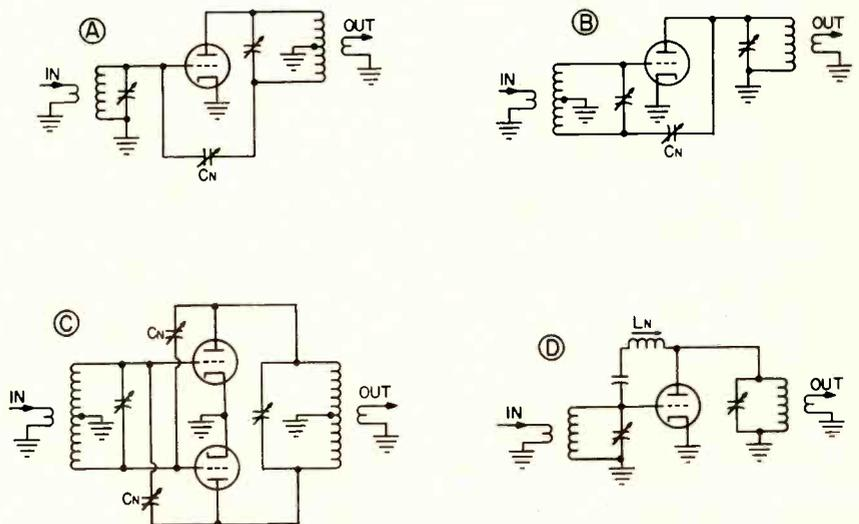
Fig. 3—Typical basic neutralization schemes. (A)—Hazeltine. (B)—Rice. (C)—Cross-neutralized push-pull. (D)—Coil neutralization.
