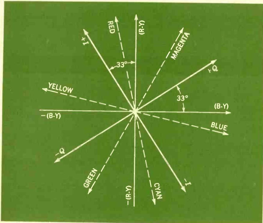
Fig. 7—Any color in the spectrum can be formed by varying the amount of R-Y and B-Y voltage.
