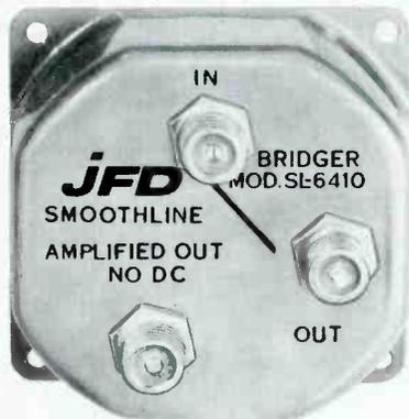
MHz, 470 to 890MHz; impedance 75  $\Omega$ ; isolation between through line and tap, 35db; through-line loss less than 1.0db; output gain, VHF, 1db UHF, -1.5db; tilt control range, VHF, 5.5db; dimensions; 2 5/16 x 2-5/16 x 1 1/2 in. List price is \$37.50. JFD.
