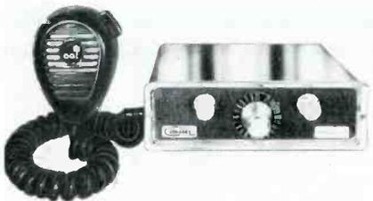
incoming signal indicator which lights automatically when receiving S6 or stronger signals, an illuminated channel selector, auxiliary speaker jack, modulation indicator and single-knob tuning. Size: 5¾ x 6¼ x 1⅞ in. Price \$149. Courier.
