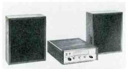
flutter is less than 0.25% RMS, output power 12w (6w channel); signal-to-noise ratio better than 45db, frequency response 70Hz to 10kHz and channel separation 35db. Craig.
