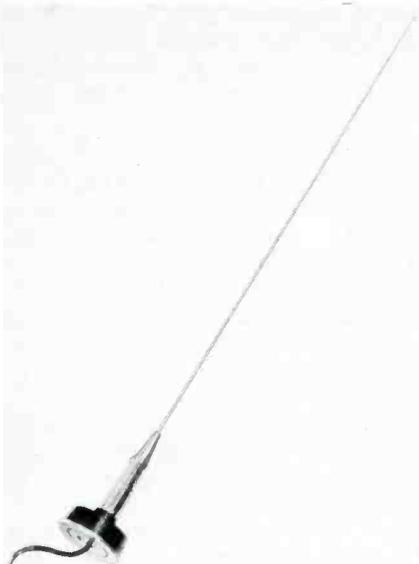
hole from 3/8 to 3/4 in. The line also features an etched copper loading coil that is photographically etched instead of printed. A triple moisture seal is included in the housing. The antenna whip is 17-7 PH stainless steel. The line includes four models; roof mounted, truck lip mounted, magnetic mounted and a shorty rooftop model. High-Gain.
