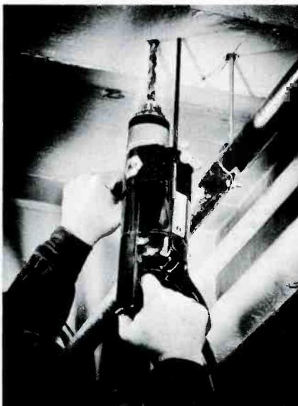
ducts and lighting fixtures. The No. 816 hammer/drill features an exclusive insulated shift collar for easy and safe conversion from hammer to drill action. Black & Decker.
