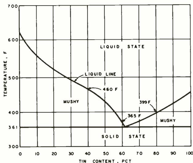
Melting Temperatures of Various Solder Alloys
