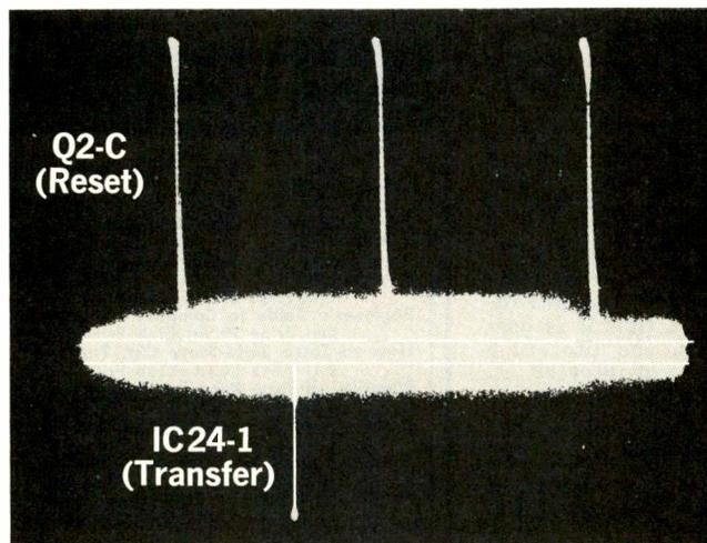
Fig. 10—By increasing the scope sweep rate we can more clearly see the timing relationship between the reset and transfer pulses.
