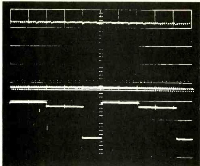
Fig. 6—Comparing the 1kHz signal applied to Inverter B (upper trace) with the 10Hz applied to capacitors C11 and C12 (lower trace).
