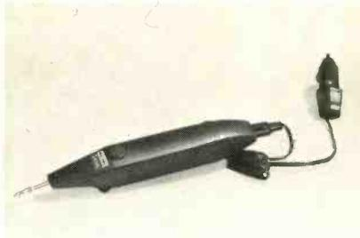
plug allows charging of the soldering iron while traveling between jobs or
