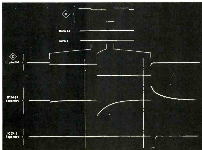
Fig. 5—Differentiated pulses from the 10Hz signal are used for producing the transfer signal.
