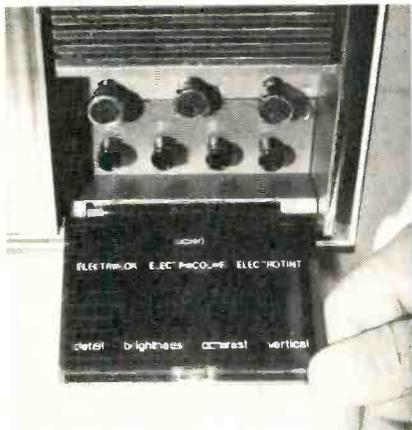
A panel door hides most of the controls on the front panel of the TV set.
