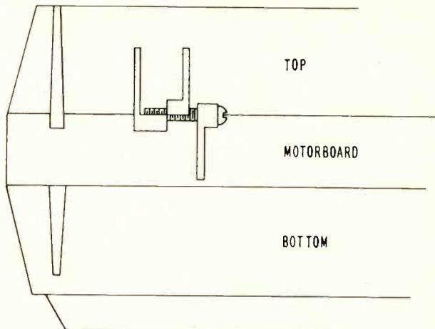
size No. 8-32 tap to thread a hole for a No. 8-32 screw,  $\frac{3}{8}$  in. long to replace the broken hinge pin.
