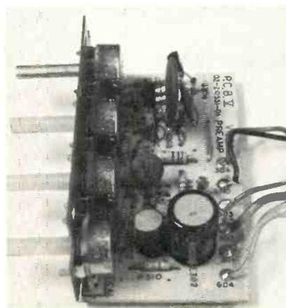
The DETAIL, BRIGHTNESS, CONTRAST and VERTICAL controls are mounted on a separate video preamp board.
