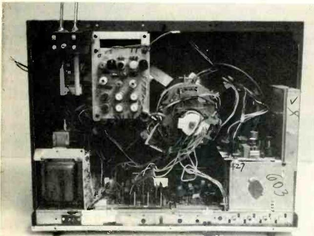
Rear view of Electrohome's Capri color-TV set with an open display of components and a slide-out chassis.
