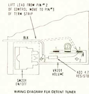
WIRING DIAGRAM FOR DETENT TUNER
