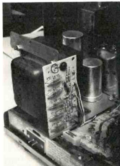
The fault indicator board is mounted vertically on the main chassis and monitors the five important voltages in the power supply. Should excess circuit current cause one of these voltages to drop, the corresponding bulb will light.
