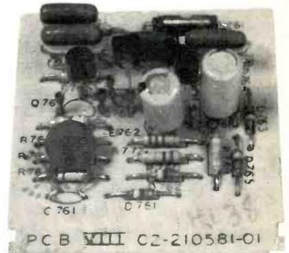
The auto-saturation printed-circuit board employs edge connectors and plugs into a socket on the main small signal printed-circuit board.
