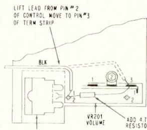
WIRING DIAGRAM FOR DETENT TUNER
