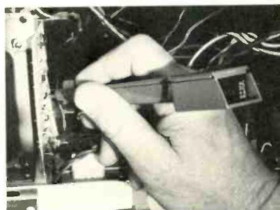
Measurements are digitally displayed at the end of the probe.
