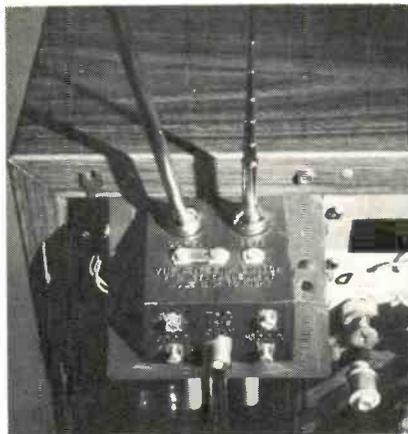
A 75Ω cable connector on the antenna block allows direct connection to cable systems or coax antenna system without additional adapters.
