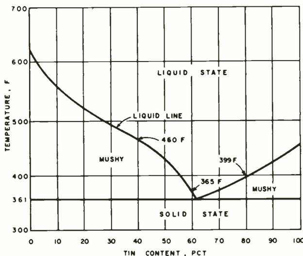
Melting Temperatures of Various Solder Alloys
