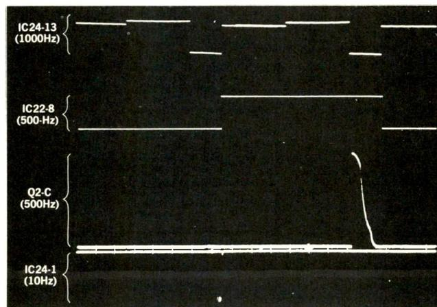
Fig. 11—Timing relationships exist between the applied 1kHz signal and the resulting *gate*, *transfer* and *reset* signals.
