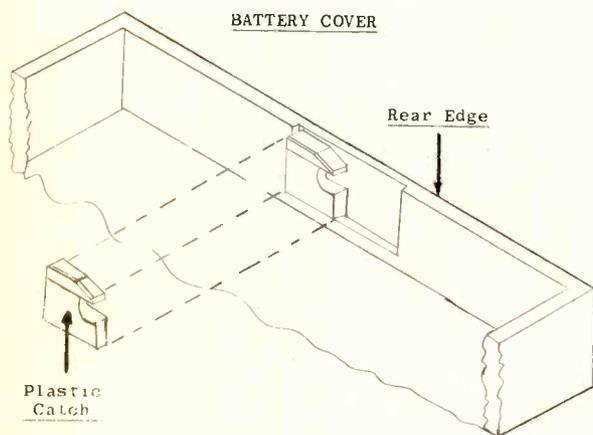
the old cover by sliding the blade of a small pen knife between the catch and the cover, very carefully prying it loose.
