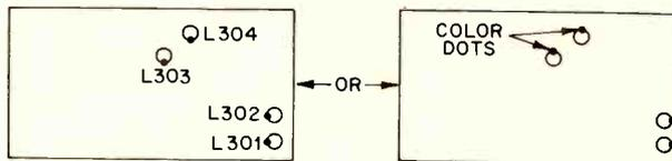
of the panel. In either of these two combinations, the coils are oriented so that stray 60Hz hum pickup is cancelled out.
