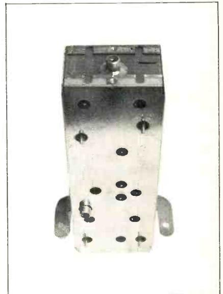
This rugged metal-cased factory serviceable IF module can be substituted in the field without requiring alignment.
