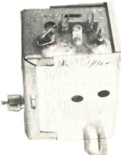
The AFT module is coupled to the IF module with a phono-type jack connector and is mounted on the top of the main chassis.
