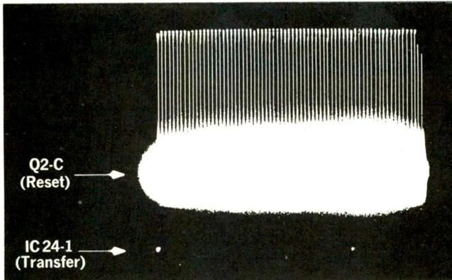
Fig. 9—There are a hundred reset pulses for every transfer pulse.
