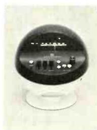
solid-state modular unit. The unit employs 3 IC's, 1 FET, 10 transistors and 12 diodes. The stereo multiplex frequency range is from 88 to 108 MHz, while AM covers frequencies
