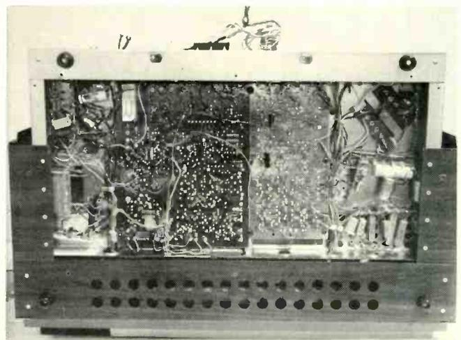
After removing a panel the complete underside of the chassis is exposed, making solder connections very accessible.
