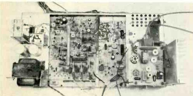
Top view of the solid-state color-TV chassis with road-mapped circuit boards to simplify identification of components.
