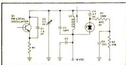
Fig. 3—FM local oscillator circuit employed in several Bendix-produced AM/FM stereo radio models.
