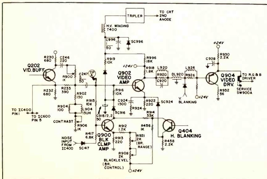
Fig. 1—Automatic Black Level circuit employed in GTE Sylvania's E20/21 color TV chassis.
