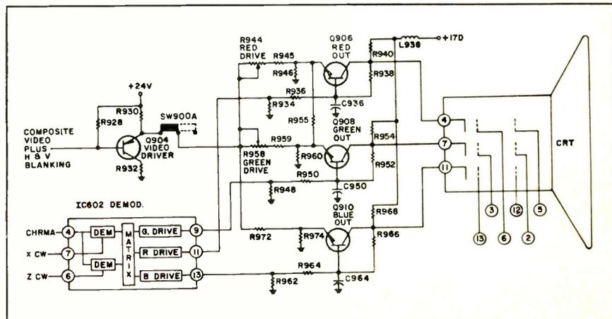
Fig. 2—The R, G and B amplifier, demodulator and video output circuits employed in GTE Sylvania's color TV chassis E20/21.
