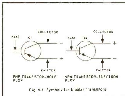
Fig. 9-7. Symbols for bipolar transistors.
