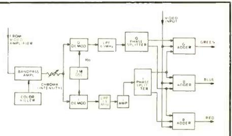
Fig. 12-7. An example of IQ demodulation.
