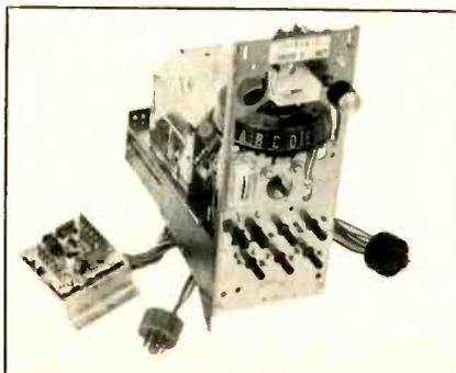
Fig. 5—The control module is side mounted, to the lower left side of the control panel cluster.
