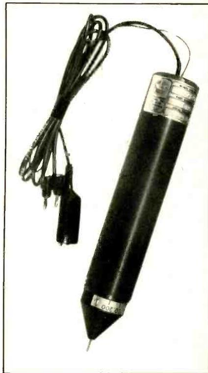
NLS RMS Measurement Probe Model RMS-10. For more information about this instrument circle 108 on the Reader Service Card.
