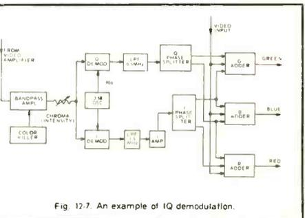
Fig. 12-7. An example of IQ demodulation.
