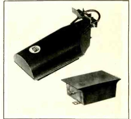
is matched to 300 ohm antennas. Downlead and output impedance are 75 ohms. A built-in 12 dB FM tunable trap can be used to eliminate interference from a local FM station. For reception in deep fringe areas, noise figure of the unit is very low, 6 dB at VHF and 8 dB at UHF. Price is \$97.50.
