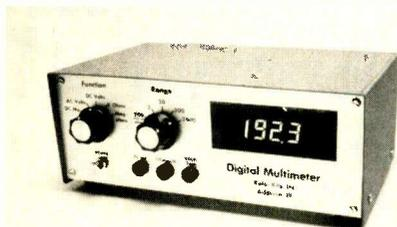
addition to DC voltage ranges from 200 mv to 2000 volts the meter has ACV, DC ma, K Ohms and a separate Megohm range that goes to 2000 Megohms full scale. The multimeter is available with either the Litronix ½-inch LED's as Model 75A priced at
