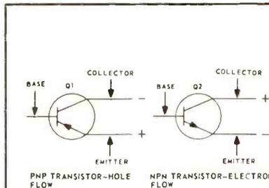
Fig. 9-7. Symbols for bipolar transistors.
