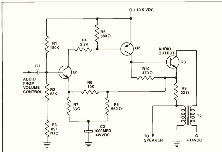
Fig. 1—Audio power amplifier circuit used in some Bendix-produced AM/FM stereo car radios of 1969-70 vintage.
