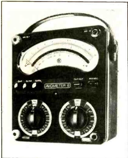
external power supply), plus make decibel readings on the AC volt scale. Easy-to-read, clear, linear scales with anti-parallel mirrors, plus unique overload protection are employed in all AVO 8 instruments. All of the instruments receive a 7 kv flash test before they leave the factory. Price is \$215.
