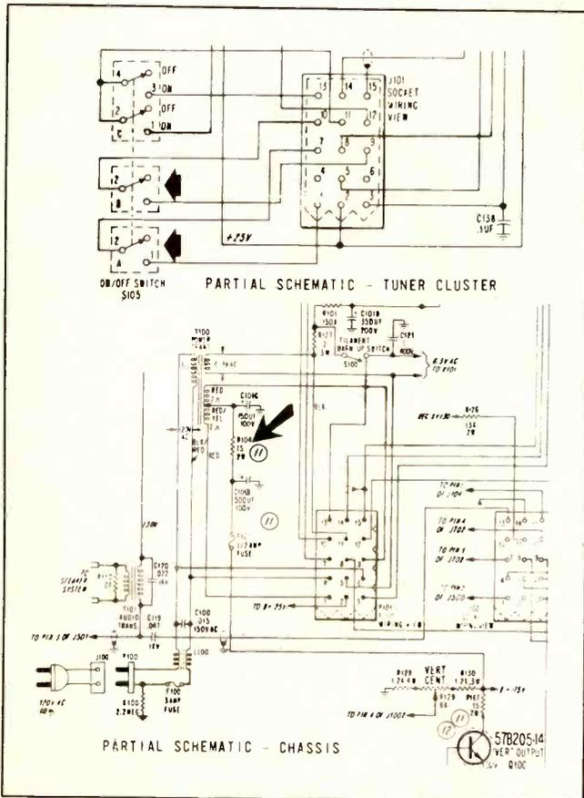
are opened by sections A and B of S105. With one switch section open, the AC circuit is incomplete, resulting in excessive current in R104.
