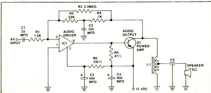
Fig. 5—IC-equipped audio circuit used in FM receivers produced by Motorola for imported cars.
