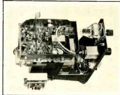
Fig. 3—The Remote Control Cluster has the remote receiver chassis mounted above the 21-position UHF/VHF strip tuner.
