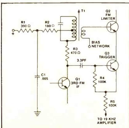
Fig. 4—Limiter section employed in Bendix-produced Ford FM receivers.
