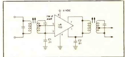
Fig. 7—IC-equipped FM IF amplifier stage employed in many Motorola car radios. (In most designs, four of these stages are connected in cascade.)
