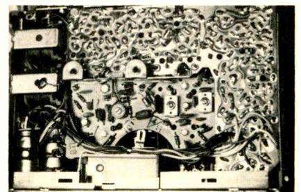
Fig. 2—Top view of the circuit board of Bendix-made Ford AM/FM stereo radio of late '60s/early '70s vintage.
