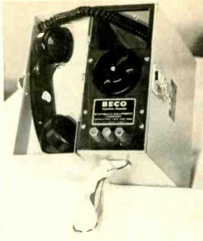
ment Co. Billed as "the first commercially produced field telephone since the introduction of its predecessor, the famous U.S. Army EE8," the new phone provides temporary and portable telephone service for construction
