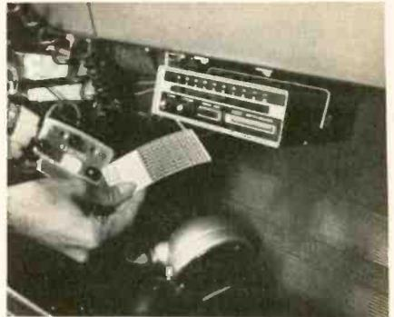
MHz, 150-170 MHz, 450-470 MHz, and 490-510 MHz). Antennas that cover all bands—LO, HI, UHF—are included with the unit, which measures 7 3/4 in. wide x 10 in. deep x 2 1/2 in. high.
