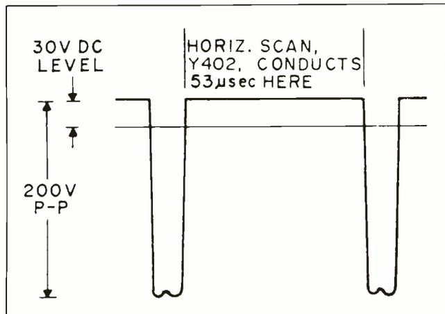
Fig. 14—Horizontal retrace pulses used in scan rectification.
