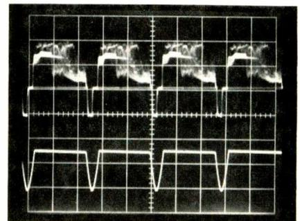
Fig. 4—Photo of the two 'keying' pulses required for conduction of AGC keyer transistor Q3 in Fig. 3. Top) Negative-going horizontal sync pulses in composite video signal applied to base of Q3. Bottom) Flyback-originated negative-going horizontal pulses applied to the collector of Q3.
