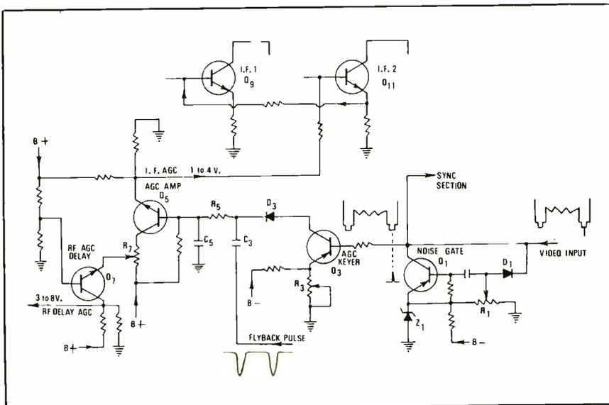
Fig. 3—A typical all-solid-state keyed AGC system.
