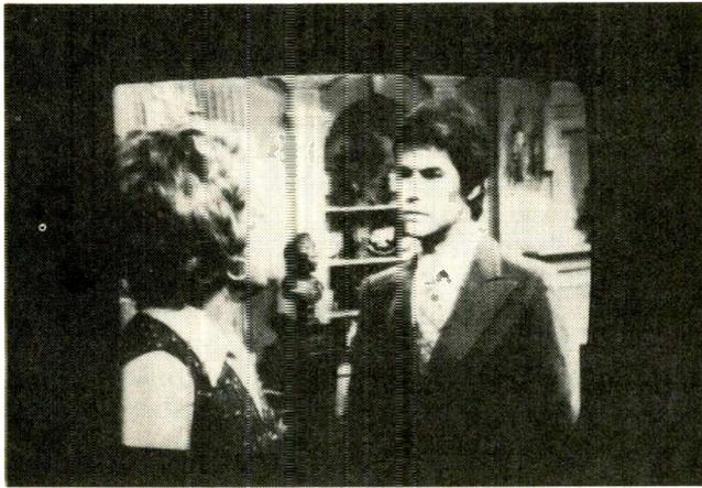
Fig. 6—Viewable picture even at a line voltage of 50V.
