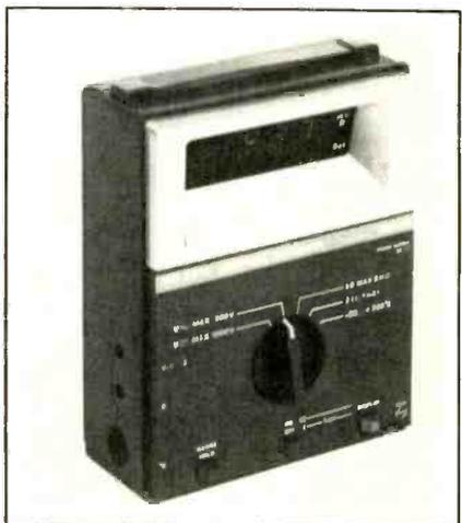
means of a range hold button. This PM2514 meter also has a low battery indication separate from the numeric display, and has an optional external
