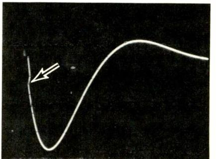
**Fig. 8—**This is an expanded scope display of the left portion of the waveform in Fig. 7. Arrow points to the "glitch" caused by a defective HV relay.
