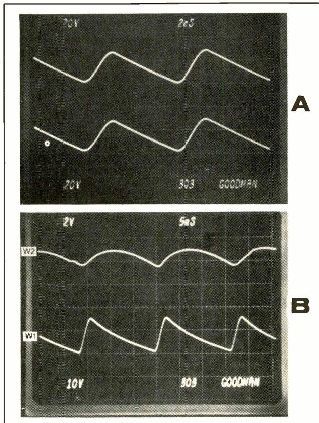
Fig. 25—Waveforms indicate a shorted choke.
