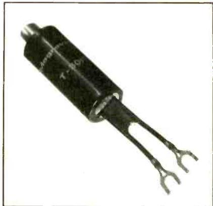
clude: high phase balance, low insertion loss, effective filtration and voltage blocking capacitors. The unit has a die cast metal casing and plastic cover, plus heavy-duty twin leads with soldered and crimped lugs.
