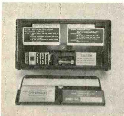
Rear view of Dana Model 2100A Digital VOM with cover of battery/fuse compartment removed. Single non-chargeable 9-volt battery provides one year of operation.
