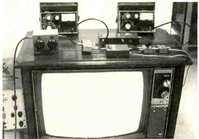
Fig. 4—Photo shows good picture quality resulting from a  $150 \mu\text{V}$  ( $-16.5 \text{ dBmV}$ ) signal amplified through a single-stage 15-dB amplifier with a rated N.F. of 3.3 dB, which provides the tuner with an  $840 \mu\text{V}$  ( $-1.5 \text{ dBmV}$ ) signal.
