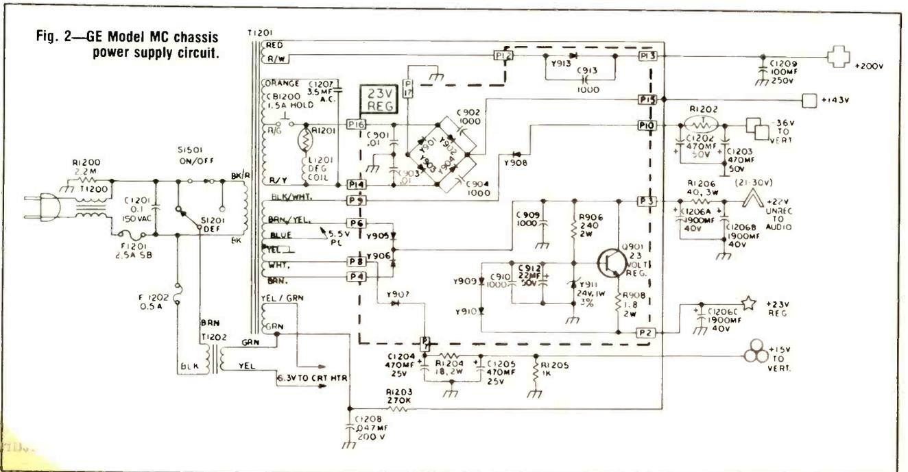
Fig. 2—GE Model MC chassis power supply circuit.
