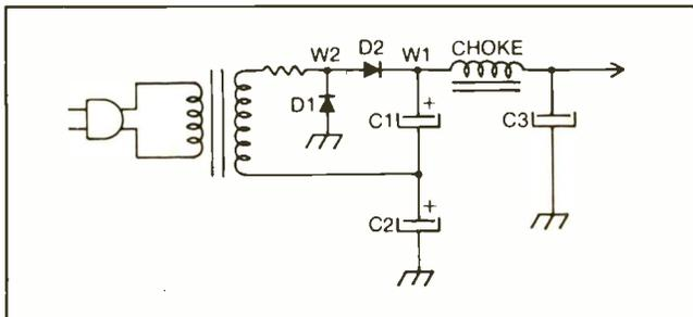
Fig. 21—Full-wave doubler circuit.
