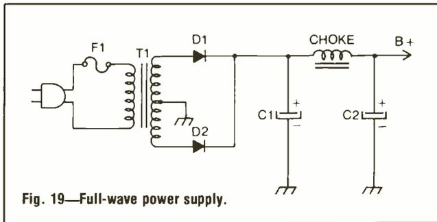
Fig. 19—Full-wave power supply.
