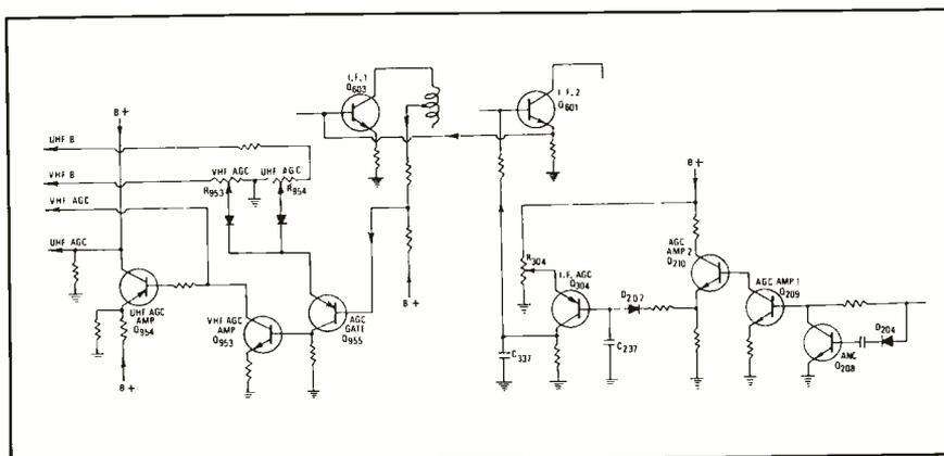
Fig. 5—Simplified schematic diagram of peak detection AGC system used in some Sony color TV receivers.
