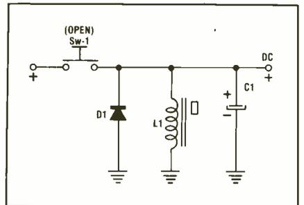
Fig. 6—Diagram of an inductive power supply circuit that could be a solenoid, relay coil, flyback coil, or deflection yoke.
