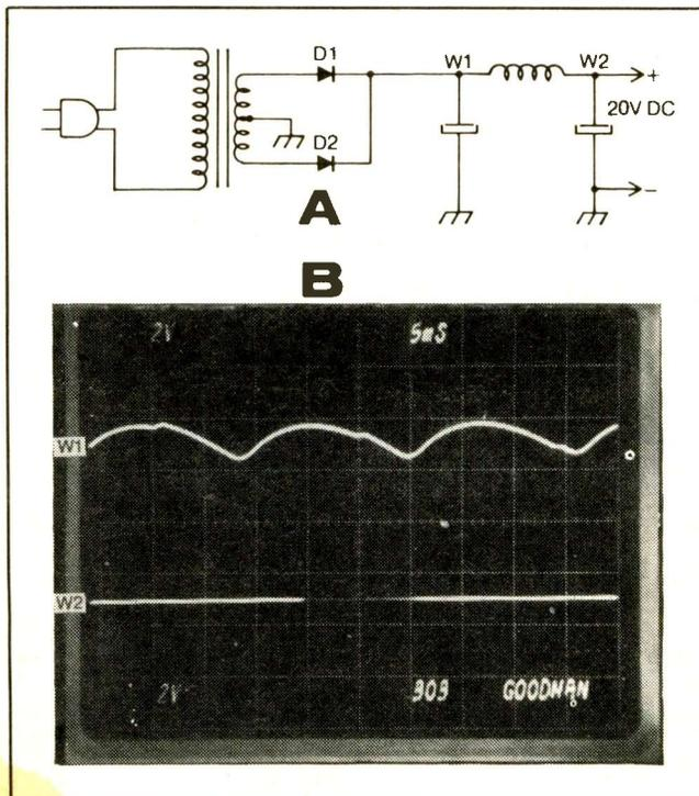
Fig. 22—Low voltage power supply with scope traces.
