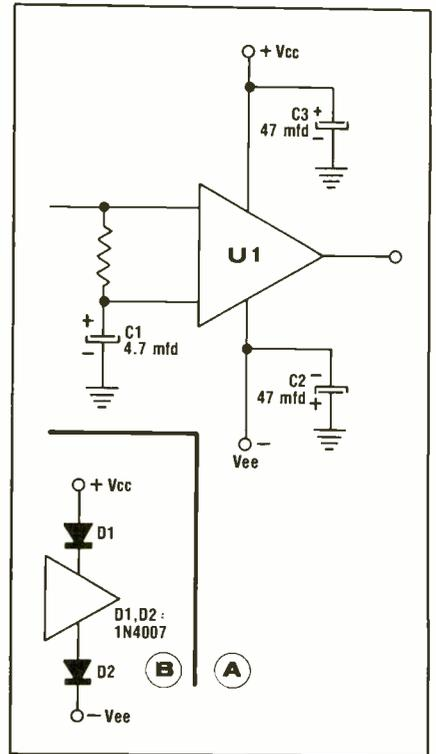
Fig. 5—This is a common type of IC linear circuit configuration, serving as an IC amplifier or signal processor device.
