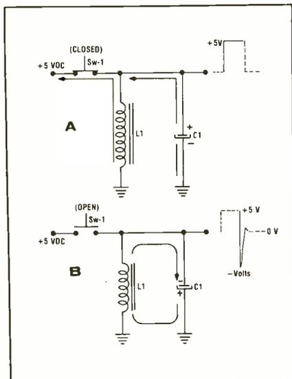
Fig. 7—Diagrams of an inductive power supply circuit without a suppressing diode, in the 'on' position (7A) and the 'off' position (7B).
