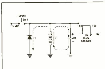
Fig. 8—The inductive power supply shown in Fig. 7 with the suppressing diode added to the circuit in the 'off' position.
