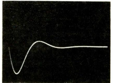
**Fig. 7—**A typical waveform taken across a 50 ohm dummy load in a properly operating defibrillator.
