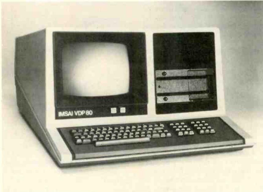
Fig. 5—Complete, self-contained, desk-top computer system intended for small business applications (courtesy Imsai Mfg. Corp.).
