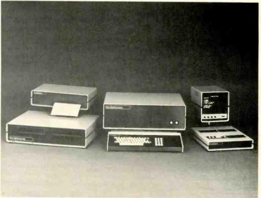
Fig. 3—Complete computer system based on a microprocessor CPU (courtesy of The Digital Group, Inc., Denver, Co.).
