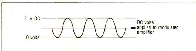
Fig. 2 AC "swing" require from modulator is twice the applied DC (peak to peak).
