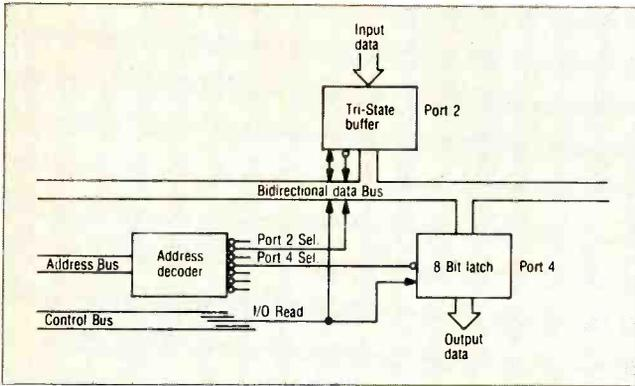
Fig. 4—Typical input/output logic of a system, showing one buffered input port and one latched output port. Address decoder and command line from the Control Bus govern the data flow, injecting or extracting data into or out of the data bus at the proper time.
