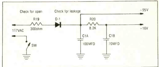
Fig. 4-A schematic diagram of the ac voltage dropping resistor (the resistance may vary between 150 and 450 ohms).
