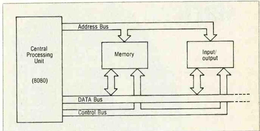
Fig. 1—General structure of computer system. The processor chip sends out addresses and commands, setting up two-way communication on the data bus. Buses can be extended, as shown on the data bus, to accommodate additions to a system.
