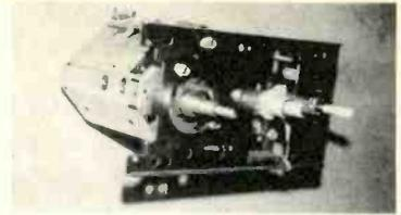
This is a wired and tested combination VHF/UHF tuner sub unit that has its own AC power supply and works equally well on color or b/w...tube or transistor sets...The VHF tunes channels 2 thru 13...The UHF is a detent (the kind that clicks for each channel) and tunes 14 thru 83.
