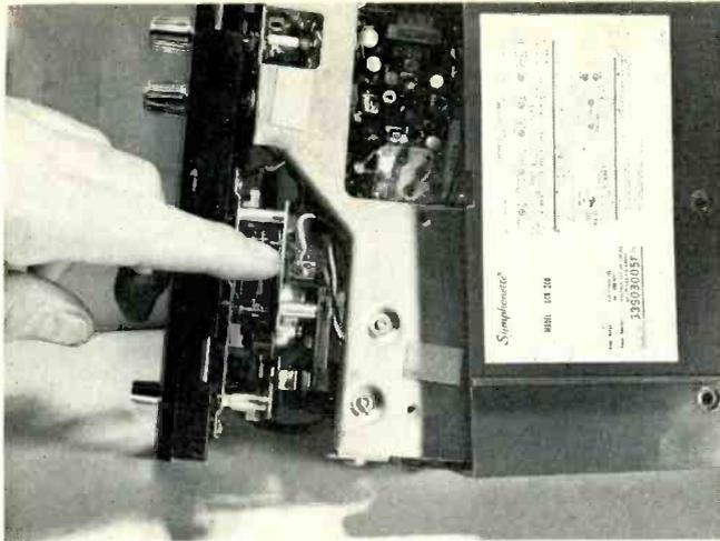
Fig. 2-Check the on-off switch continuity with the VOM, the on-off switch is located on the clock assembly in this Symphonette model LCR200.
