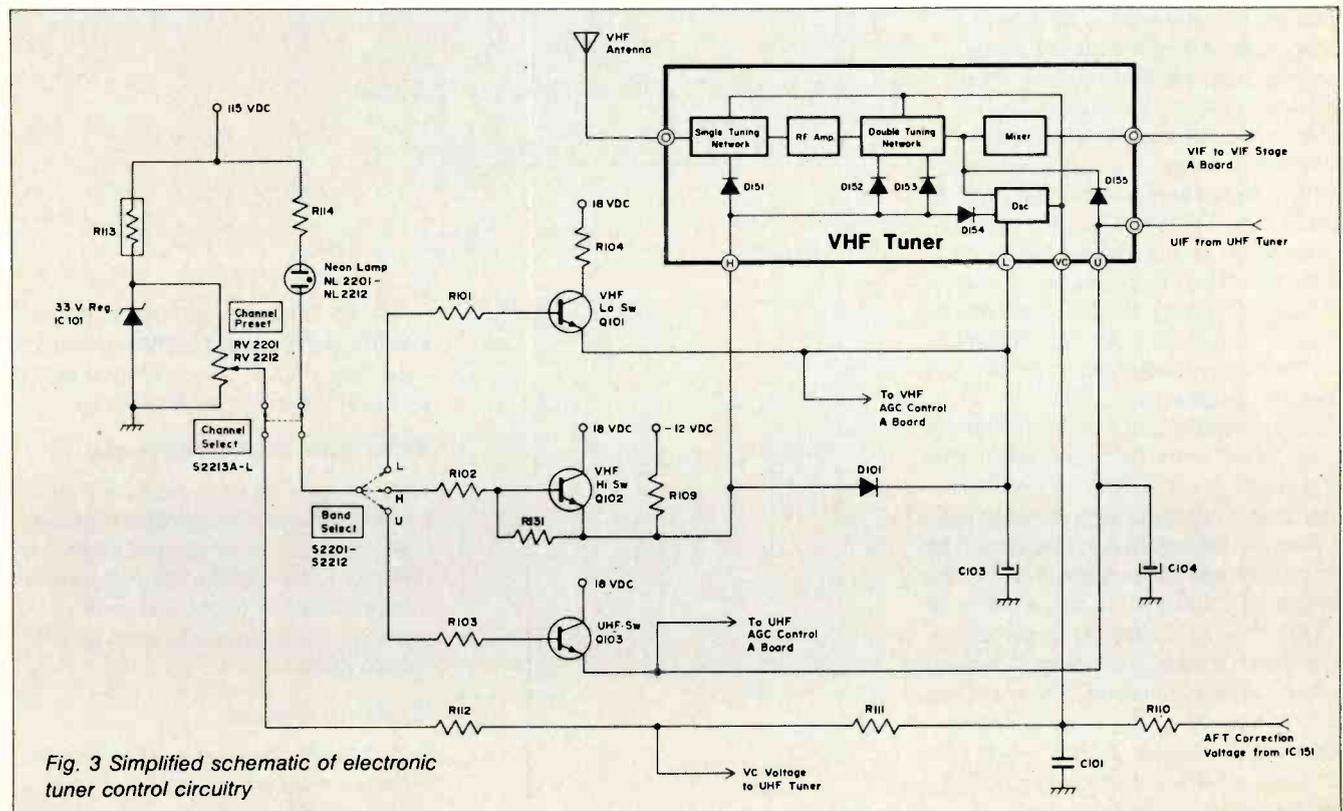
Fig. 3 Simplified schematic of electronic tuner control circuitry
