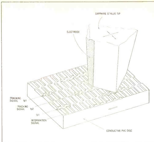
Fig. 1 Information and tracking signals are recorded on the disc surface as fine pits.
