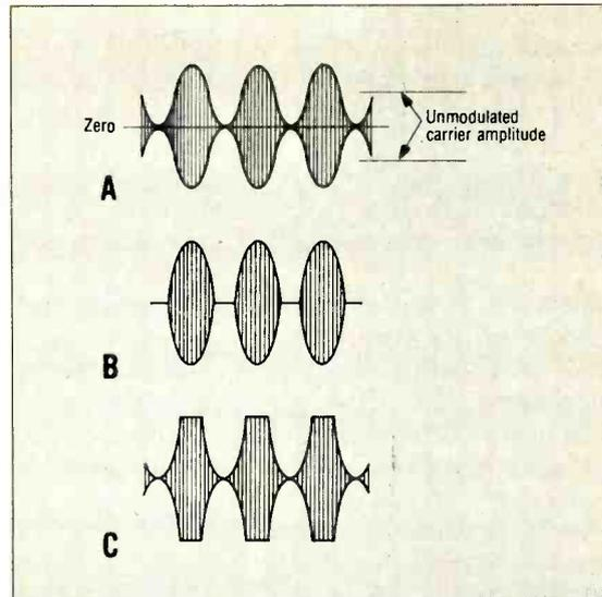
Fig. 3A Sine wave modulated carrier (100%). 3B Overmodulated carrier 3C Peak flattening due to inability of modulated amplifier to provide peak output power.
