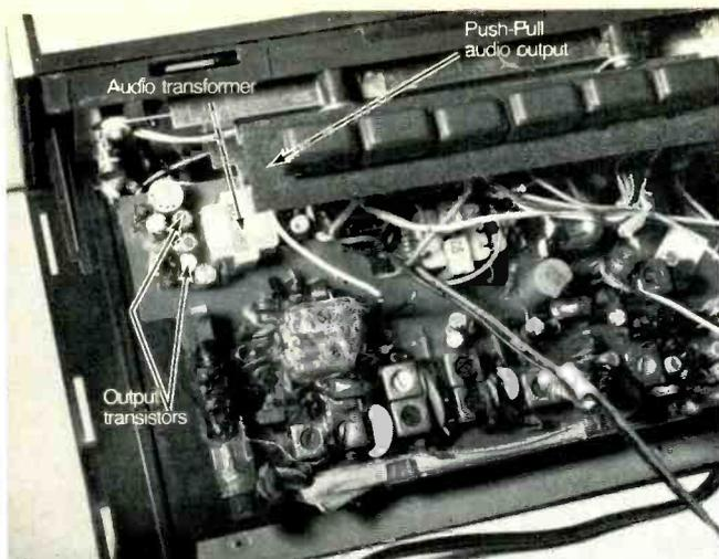
Fig. 8-Notice the two small audio output transistors bunched near the audio output transformer in this Lloyd's J-627G model.
