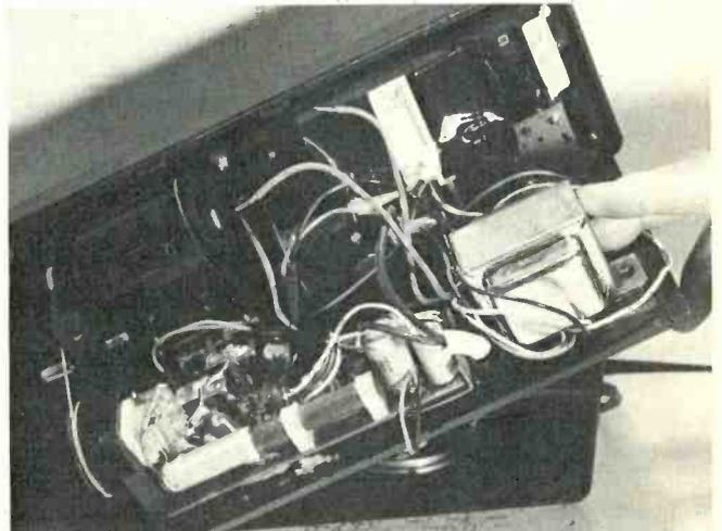
Fig. 5-Some table and portable receivers have a power transformer to operate the radio and digital clock circuits (Dyn model DS4555).
