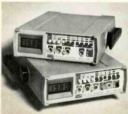
to 1 miliohm. The accuracy is reportedly .1% on dc and the instruments will hold this accuracy for at least one year. Both the 8010A and the 8012A are protected against transients to 6000V and against voltages up to 600V (400vRMS) applied to the current terminals. The prices are \$239 for the 8010A and \$299 for the 8012A.
