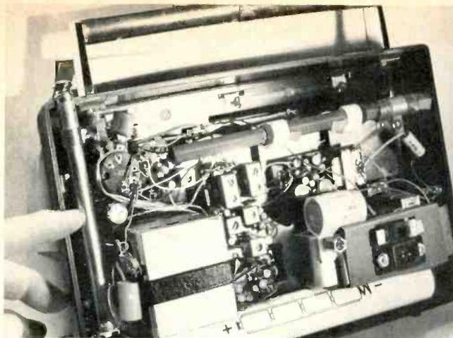
Fig. 6-A tunable squealing noise was heard across the entire band in a Magnavox IR-1201 3-band radio. The finger points at the defective decoupling capacitor.
