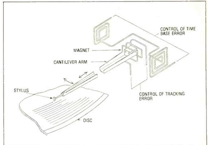
Fig. 2 Diagram showing the electro tracking system.
