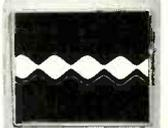
27 MHz "CB" envelope and modulating signal
