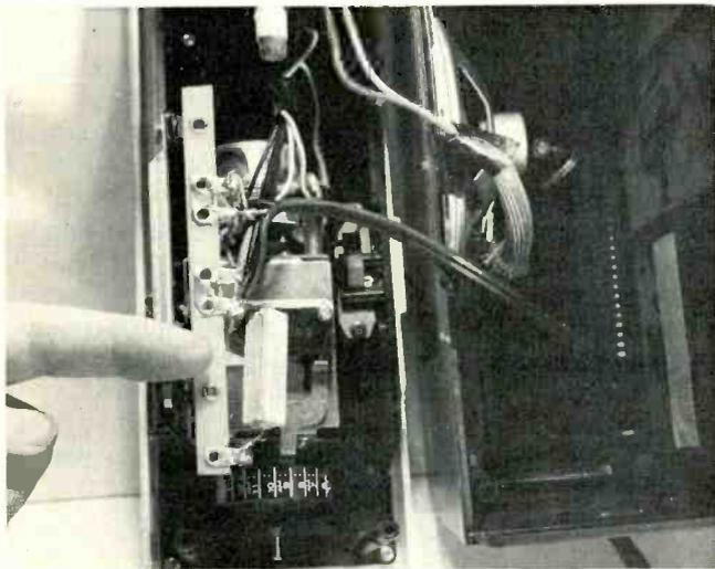
Fig. 3-A photo showing the size and where the ac voltage dropping resistor is located in many table model radios.
