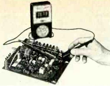
cept for the ½ digit. Ranges of the Model 3400 are 200 mv to 500 v ac and dc in 5 ranges, 2 to 2000 ma ac and dc current in 4 ranges and 200 ohms to 20 Megohms in 6 ranges. The ohmmeter features high and low power ohms ranges for semi-conductor circuit resistance measurements. The Model 3400's price is \$140 with test probes, battery, instruction book and 1 year warranty.
