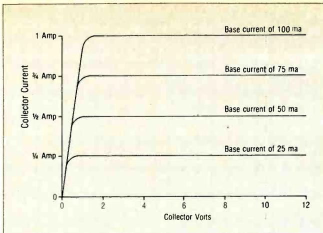
Fig. 1 Collector current versus collector voltage and base current of a silicon transistor
