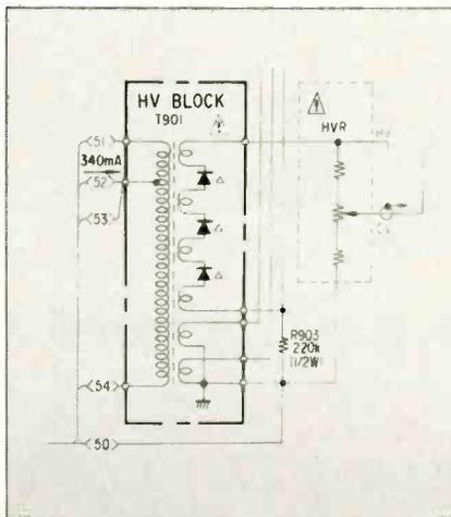
Fig. 6 Flyback transformer from Y-2 chassis.
