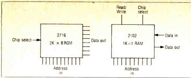
Fig. 3—Simplicity of ROM and Ram chips is suggested by pinouts of these popular devices.
