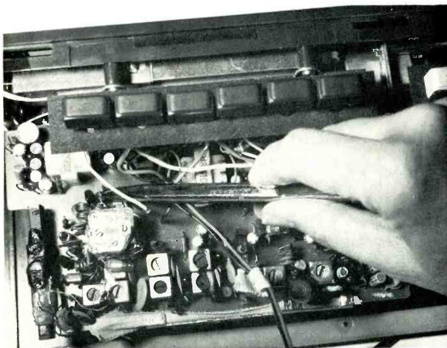
Fig. 10-The FM oscillator transistor may be located next to a couple of air-wound self-supporting coils and close to the variable tuning capacitor.
