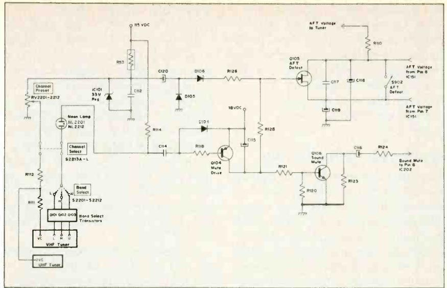
Fig. 4 Simplified schematic of AFC defeat mute circuitry.
