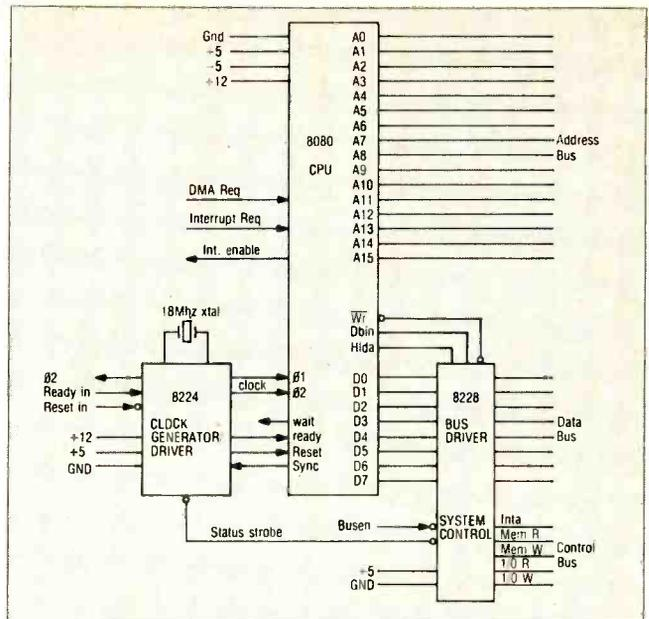
Fig. 5—8080 CPU chip is shown with its support logic. This circuit with added memory and I/O is a complete computer. Parts cost can be as little as \$40.
