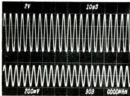
Fig. 6 Top: 200KHz signal at pin 13 of IC1
