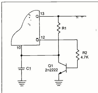
Fig. 3 One-shot (Per figure 2A) modified to allow Q to drop all of the way to zero on low.
