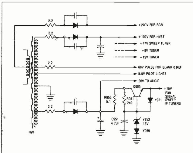
Fig. 2 The EC chassis scan derived supplies.
