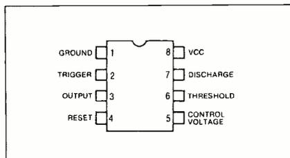
Fig. 4A 555 pinouts and package.
