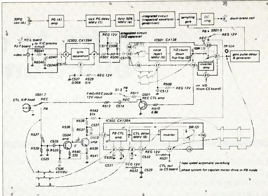
Fig. 18 The vertical sync and CTL (control) signal circuits
