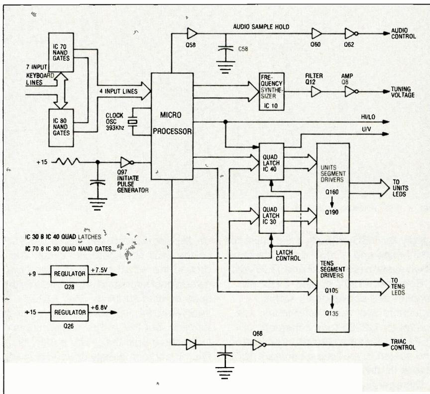
Fig. 7 MP-82 block diagram.
