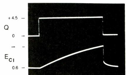
Fig. 2B Output and capacitor waveforms.
