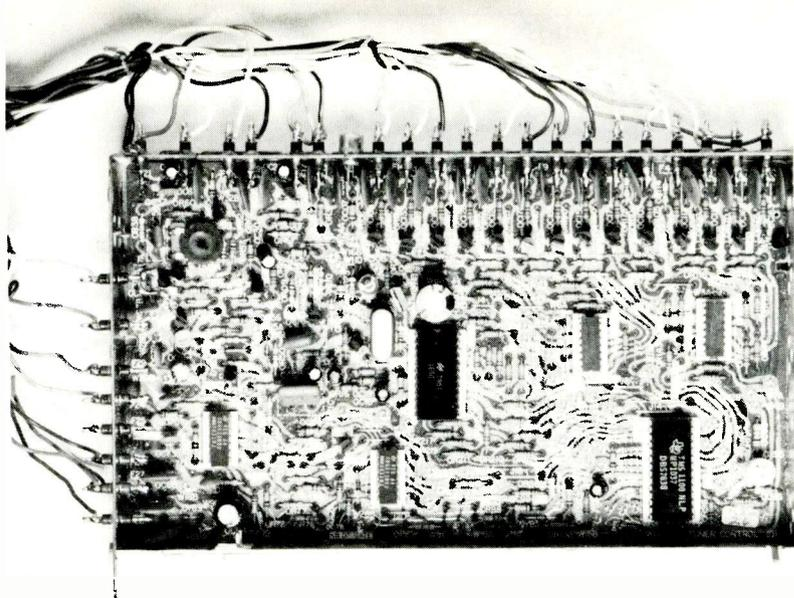
Fig. 6 MP-82 control module.
