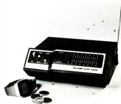
tinuous reception of weather forecasts. As an extra safety feature the monitor is available with an emergency power supply that allows it to keep playing for hours should the power go out. A flashing, red light on the front of the radio lets the user know if the battery inside is weak.
