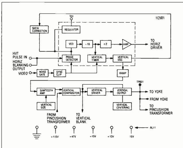
Fig. 5 Sweep module block diagram.
