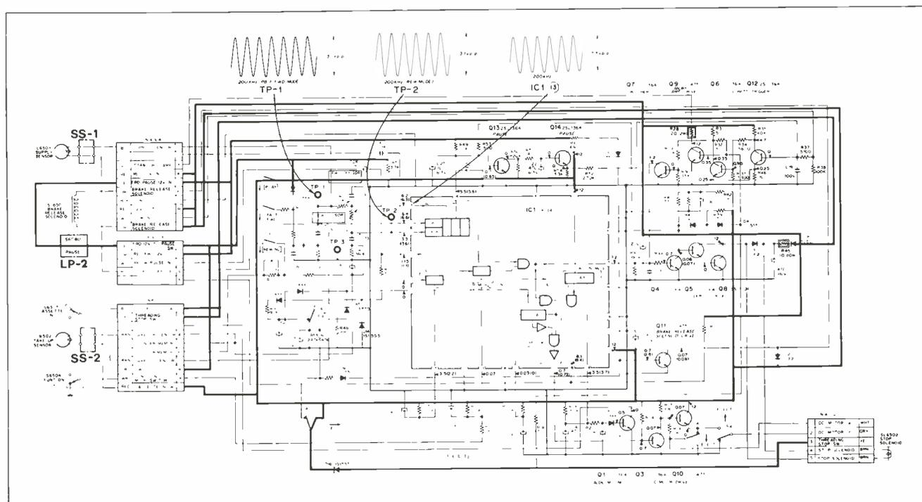
Fig. 5 The SY-2 system circuit diagram
