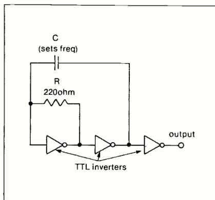
Fig. 5C Another configuration for TTL astables.
