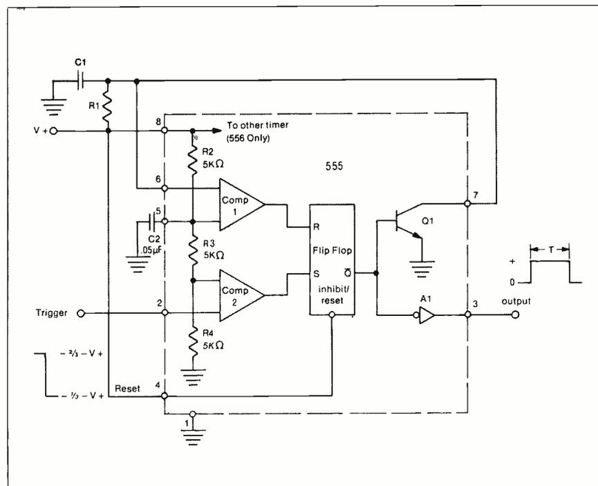
Fig. 4B 555 Connected as a one-shot (internal block diagram).
