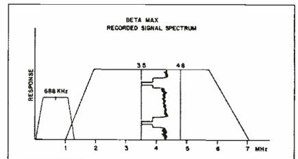
Fig. 2 The Betamax signal spectrum
