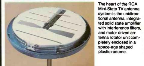
The heart of the RCA Mini-State TV antenna system is the unidirectional antenna, integrated solid state amplifier with interference filters, and motor driven antenna rotator unit completely enclosed in a space-age shaped plastic radome.
