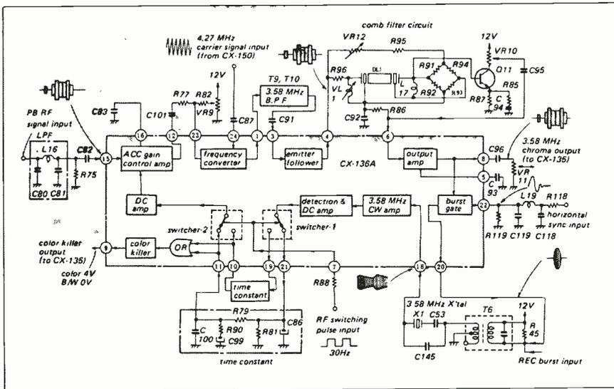
Fig. 8 Block diagram of the chroma playback circuitry
