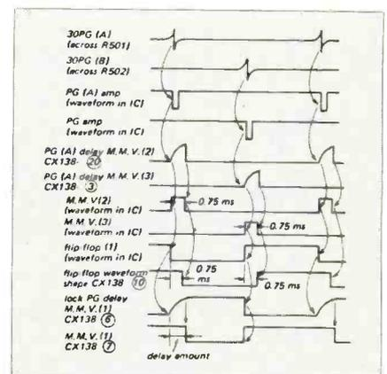
Fig. 16 Timing chart for the 30Hz pulse generator circuit
