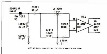
Fig. 6 A new ceramic filter, CF3001, replaces the transformer/capacitor tuned circuit in the CTC97's audio channel.
