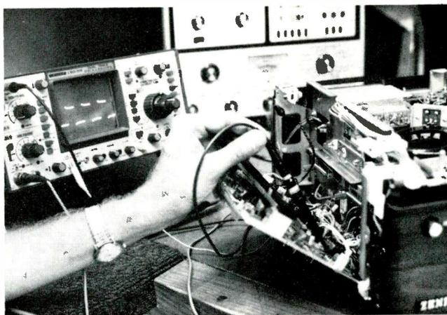
Fig. 4 Slant down boards aid circuit accessibility
