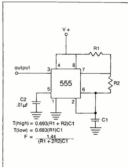
Fig. 5A The 555 used as an astable MV.
