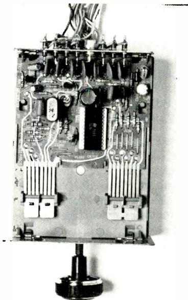
Fig. 9 The switch fingers are operated by the raised sections on the disc.
