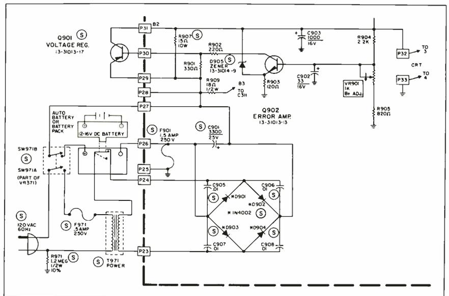
Fig. 5 The power supply schematic for the MT9022W portable from Philco.
