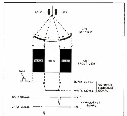
Fig. 7 Sony's newest, Velocity Modulation, controls electron beam scan speed in the new 26-inch CRT for sharper edge enhancement in black to white, and white to black switching.
