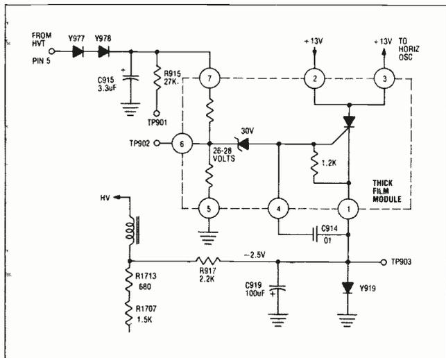
Fig. 4 High voltage shutdown circuit.
