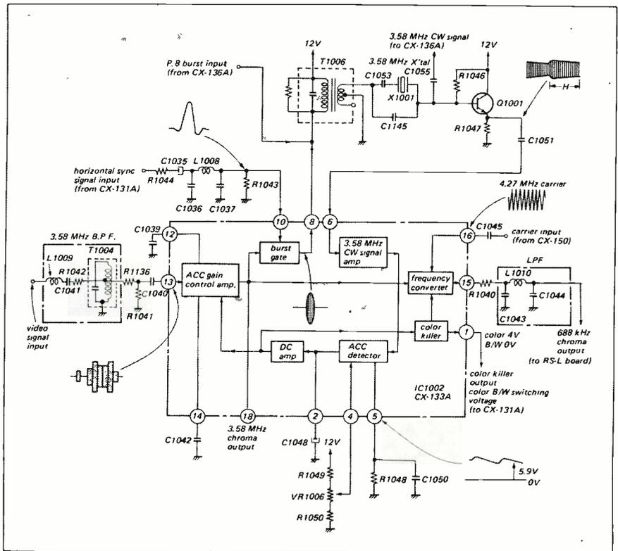
Fig. 7 Block diagram of the chroma playback circuitry
