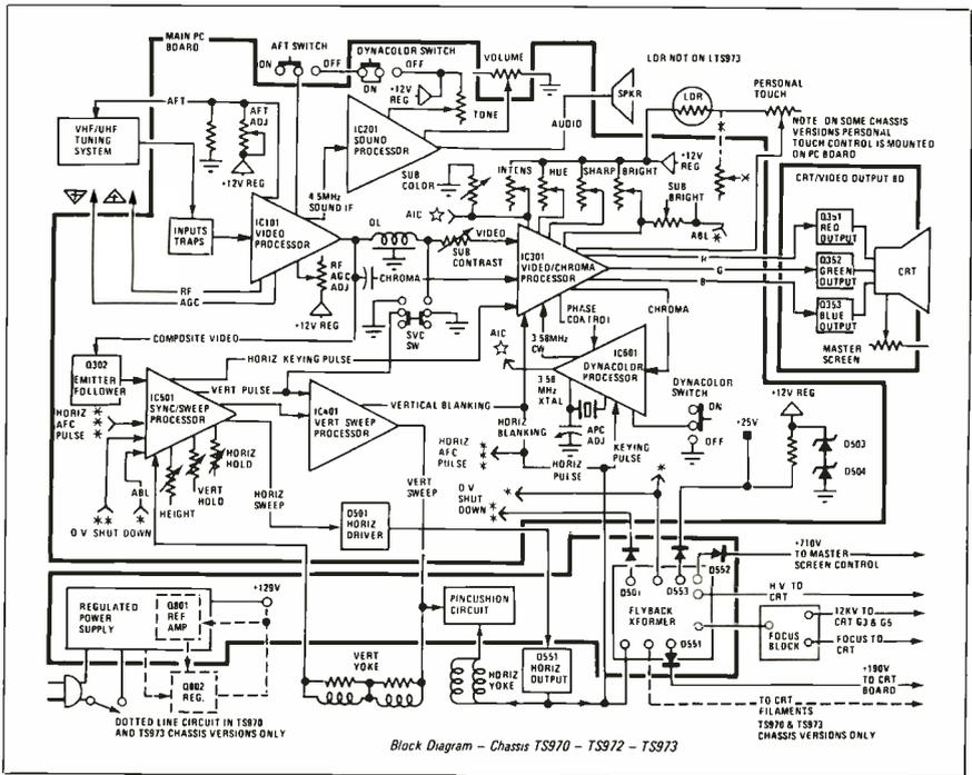
Fig. 4 The basic block layout of Quasar's three newly modified chassis, the TS970, 972, and 973.
