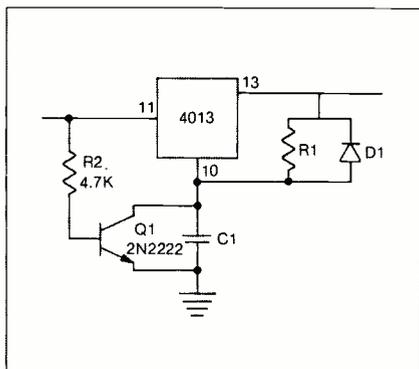
Fig. 6 Figure 2A modified to allow retriggerable operations.
