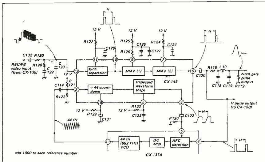
Fig. 10 Block diagram of the sync separator and countdown circuits
