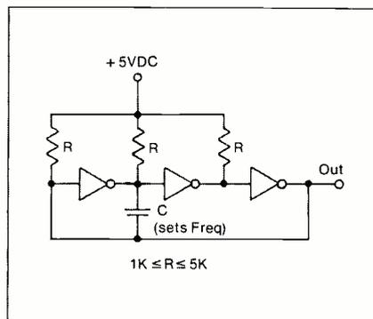
Fig. 5B TTL inverters connected as an astable.
