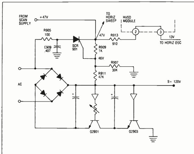
Fig. 3 Power supply start-up circuit.
