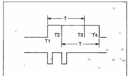
Fig. 1B Retriggerable one-shot operation.
