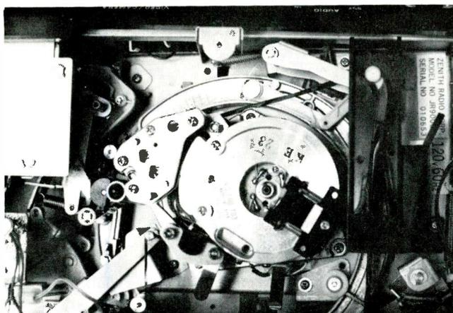
Fig. 3 View of the recording drum and tape heads
