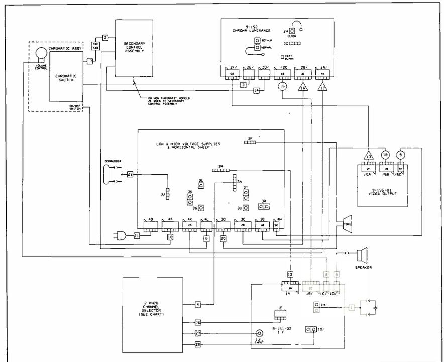
Fig. 3 The modular interconnect diagram for Zenith's L131C and 331 Triple Plus chassis.
