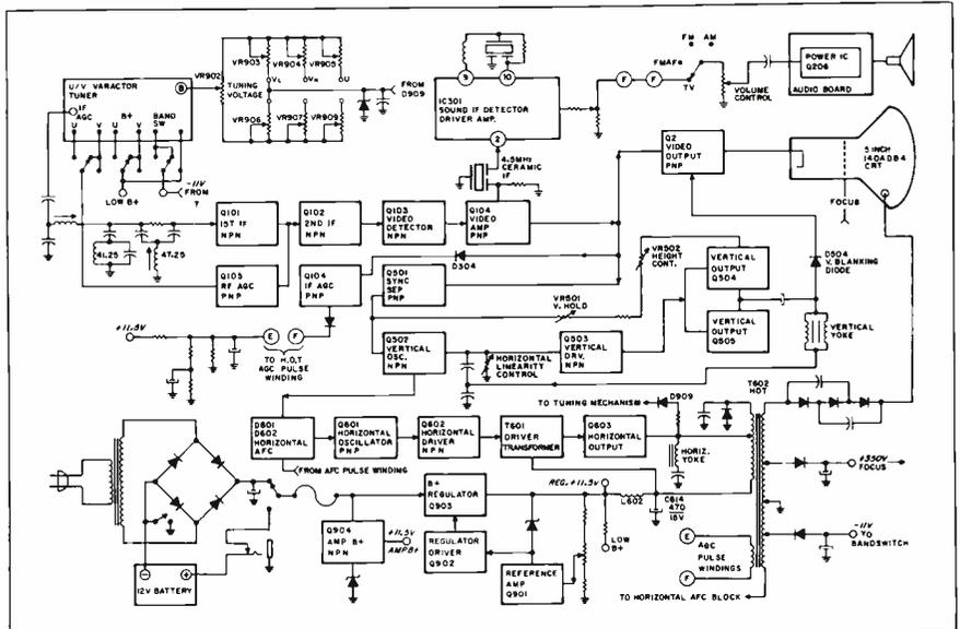
Fig. 2 The M9014GY in block diagram form.
