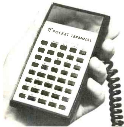
A miniature data terminal of tool-kit size has recently been introduced by G. R. Electronics. The device sends and receives all 128 ASCII codes. The last 30 characters received are held in memory for access through a built-in 16-segment alphanumeric display. Applications could include troubleshooting, debugging, status monitoring, information retrieval and small-scale reprogramming.
