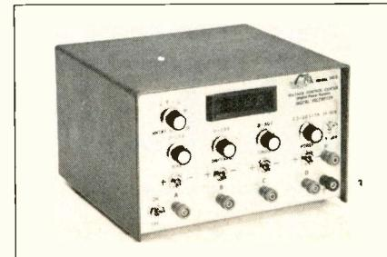
*PTS Electronics* new regulated power supply/DMM includes a 0-30vdc 5 amp supply and three low current supplies, 0-15vdc 50 ma, 0-20vdc at 100ma and 0-30vdc at 200ma. The digital voltmeter can be used independently or to monitor any of the supplies to a reported accuracy of 0.05%. The price is \$269.95 with a one-year limited warranty. **ETD**
