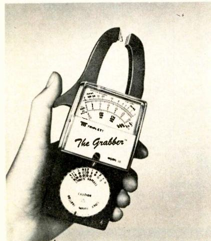
Triplett has just introduced a new clamp-on ammeter/ac voltmeter designated the Model 30. It features a one inch opening and a "Memo-Loc" pointer to permit out of sight measurements. Meter ranges cover 0-300 ac amperes in six ranges, 0-600Vac in three ranges and a ten ohm center scale ohmmeter range with an optional adapter. A leather carrying case is also available. The price is \$65.00.
