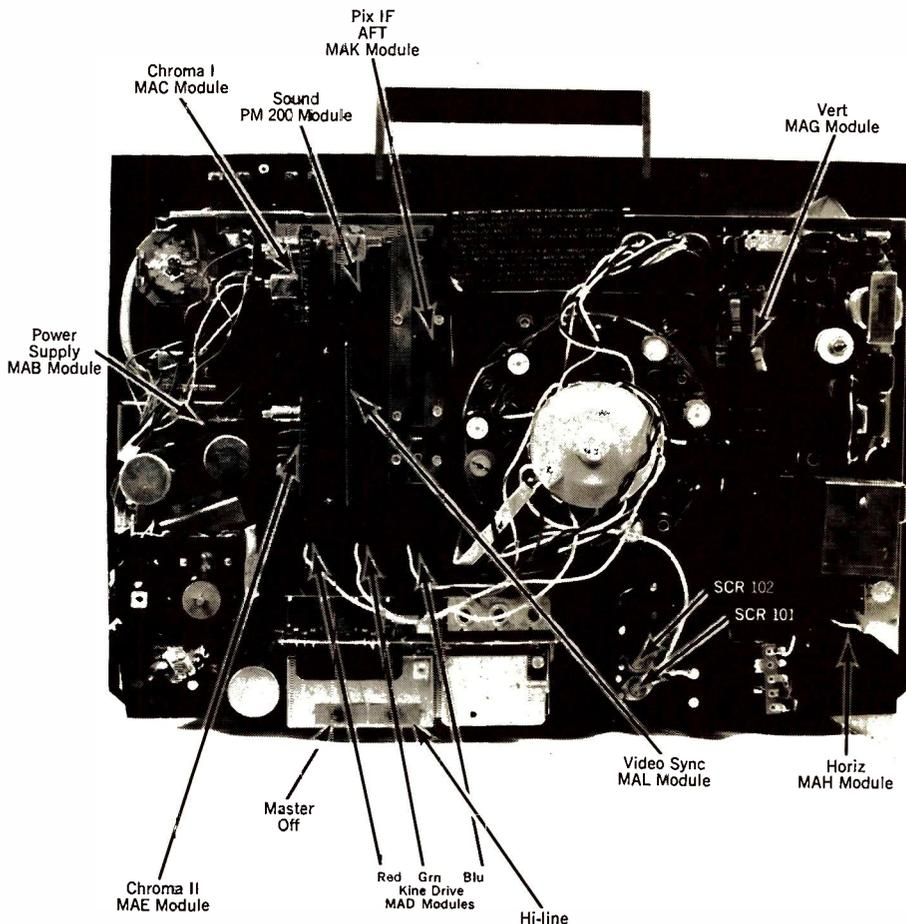
Rear view of the CTC49-color chassis exposing the 11 AccuCircuit modules. With extensive use of modules, the chassis is compact and yet easy to service.
