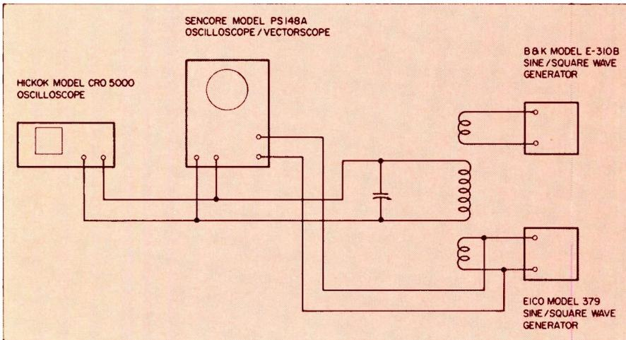
Fig. 1—Schematic of signal resonant circuit used for combining two RF signals.
