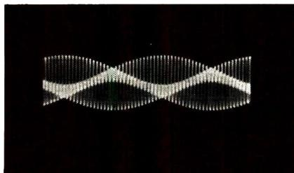
Fig. 25—With a slight reduction in the scope sweep rate it became possible to see that the secondary beat frequency had a wavelength that was 56 times as long as the applied RF signal—indicating that it was a 17.9kHz secondary IF signal.
