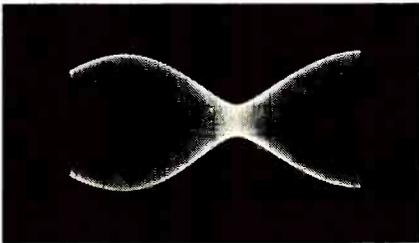
Fig. 7—The 8.0kHz IF signal was more clearly seen by increasing the scope's sweep rate.
