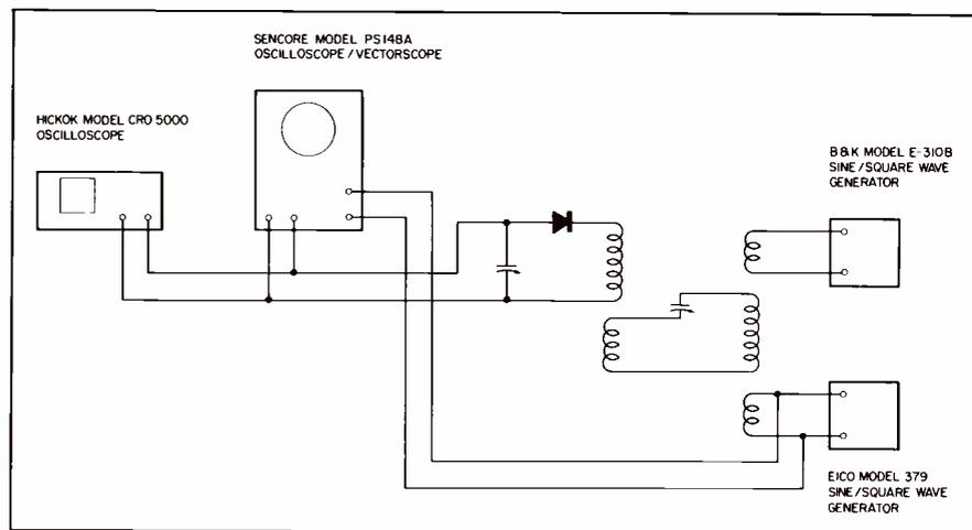
Fig. 21—A second tuned circuit was incorporated in the breadboarded circuit in order that the intermediate frequencies might be more readily observed.
