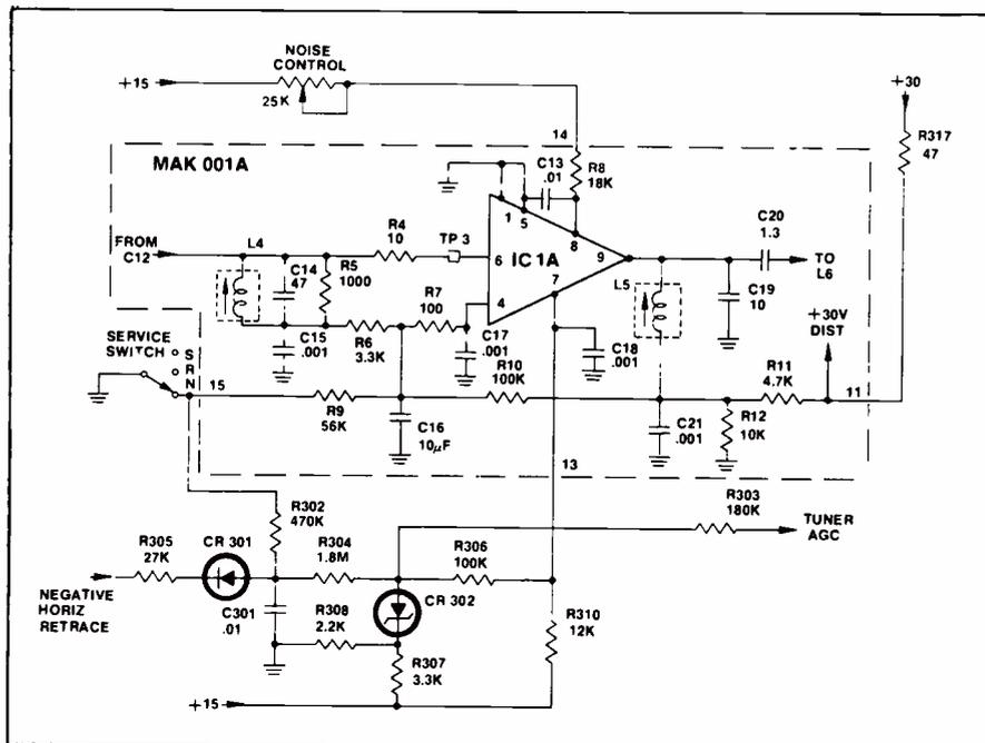
Fig. 1—The First and Second IF Amplifiers and AGC Circuits.
