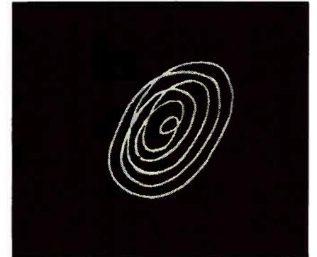
Fig. 12—When the beat frequency is exactly  $\frac{1}{6}$ th the applied RF signal frequency, the phase relationship between the two signals appears as a six-turn spiral.
