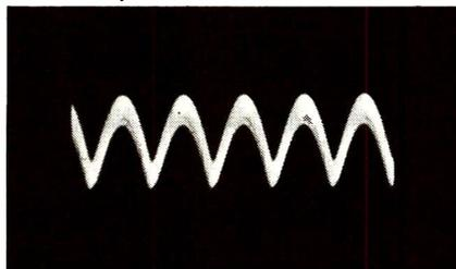
Fig. 27—By transferring the scope leads to the second tuned circuit and increasing the scope's vertical gain, the secondary beat signal became even more apparent.
