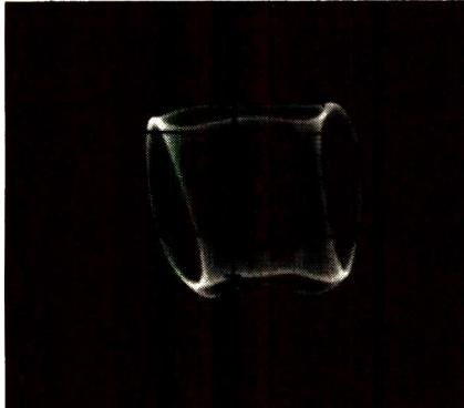
Fig. 23—This phase relationship disappeared when the signal generator was re-tuned to a frequency slightly higher than 2.0MHz.
