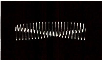
Fig. 24—By combining a 1.0MHz signal with one slightly greater than 2.0MHz, the resulting waveform contained a 1.0MHz beat signal plus some indication of a secondary beat signal.
