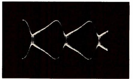
Fig. 5—This beat frequency resulted when a 1.0MHz signal was mixed with another signal having a 1.6kHz higher frequency.
