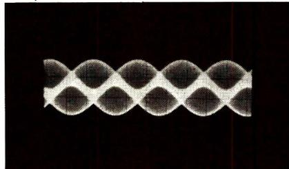
Fig. 26—A further reduction in the scope sweep rate made the secondary beat signal even more apparent.
