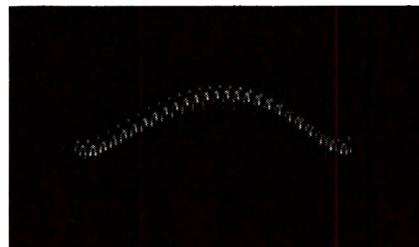
Fig. 28—By increasing the scope sweep rate, it was still possible to see a remnant of the applied RF signals and the primary IF signal riding on the secondary IF signal.
