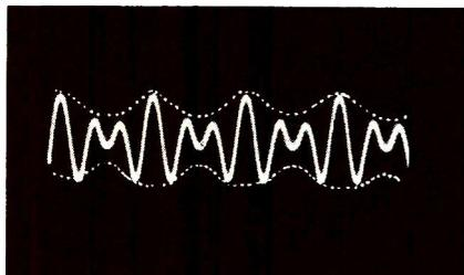
Fig. 15—This beat signal has a frequency  $\frac{1}{3}$ rd that of the applied RF signal.
