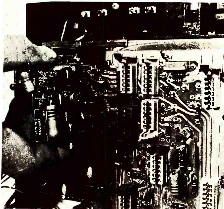
By lifting two spring locks the modules can be easily removed from their edge connectors.
