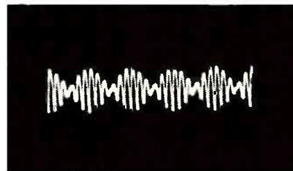
Fig. 10—As the difference between the two applied RF signals becomes greater, the frequency of the resulting beat signal begins to approach the applied RF signal frequency.
