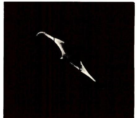
Fig. 4—No phase relationship appeared between the 1.0MHz applied RF signal and the resulting 1.6kHz beat signal.
