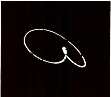
Fig. 18—With the beat frequency being half the applied RF signal frequency, a two-turn spiral was observed.
