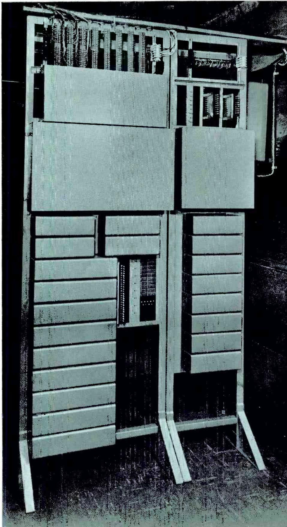
An example of an automatic switchboard which can be expanded with the installation of plug-in modules.
