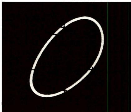
Fig. 2—A circular pattern appeared on the Sencore scope when the two signal generators were both tuned to 1.0MHz.
