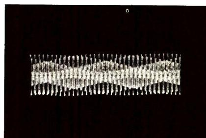
Fig. 20—By reducing the scope sweep rate a secondary IF signal could be observed in addition to the primary IF signal.
