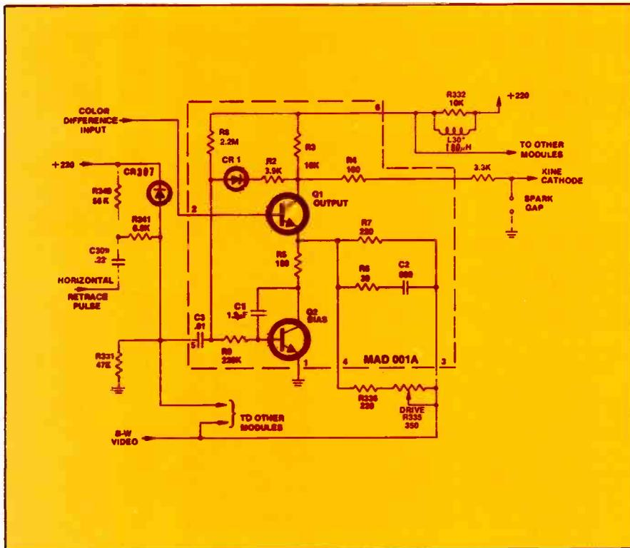
Fig. 3—Schematic of a Module MAD kine driver. The load from the three CRT cathodes is divided equally among three moderately rated drivers instead of one high power device.
