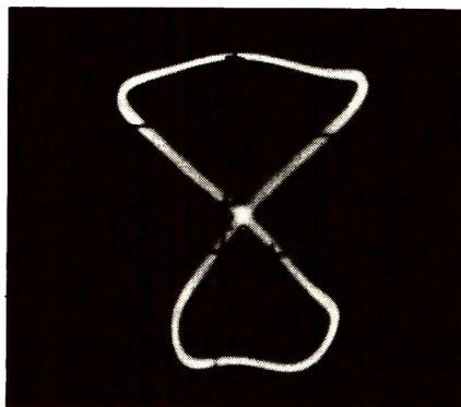
Fig. 22—A figure-eight pattern could be seen on the Sencore scope when the EICO signal generator was tuned to 2.0MHz while the B & K signal generator remained at 1.0MHz.
