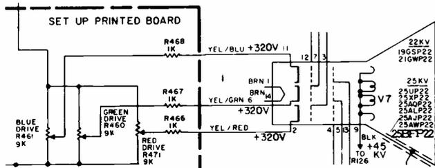
25BFP22. Each control has a value of 9K so that the three controls in parallel provide a 3K load on the video output tube.
