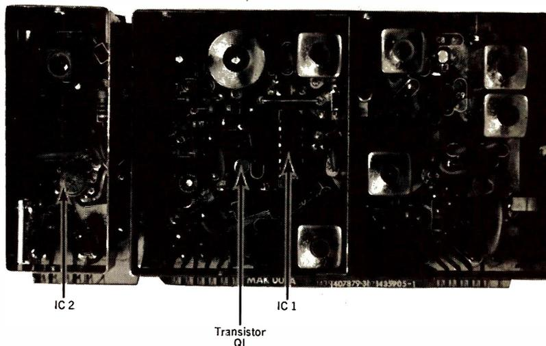
All of the IF amplification and the generation of AGC voltage is accomplished in a single integrated circuit IC1 mounted in the IF Module, MAK.
