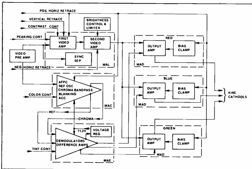
Fig. 2—Functional block diagram of the video system used in the RCA CTC49 color chassis.
