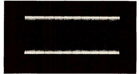
Fig. 3—No beat frequencies were apparent on the Hickok scope when the two signal generators were both tuned to 1.0MHz.
