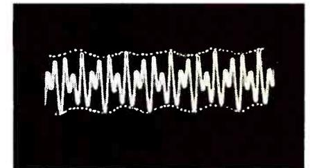
Fig. 13—The wave form that results when the beat frequency is  $\frac{1}{5}$ th the applied RF signal frequency.
