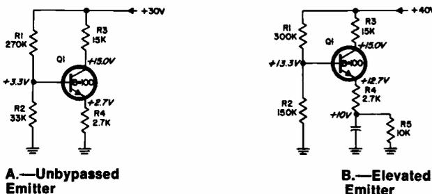
Fig. 1—Common emitter stages.
