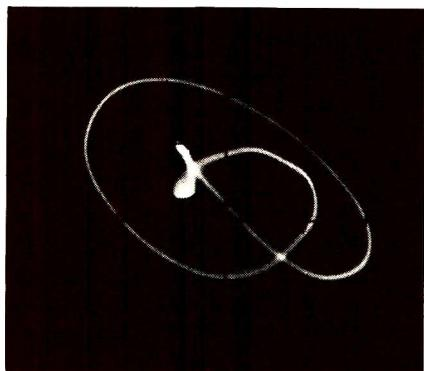
Fig. 16—A little imagination is also required to see the three-turn spiral representing the phase relationship between the applied RF signal and the resulting IF signal.
