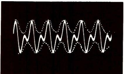
Fig. 17—When one signal generator was operating at 1.5MHz while the other was operating at 1.0MHz, there was a 500kHz resulting beat frequency.
