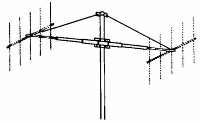
mit them to be extended to optimum spacing. A phasing harness is supplied with the stacking kit. Price \$49.95. Antenna Specialists Co.
