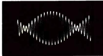
Fig. 9—This IF signal had a wave length 17 times as long as the 1.0MHz applied RF signal, indicating that its frequency was about 63kHz.
