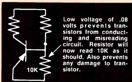
**Here is why you should have both Hi and Lo battery voltages for correct in-circuit resistance measurements in solid state circuits:**
