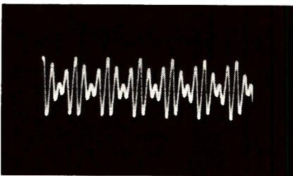
Fig. 19—A waveform that appears when the beat frequency is somewhere between  $\frac{1}{4}$ th and  $\frac{1}{3}$ rd the applied radio frequency.
