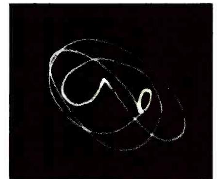
Fig. 14—With a little imagination, the phase relationship between the 1.0MHz applied RF signal and the 200kHz IF signal resembles a five-turn spiral.
