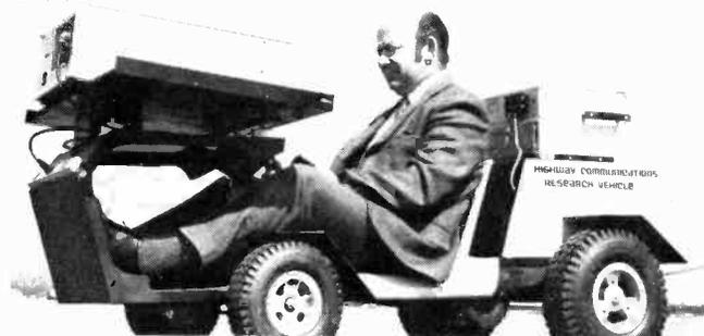
The vehicle measures signal strength and noise levels of several antenna models which are buried in a test roadway. Based on test results, GTE Sylvania's Sociosystems Products Organization will recommend antenna models and related equipment, as well as techniques, for the development of a highway communications system whereby drivers and authorities can exchange messages.
