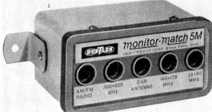
work isolation and impedance matching in conjunction with a regular outside mounted or windshield antenna. It is said to cover the 25 to 50MHz, 140 to 175MHz and 300 to 500MHz bands. Installation requires only that connectors be plugged in. New-Tronics Corp.
