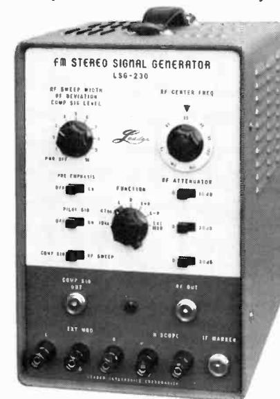
justable frequency range of 75 to 110MHz. Rated separation is over 30dB from 50Hz to 15kHz. The instrument checks separation and balance in FM receivers and tuners and also serves as a sweep-marker for 10.7MHz FM and IF alignments. It
