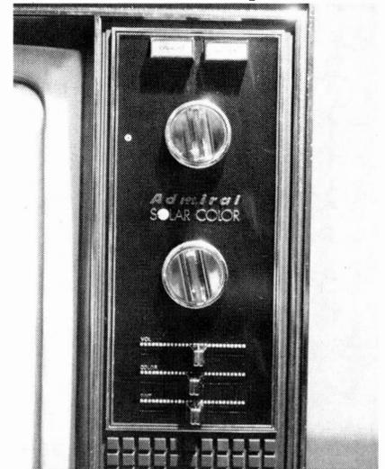
Fig. 2—Front control panel showing the new AUTOMATIC FINE TUNING/COLOR MONITOR control (top right). The VOLUME, TINT and COLOR controls are the slide throttle type.
