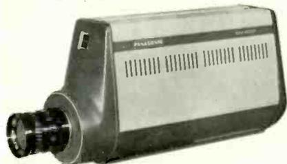
camera has horizontal resolution of more than 550 lines. It uses a  $\frac{2}{3}$ -in. separate mesh vidicon for lower lag, lower video noise levels. Weight is 4.4 lb. The new diecast frame increases reliability and allows easier maintenance. Target voltage is controlled automatically, and once the beam and focus are set for normal operation, simply turning the camera ON and OFF is all that is required for surveillance operations. Matsushita Electric Corp. of America.
