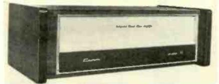
and noise—110dB below 75w output; distortion—IM less than 0.05%, 0.01w to 75w or harmonic less than 0.05% at 75w; separation—better than 90dB, 20Hz to 20kHz; damping—greater than 200, 0Hz to 1kHz; input-impedance—25K adjustable; sensitivity—1.2v for full output. The weight is 22 lb. rack mounted 24 lb, and the dimensions are 17-in. wide by 5¼-in. high by 9-in. deep. Price: \$399.00 without panel, \$429.00 with panel, walnut cabinet \$33.00. Crown International.
