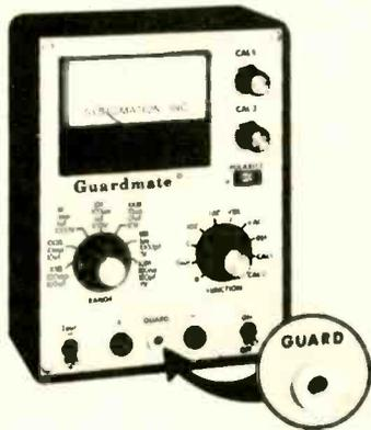
In addition to the conventional red and black test leads, our Portable GUARDMATE has a third lead which offers an exclusive In-Circuit testing capability. The third lead puts a patented Guard Circuit to work, electronically isolating the component under test from all unwanted parallel circuit paths. This is the same Guard Circuit that has been proven by years of operation in Systomation's \$40,000 production PC board testing systems.
