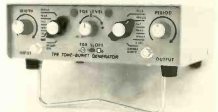
burst width adjusts from 1μsec to 100msec and the period varies from 10μsec to 1 sec. Overshoot and ringing are too low to measure, 170ns rise and fall times, 70ns through-put delay, 5v p-p output, and input and output Z of 10K and 2Ω respectively. Gate switching is phase coherent with the input. This instrument can be used for accurately calibrating audio sys-
