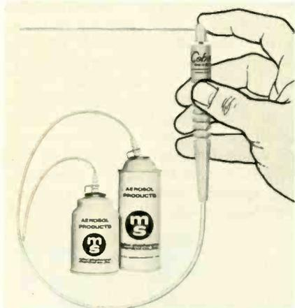
cleansers. The extension nozzle permits application of the cleaning spray to minute, localized areas of printed-circuit boards, instrument circuits, EDP and magnetic recording heads, miniature contacts and other difficult-to-service points. The regular valve is removed from the aerosol can and the extension unit pushed firmly into place. A wire hook is engaged under the rim of the can top to permit spraying and released to relieve pressure during storage. Miller-Stephenson Chemical Co.
