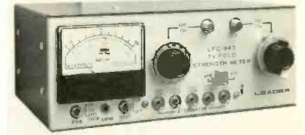
orientation of TV antennas, including those used in MATV and CATV systems. It features a combination dB/mv scale, a precision decade attenuator and a level indicator. It also provides a 75Ω input (VHF), 300Ω (UHF), and "F" connector; and is equipped with an earphone for audible signal checks and noise tracks. It is said to be complete with a sturdy carrying case and a neck strap for a hands-free use. Price is \$375.00. Leader Instruments Corp.
