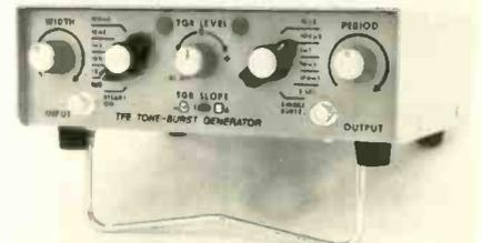
burst width adjusts from 1μsec to 100msec and the period varies from 10μsec to 1 sec. Overshoot and ringing are too low to measure, 170ns rise and fall times, 70ns through-put delay, 5v p-p output, and input and output Z of 10K and 2Ω respectively. Gate switching is phase coherent with the input. This instrument can be used for accurately calibrating audio sys-
