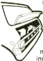
**Engine clear forward.** In Ford's clear-deck design, engine is forward—all the way out of cargo area. Over 8½-ft. clear floor space behind driver's seat... over 10 ft. in the SuperVan. Driver and passenger can easily step from their seats into rear cargo area, exit through side or rear doors.
