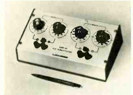
The compact 3.5 lb unit is also said to preclude the necessity for working with unmarked or illegible color coded resistors or capacitors. It measures 3½ in. H by 9½ in. W by 6¾ in. D. Leader Instrument Corp.
