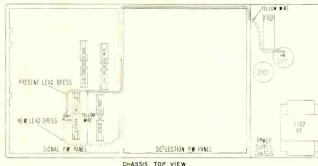
lead dress can be performed without removing the chassis or extending the lead length.
