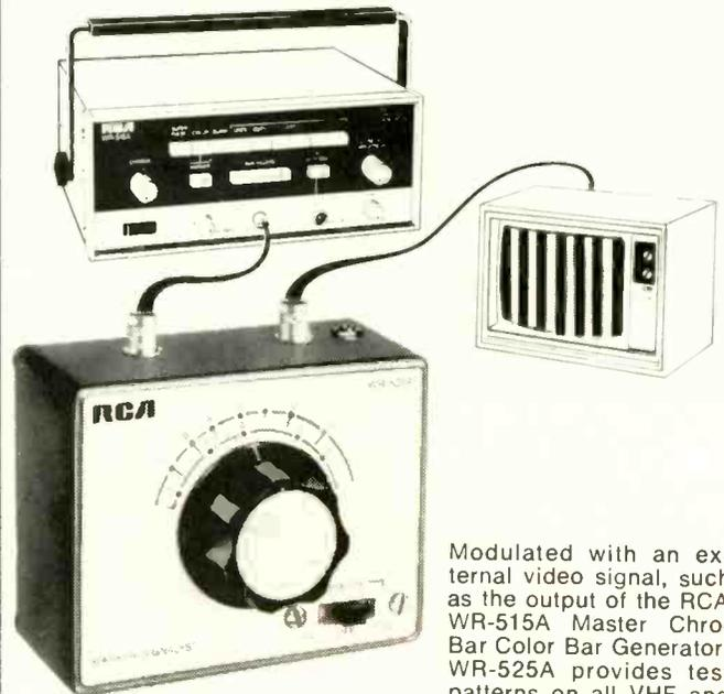
Modulated with an external video signal, such as the output of the RCA WR-515A Master Chro-Bar Color Bar Generator, WR-525A provides test patterns on all VHF and many UHF channels. Use these patterns to check tuner operation and receiver performance. Also use them to check CATV and MATV systems, as well as closed-circuit RF distribution systems and their amplifiers, line-splitters, and other components.
