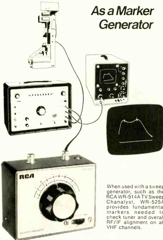
When used with a sweep generator, such as the RCA WR-514A TV Sweep Chanalyst, WR-525A provides fundamental markers needed to check tuner and overall RF/IF alignment on all VHF channels.
