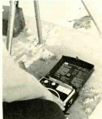
The field strength meter shows 1800 $\mu$ v of signal available on Channel 9 with the antenna at optimum orientation. Even with system losses, Joe Barno calculates that this should be sufficient to give a good picture on the TV set without additional amplification.
