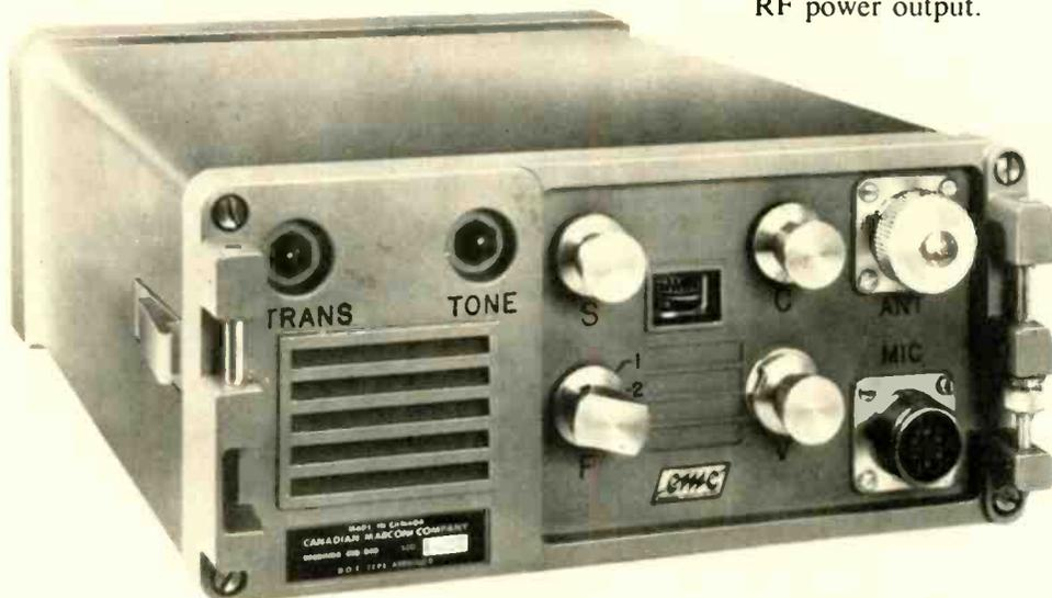
Portable SSB transceiver. Courtesy of Kaar Electronics Corp.
