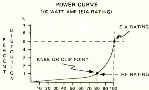
there is always less distortion though the number will always be less than EIA figure.
