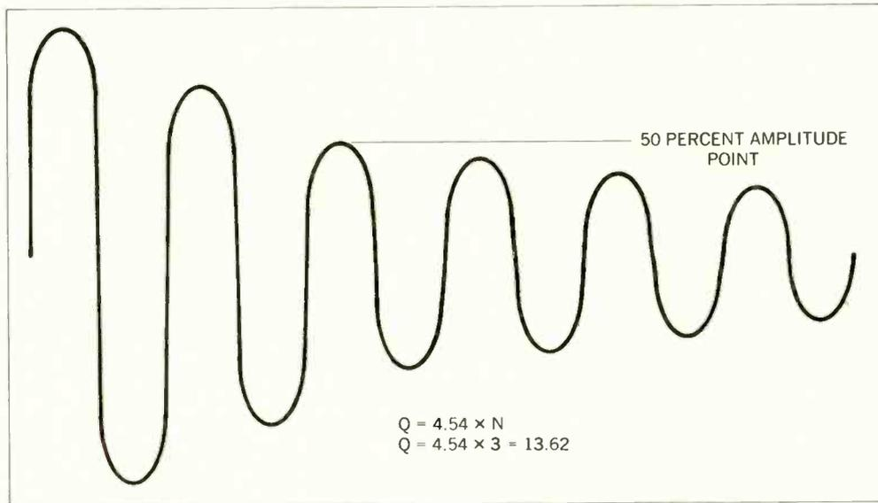
Fig. 13—The wave train may be used to determine the Q of a coil. In the equation, N equals the number of cycles up to the 50 percent point.
