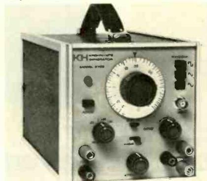
1000:1 tuning range of the dial. Output is said to be controlled by a two-position dB step attenuator and amplitude vernier, providing both a 50 $\Omega$  single ended and a 600 $\Omega$  balanced output. The outputs reportedly provide 15v p-p and 30v p-p respectively, plus a 1v auxiliary output. Krohn-Hite Corp.
