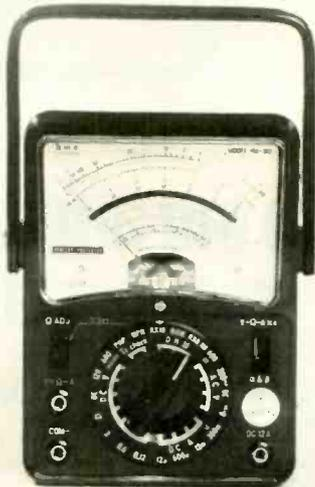
HM-310, VOM/Transistor Tester is a self-contained three-in-one VOM/Transistor/Capacitance Tester featuring 100K per volt, taut-band movement, 3-in. mirrored scale and burn-out protection. Measurement capabilities include: AC and dc volts,
