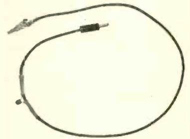
Fig. 4—Ringing lead made up by putting a 15pf capacitor in series with a wire and terminating it with an alligator clip.
