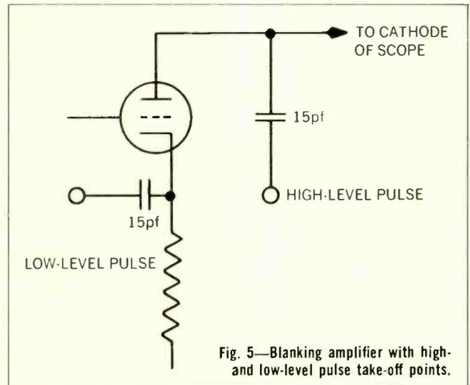
Fig. 5—Blanking amplifier with high- and low-level pulse take-off points.
