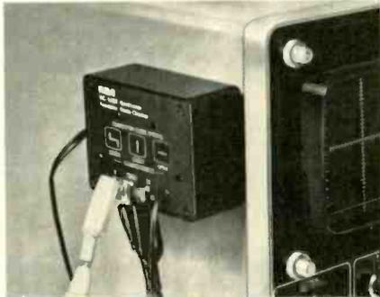
diodes and zener diodes. The unit can be attached to the oscilloscope. RCA Electronic Components.
