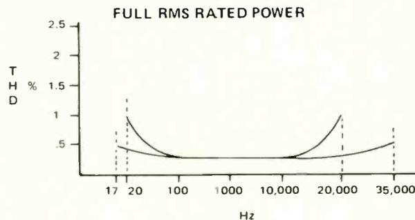
power (RMS) without exceeding its rated distortion set by the IHF standard.
