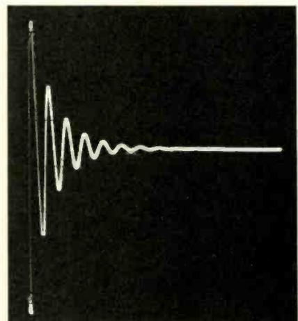
Fig. 12—The wave train of a choke.
