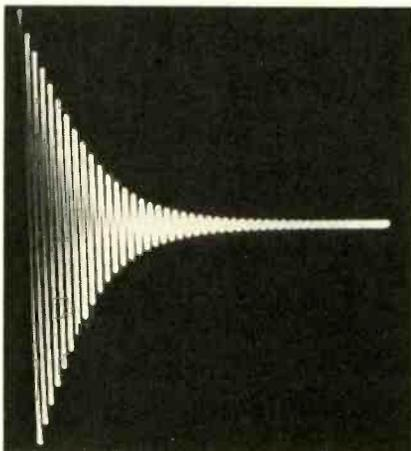
Fig. 7—Wave train of a horizontal-output transformer, using a pulse voltage obtained from the scope.
