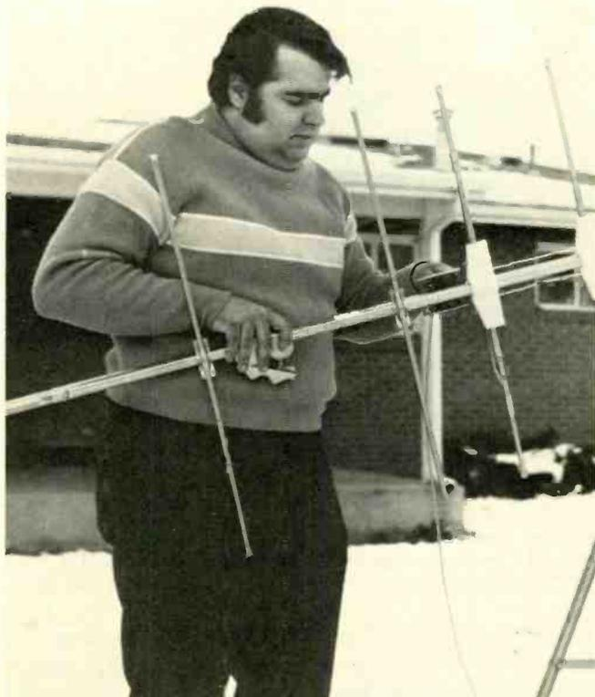
Joe Barno, Denver area MATV contractor, connects a down-lead to the test antenna in preparation for determining the available TV signal at an installation site.
