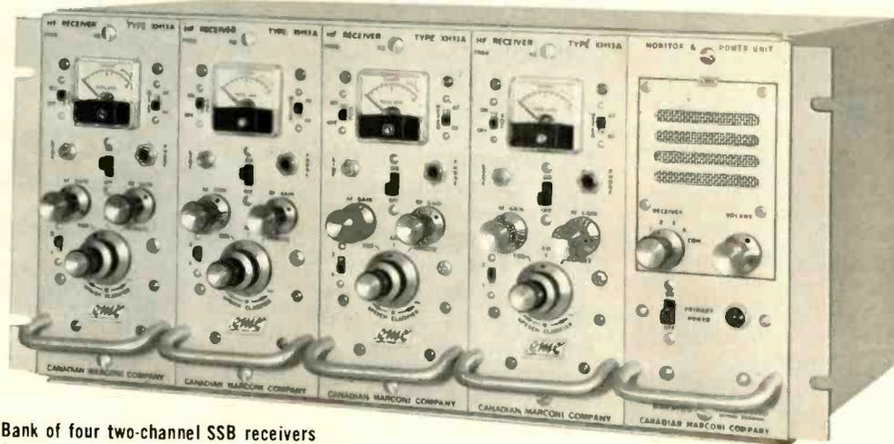
Bank of four two-channel SSB receivers for use on ships or at shore stations. Courtesy of Kaar Electronics Corp.
