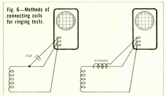
Fig. 6—Methods of connecting coils for ringing tests.
