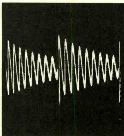
Fig. 8—Wave train of a good horizontal-output transformer using a pencil-type signal injector as a pulse source.
