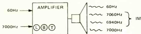
signals—the sum of 60Hz and 7000Hz, and the difference of 7000Hz minus 60Hz. Here again, the lower the percent of IM, the better the amplifier performance.
