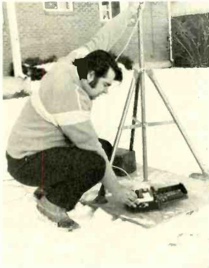
While rotating the mast and antenna with his left hand, Joe Barno watches the field strength meter to find the direction from which maximum signal strength is received.
