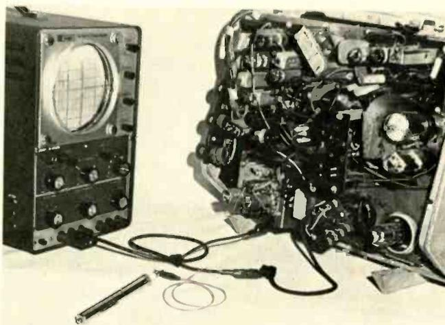
Fig. 1—Ringling test of a horizontal-output transformer using a pencil-type signal injector.
