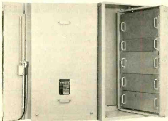
Marine radiotelephone system for larger vessels. Rack contains both VHF/FM and MF-HF/SSB transmitters and receivers. Courtesy of COMCO, a subsidiary of E. F. Johnson Co.
