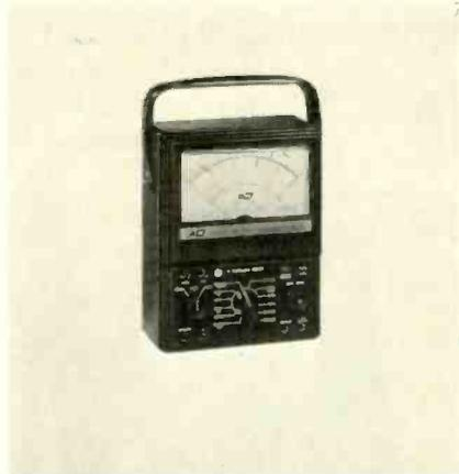
0-250v ac in four ranges. Ohms: R × 1, R × 100, R × 10,000. All ranges except the 10a and 1000v dc ranges are protected by the electronic overload system and the relay contacts are protected by a 3a fuse in the input circuit. The unit measures 5¼ by 7 by 3½ in. deep and weighs 3 lb. Dynascan Corp.
