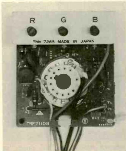
The COLOR SCREEN controls are now mounted on the picture tube socket, reducing the number of wires to the chassis.
