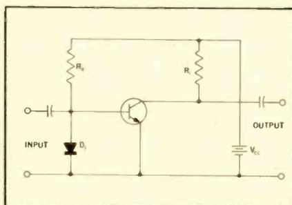
Fig. 11—Diode bias stabilization.
