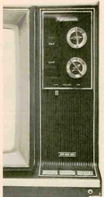
The front control panel has an illuminated channel indicator window for the VHF and 70-channel click-stop UHF tuner. Also included are a lever throttle type VOLUME control and key type switches for Q-Lock, AFT and ON/OFF.
