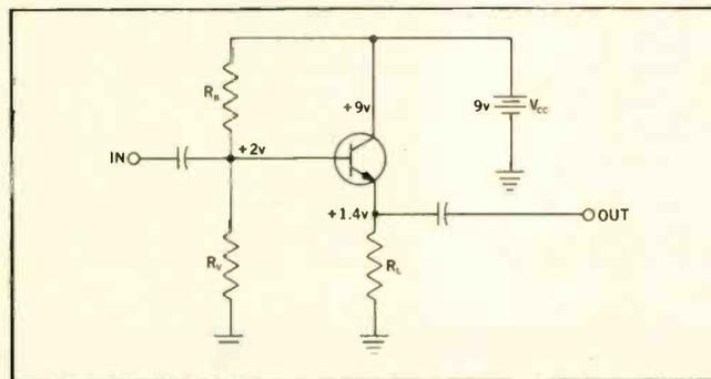
Fig. 18—Common-collector circuit (emitter follower).
