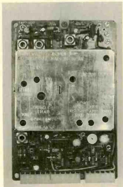
Module Board "A" contains the Video IF and Video Amplifier circuits.
