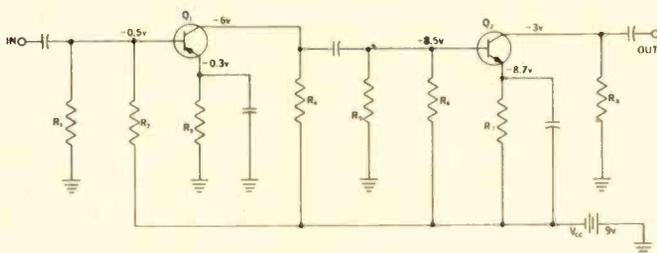
Fig. 14—PNP and NPN transistors in the same circuit.
