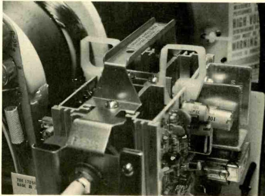
The modules incorporate plastic loop type handles for easy removal and reduce chances of component damage.
