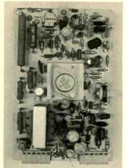
Horizontal oscillator and drive circuits are found on the "H" Board. The horizontal drive transistor, TR504, is located in the center of the module.
