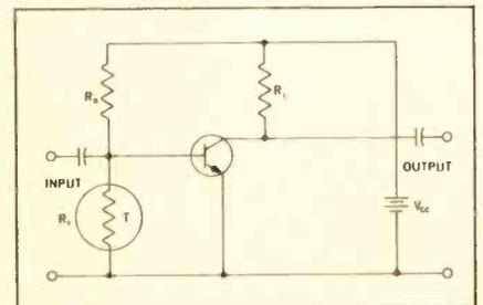
Fig. 9—Thermistor bias stabilization.
