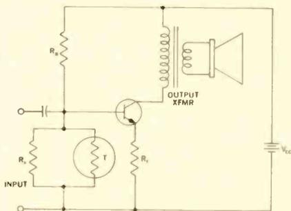
Fig. 10—Bias stabilization of an AF power-output stage.
