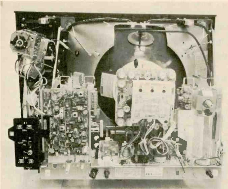
Rear view of the chassis showing service controls and the vertically mounted modules. An additional board is mounted horizontally on the main chassis.
