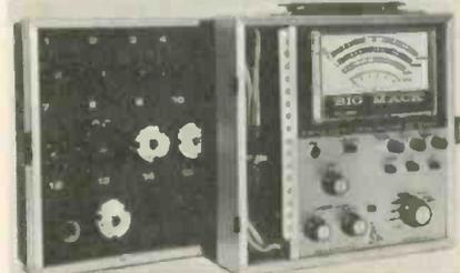
feature is the automatic color tracking test, which enables the user to test single- and tri-gun picture tubes with the same simple push of a button test through a computer type memory bank. All tests are made alike, whether checking B/W tubes or any type of color picture tube. Shorts test have also been moved to the meter, rather than using neon lights. Sencore Inc.
