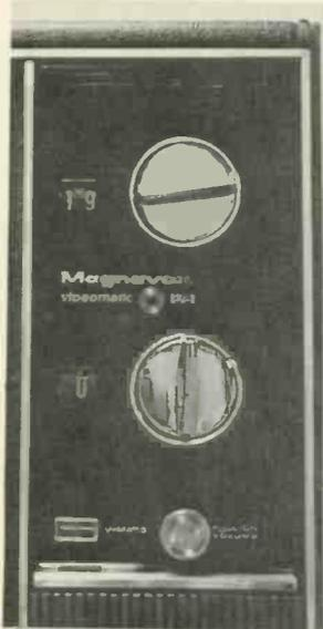
The front control panel has a clean uncluttered appearance and the channel number indicators are of the lighted window type. Also shown is the Videomatic pushbutton to activate the preset controls.
