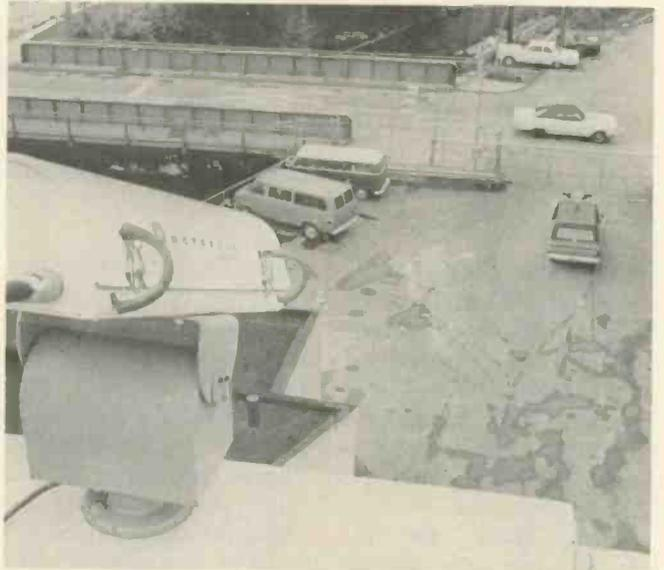
Motorola S-1140B CCTV camera mounted on roof of plant views activity on ground below. Four more cameras, mounted in strategic locations, give monitoring officer view of all that goes on over approximately 95 percent of company facility.
