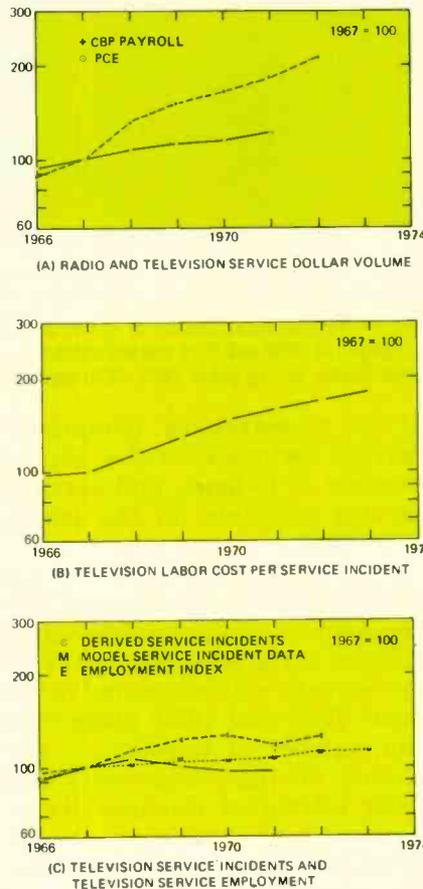
Fig. 6—Annual plots of A) TV and radio service dollar volume, B) TV labor cost per service incident and C) comparisons of service incidents and TV technician employment, for the years 1966-1972, indexed to 1967. In A) the data for the curve labeled "CBP" is from County Business Pattern volumes and the data for the curve labeled "PCE" is from Personal Consumption Expenditure figures.
