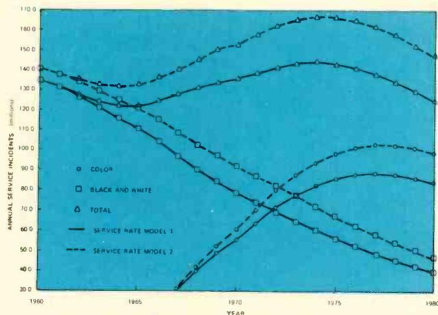
Fig. 7—Annual levels of service incidents generated by color and b/w TV receivers during the period 1960-1980.
