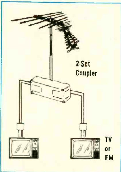
Fig. 10-An example of a passive two-set coupler, designed to serve two TV sets from single antenna.
