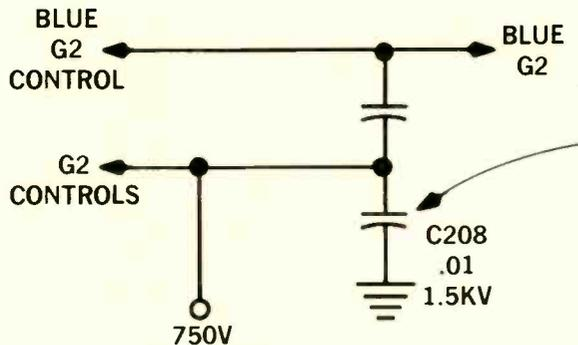
**CAUSE:** Leaky C208. About 5 megohms of leakage measured across C208.
