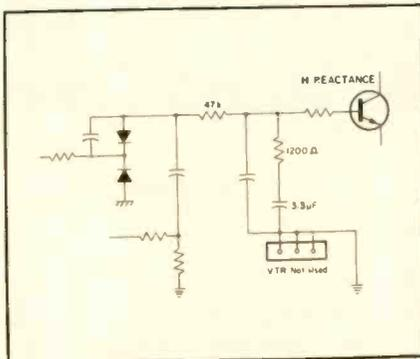
Fig. 8—The three-pin socket labeled "VTR Not Used" in this simplified schematic of the horizontal AFC system of a late-model Sears color chassis seems to be indicative of this and other TV manufacturers' increasing awareness and response to the need for quicker-responding horizontal AFC systems.
