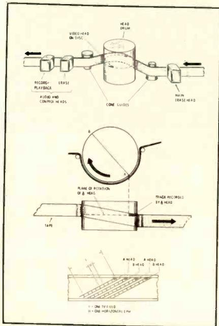
Fig. 1—The tape scan action of a typical helical videotape player/recorder equipped with two heads. As the tape is pulled across the head drum by the capstan, the two rotating heads inside the drum swipe across the tape in a slanted (helical) path. One TV field (262-½ horizontal lines) is recorded on (or played back from) the tape as each head swipes across the tape. (Courtesy of Howard W. Sams Co.)
