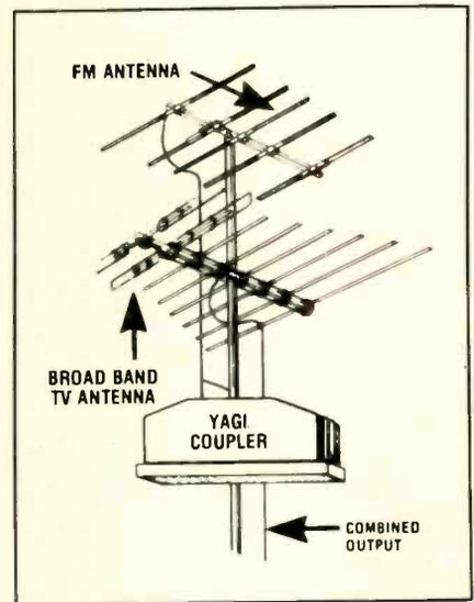
Fig. 3—An example of how a Yagi coupler is used to combine FM antenna with a broad-band TV antenna.
