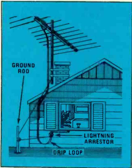
Fig. 6-Lightning protection as provided by lightning arrester, ground wire and ground rod for twinlead transmission line.
