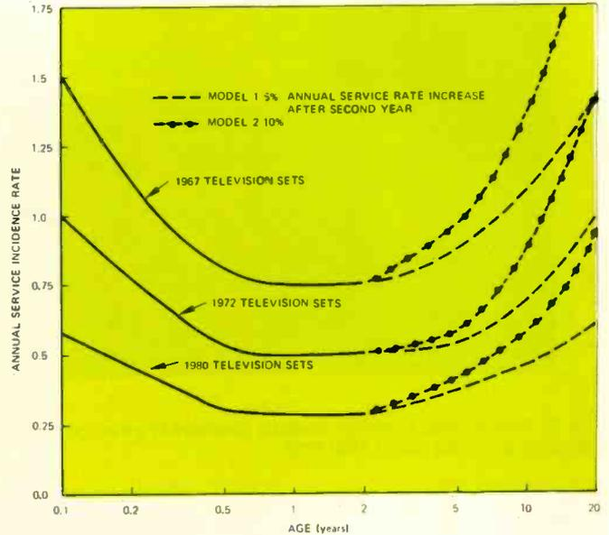
Fig. 5—Models of annual service-incidence rates of 1967, 1972 and 1980 model-year b/w TV receivers.
