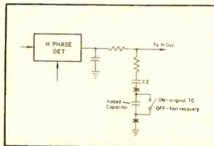
Fig. 6—Connecting additional capacitor in series with C2 reduces total capacitance, thereby speeding up AFC response time.
