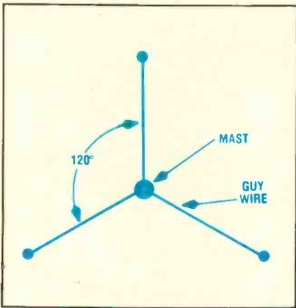
Fig. 5-The method of spacing three guy wires around an antenna mast. Wires should be spaced equally about 120 degrees apart.
