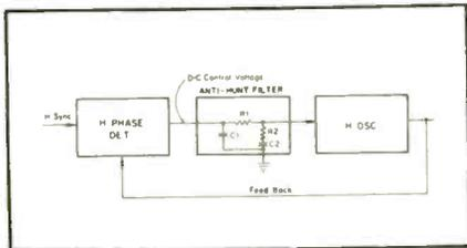
Fig. 4—Diagram of typical anti-hunt filter in a horizontal AFC system. Principal function of filter is to slow down changes in AFC control voltage so that horizontal sync is not affected by random noise impulses.
