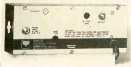
TV camera or other source, monochrome or color-TV, can be applied to an existing MATV system or to a single TV receiver or any unused VHF TV channel. Price is \$99 with LC control, or \$136 with crystal control.
