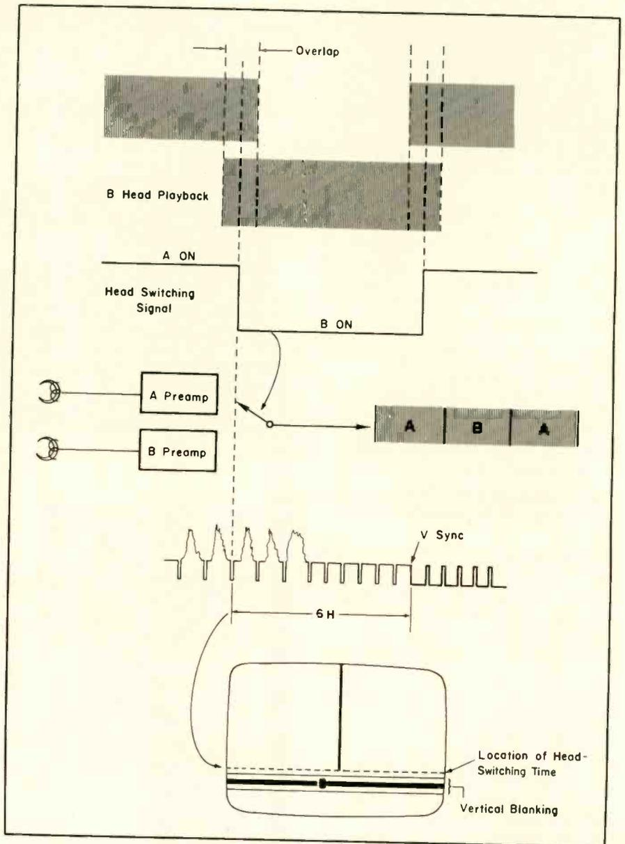
Fig. 2—Illustration of head switching in a two-head helical videotape unit.
