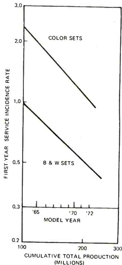
Fig. 2—First-year service-incidence rates of televisions introduced into use during model years 1965 through 1972, plotted as a function of total cumulative production.
