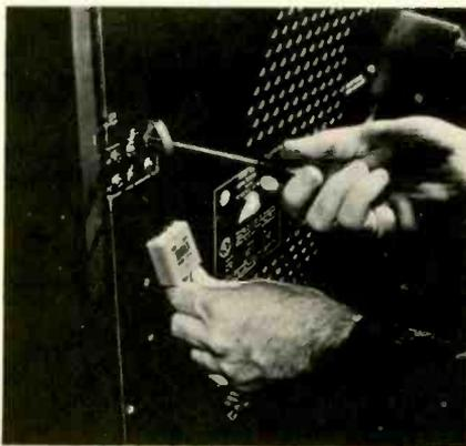
Fig. 8-A combination matching transformer/U-V signal splitter mounted at back of TV set.
