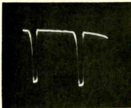
Fig. 3—Clipped horizontal sync waveform.
