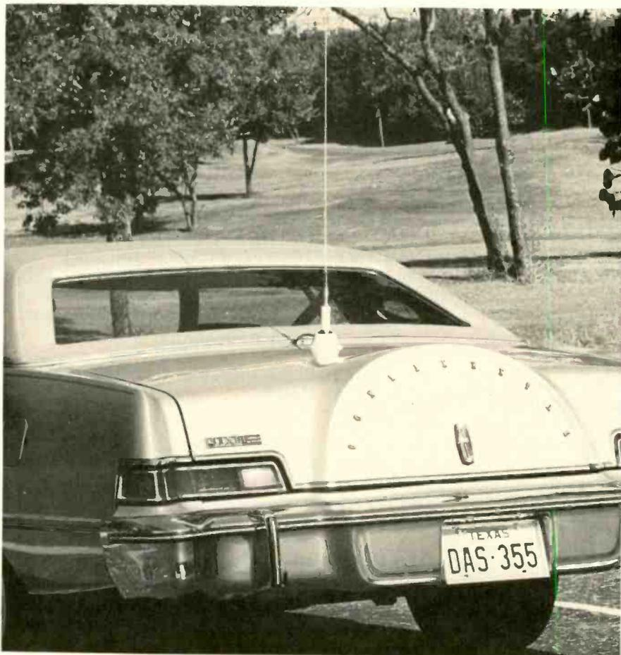
Fig. 6—This whip antenna from Breaker has a magnetic base encapsulated in ABS to prevent surface scratching. It is quickly removed for theft prevention.
