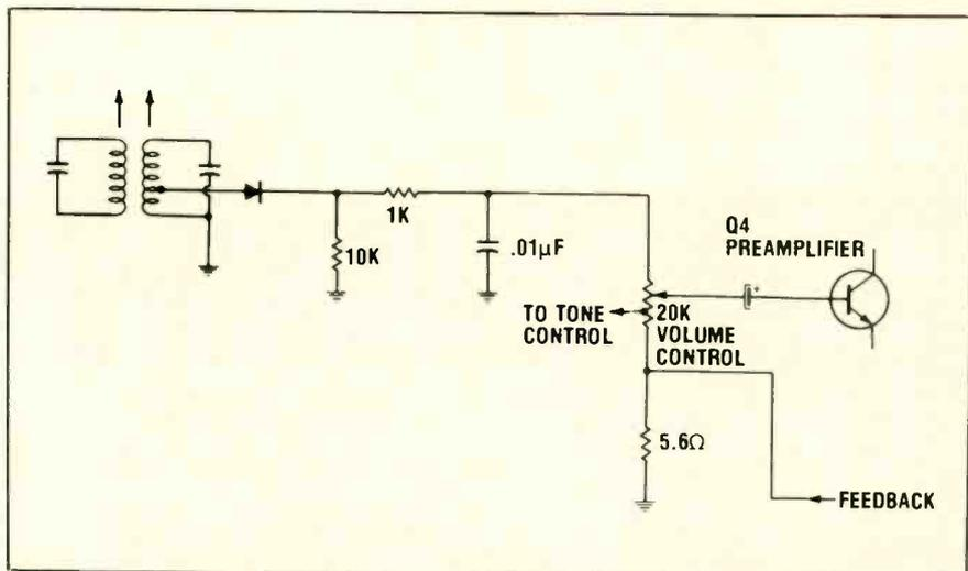
Fig. 1—A shorted AM detector diode does not necessarily mean no audio output. Strong signals can feed through shorted detector, be rectified by the base-emitter "diode" of Q4 and produce weak, distorted audio output.
