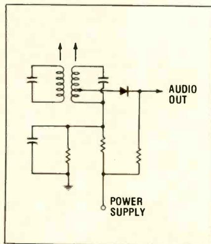
Fig. 2—A defect which increases the reverse bias across the normally-reverse-biased audio detector shown here can cause weak, distorted audio.
