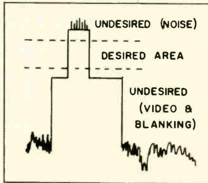
Fig. 1—Horizontal blanking and sync pulse showing portions "clipped out" by sync clipper action.
