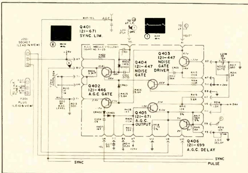
Fig. 2—Typical all-solid state AGC and sync module.
