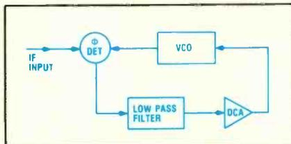
Fig. 9—Block diagram of a typical phase locked loop (PLL) FM detector IC.
