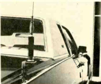
Figs. 10 & 11—Two somewhat similar antenna-concealment devices for CB that allow the user to lock the antenna inside the car trunk when not in use. Fig. 10 is the Stowit antenna from Holly Enterprises, and Fig. 11 is the Tuk-a-Way antenna from Deep South Marketing.
