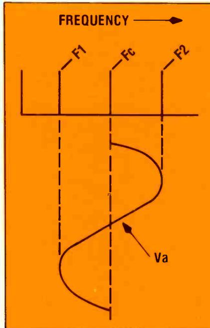
Fig. 1—The frequency of the FM carrier varies from its rest, or unmodulated, value to a maximum at  $F_2$  and a minimum at  $F_1$  as the audio signal,  $V_a$ , varies through positive and negative excursions.
