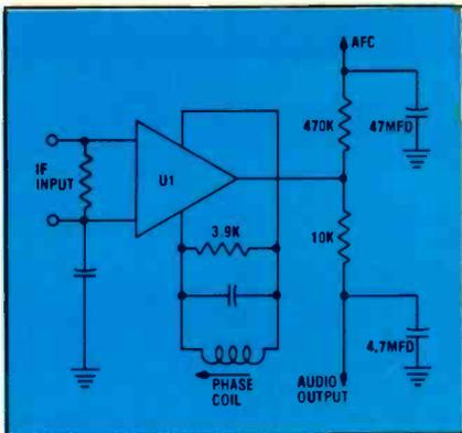
Fig. 8—Partial schematic of an FM detector using the ICQD. This circuit is identified as a quadrature detector by the presence of the "phase coil" and not by the fact that an IC is used.
