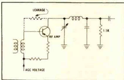
Fig. 4—Collector-to-base leakage in the RF amplifier, illustrated here, also can cause distortion which varies with received signal strength.
