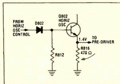
**CAUSE:** Slow stabilization of horizontal oscillator as result of increase in the value of resistor R816 (470 ohm, 10%, ½ watt). Replace R816 with Admiral Part No. 60A105-471 (470 ohm, 5%, ½ watt).
