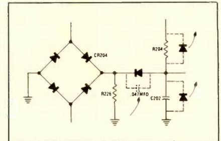
**CAUSE:** Presence of the AC power line of even harmonics (120 Hz and 240Hz) of the 60-Hz power line frequency. The following modifications of the remote system clock circuit will restore normal operation in the presence of such AC power line interference:
