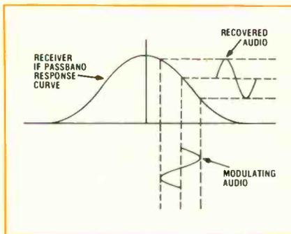
Fig. 2—Slope detection is an FM demodulation method in which the receiver is tuned so that the carrier,  $F_c$ , is centered on the descending portion of the IF selectivity curve.
