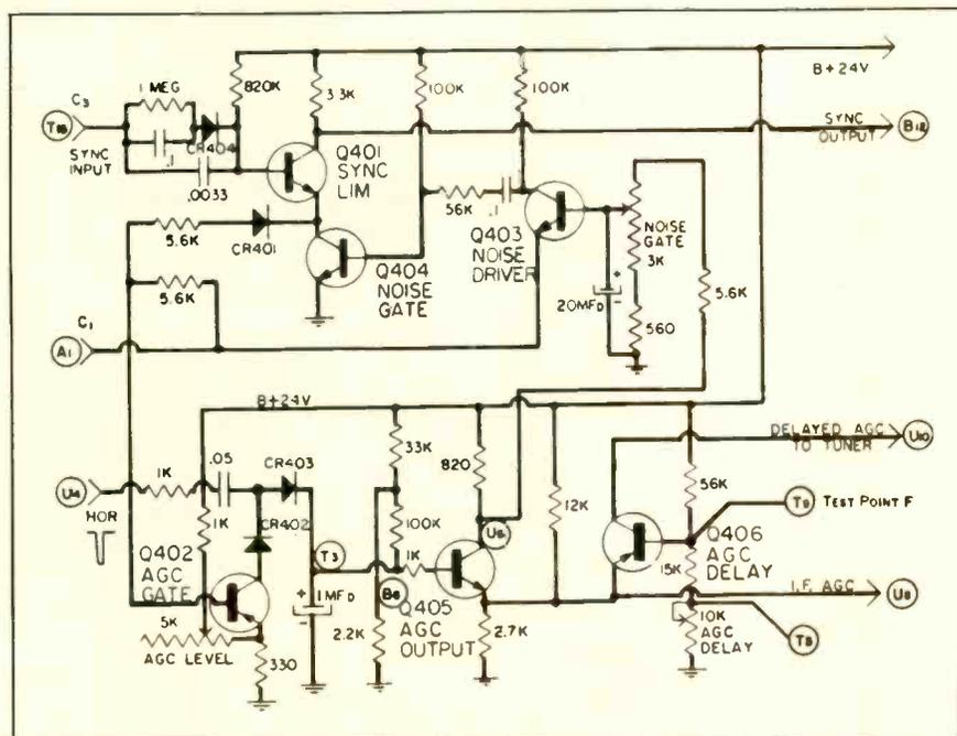
Fig. 4—Simplified version of AGC and sync module circuits shown previously in Fig. 2.
