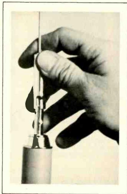
Fig. 8—This Model M-450 from Antenna Specialists allows only the whip to be removed from a base-loaded antenna. A downward push and twist on the knurled adapter releases the whip.
