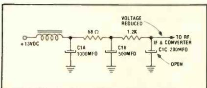
Fig. 6—Open C1C in the AM car radio power supply shown here or a "partial short" in the Zener B+ regulator of an FM car radio also can cause distorted audio.
