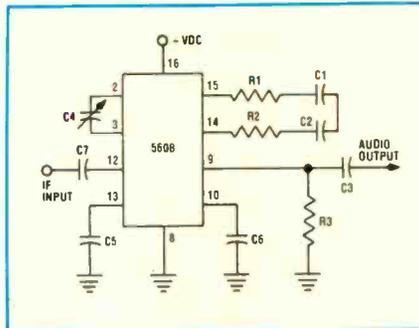
Fig. 10—Circuit of an FM detector equipped with the Signetics 5608 IC PLL.
