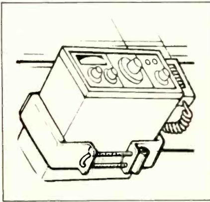
Fig. 3—A new locking CB radio mount for theft prevention. Mounting bolts are concealed by metal cover that is padlocked.
