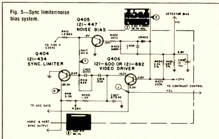
Fig. 5—Sync limiter/noise bias system.
