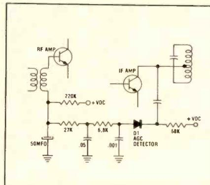
Fig. 3—Typical car radio automatic gain control (AGC) system. Defects in this system can cause audio distortion whose degree varies with received signal strength.
