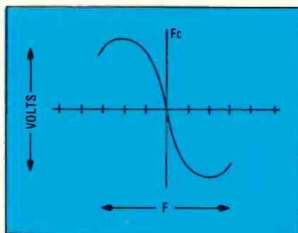
Fig. 5—Frequency response of the typical FM discriminator.
