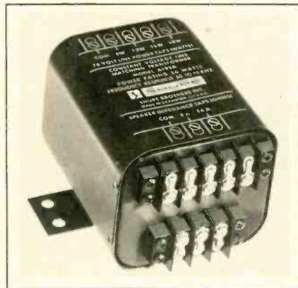
with speaker impedance taps to accommodate various speaker loads. Four power taps (50, 25, 12 and 6 watts) are provided on the model A102-A for connection to the 70-volt speaker line from the power amplifier. It features a weatherproof steel case, an encapsulated autotransformer sealed from moisture, and an integral mounting strap. User net price is \$31.50.
