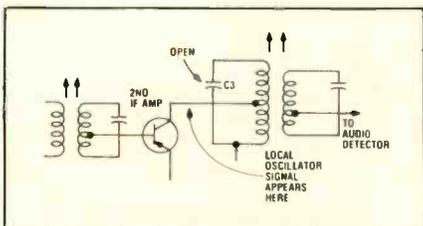
Fig. 5—Defects in IF amplifier section of a car radio can cause non-audible oscillations which, in turn, causes distortion of the audio output. Or if the resonant frequency of the 2nd IF transformer is changed by a defect, the local oscillator signal might feed right through to the collector of the IF amplifier transistor.
