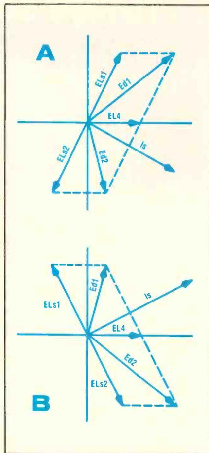
Fig. 4—A) Voltage relationships in the discriminator as the carrier approaches F2. B) Voltage relationships in the discriminator as the carrier approaches F1.
