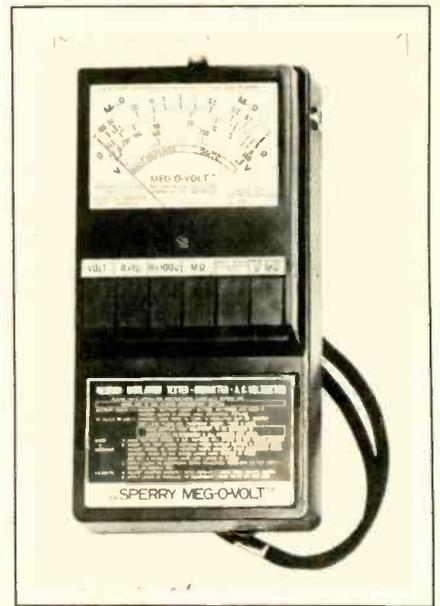
mid-scale, and the 520, which has a 1,000 megohm scale with a 20 megohm mid-scale. Both models have Rx1 and Rx100 resistance scales, as well as a 0-300 AC voltage scale. They feature keyboard push-button controls, threaded test leads, and a shock-resistant plastic housing. Powered by 8 AA batteries, the meter is portable. It develops a 500 VDC test voltage for insulation testing.
