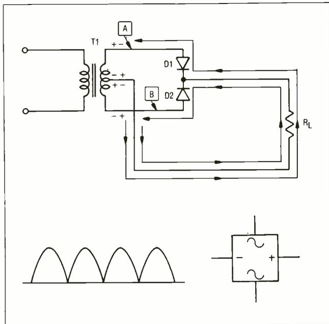
Fig. 4 A) Full-wave bridge rectifier, B) output waveform, C) prepackaged bridge rectifier.
