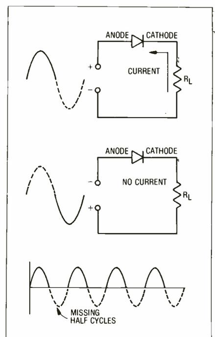
Fig. 2 Half-wave rectifier A) On positive half of input cycle, B) on negative half of input cycle, C) output waveform across  $R_L$ .
