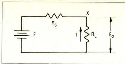
Fig. 6 Equivalent circuit of any power supply
