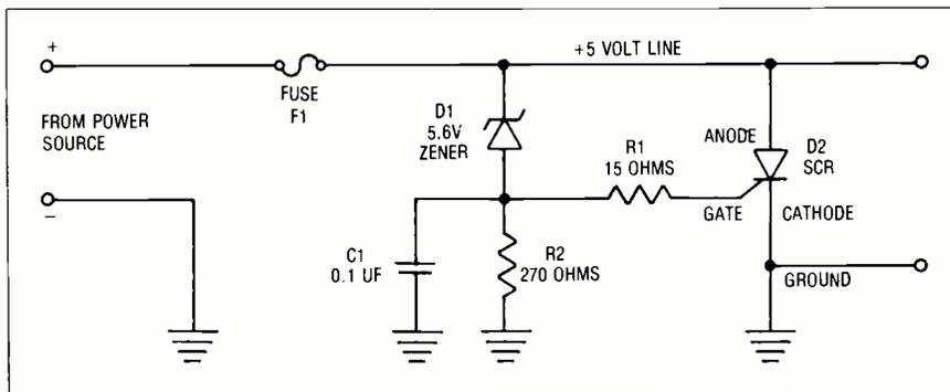
Fig. 13 SCR Crowbar overvoltage protector
