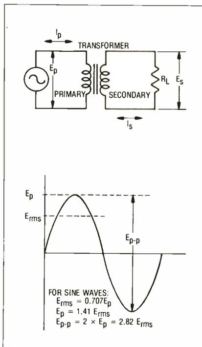
Fig. 1 A) Transformer circuit
