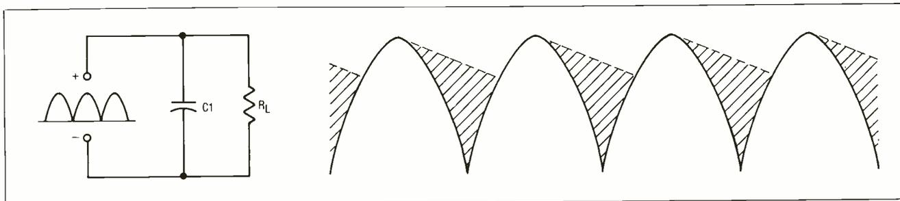
Fig. 5 A) Simplest form of power supply filter B) Solid lines show output waveform without capacitor C1, dotted lines show waveform with C1 connected. Shaded area represents energy dumped back into the circuit that had been stored in C1.
