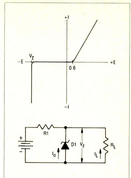
Fig. 8 A) Zener diode curve B) Typical Zener regulator circuit
