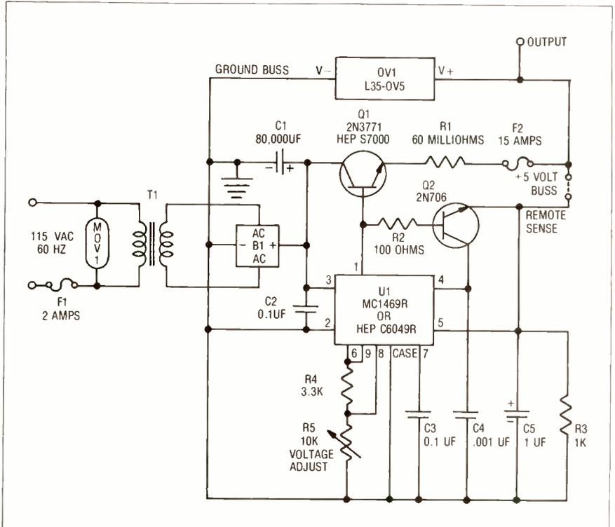
Fig. 12 +5 volts DC, high current power supply
