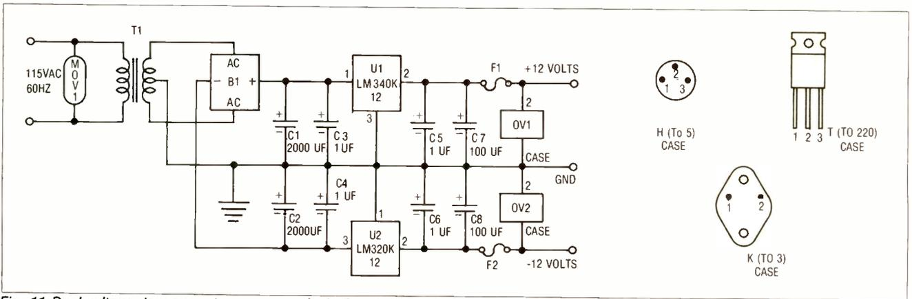
Fig. 11 Dual voltage, low current, power supply A) Circuit, B) typical three-terminal IC regulator case styles.
