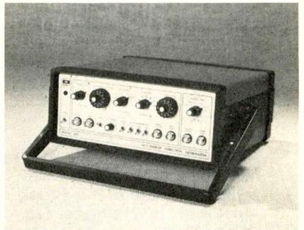
The Model 501 Function Generator by *Exact Electronics* is a sine, square and triangle wave generator with variable symmetry, dc offset, internal ramp, gate and trigger, and start/stop frequency controls. It has a 30v p-p maximum output with 60dB of attenuation in 10dB steps plus 20dB of variable attenuation. It also offers external VCF input, main generator sync output and ramp generator sync output. The price is \$595.
