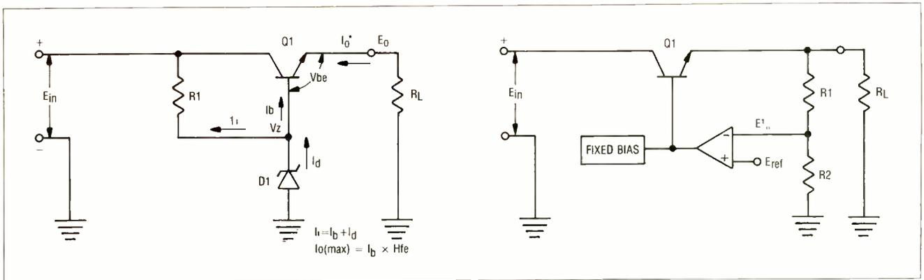
Fig. 9 A) Zener-referenced series-pass regulator B) Feedback Series-pass regulator.
