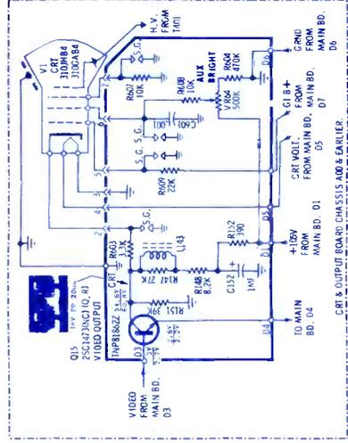
Partial Schematic-CRT & Output Board
