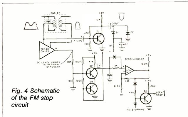
Fig. 4 Schematic of the FM stop circuit
