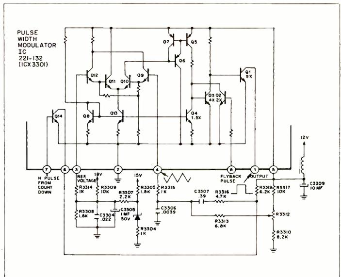
Fig. 6 Schematic of the pulse width modulator IC
