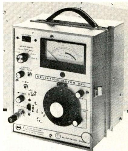
sion oscillator reportedly has low inherent residual frequency modulation. The range of this instrument can be extended below 25MHz by using an external oscillator to heterodyne the transmitter frequency to the 100kHz intermediate frequency. The output system includes a 750 micro-second deemphasis network which allows the Model 920 to be used as a standard test receiver meeting the requirements of EIA Standard RS-152-A. The price of the Model 920 is \$630.00.
