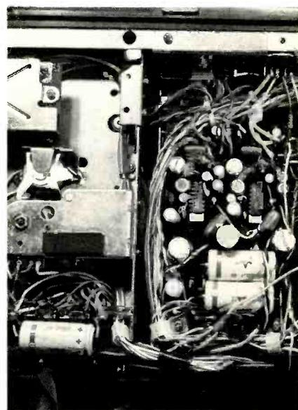
Fig. 4 The audio IC output circuits create a lot of popping or frying noise in the audio channels. It's possible to have two noisy IC components. Be sure and isolate since they are more difficult to remove.
