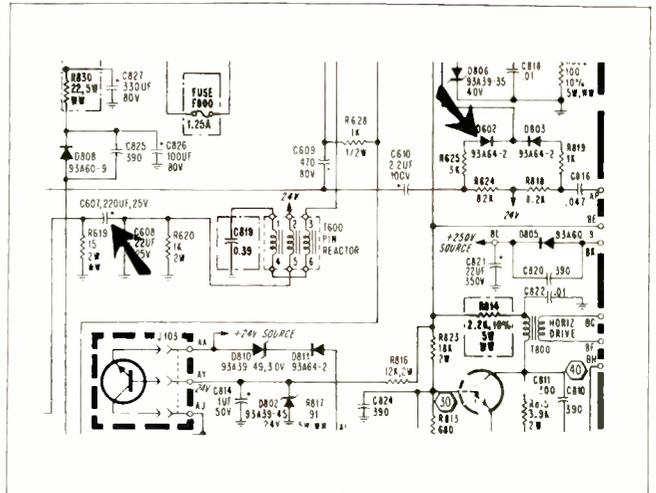
**6. Dark at top, light at bottom, no brightness control.** Possible Cause: Defective D602 (93A64-2).
