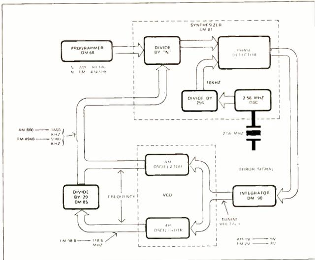
Fig. 2 The tuning system block diagram
