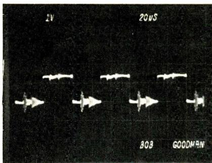
Fig. 8 Correct horizontal pulse to the PWM IC
