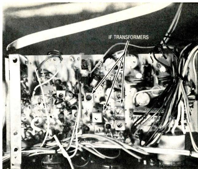
Fig. 7 A noisy IF transformer may be found in some AM-FM-MPX tape player chassis. Isolate the various stages or use signal tracing methods to locate the defective IF transformer.
