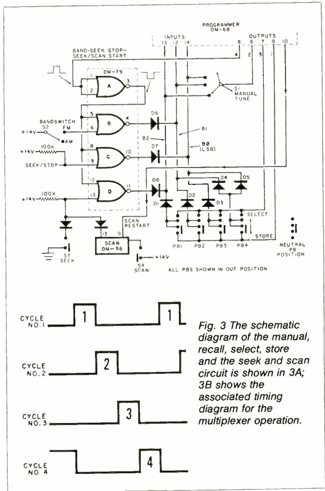
Fig. 3 The schematic diagram of the manual, recall, select, store and the seek and scan circuit is shown in 3A; 3B shows the associated timing diagram for the multiplexer operation.
