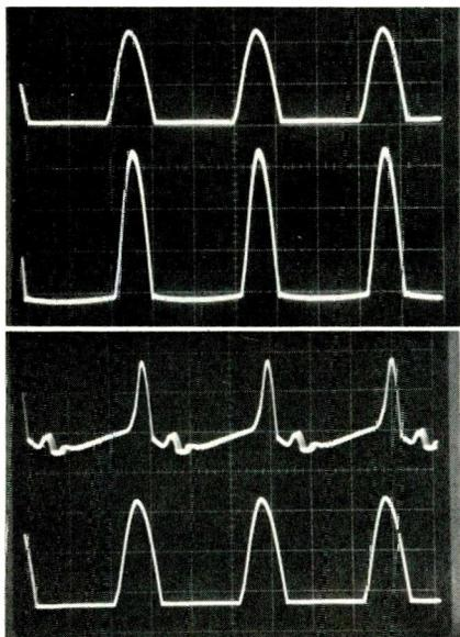
Fig. 10 (A) Top trace indicates shorted yoke compared to good one. (B) Top trace indicates an open yoke taken at 250 volt pulse winding of sweep transformer. Good yoke trace is shown on bottom.
