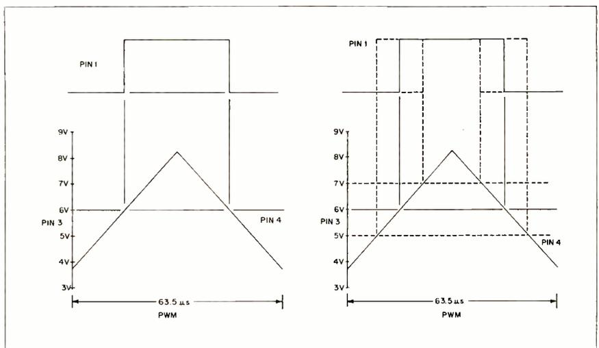
Fig. 7 (A) Transfer characteristics of the pulse width modulator. (B) Variations of the transfer characteristics
