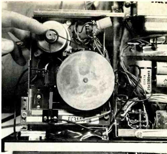
Fig. 5 A defective motor may create both mechanical and electronic noise. Replacement is the correct solution to noise generated in the amplifier by the motor.
