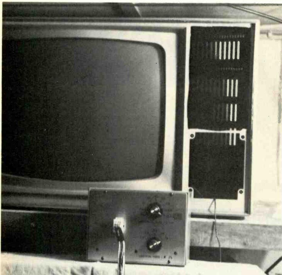
The 10J107 Test Jig Adapter and the defunct TV set that was converted. For information Circle No. 150 on the Reader Service Card.
