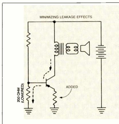
Fig. 3 A modified circuit to reduce leakage currents. Here a low ohmage shunt across the base-emitter junction draws off the transistor's junction leakage. Notice the added emitter resistor.
