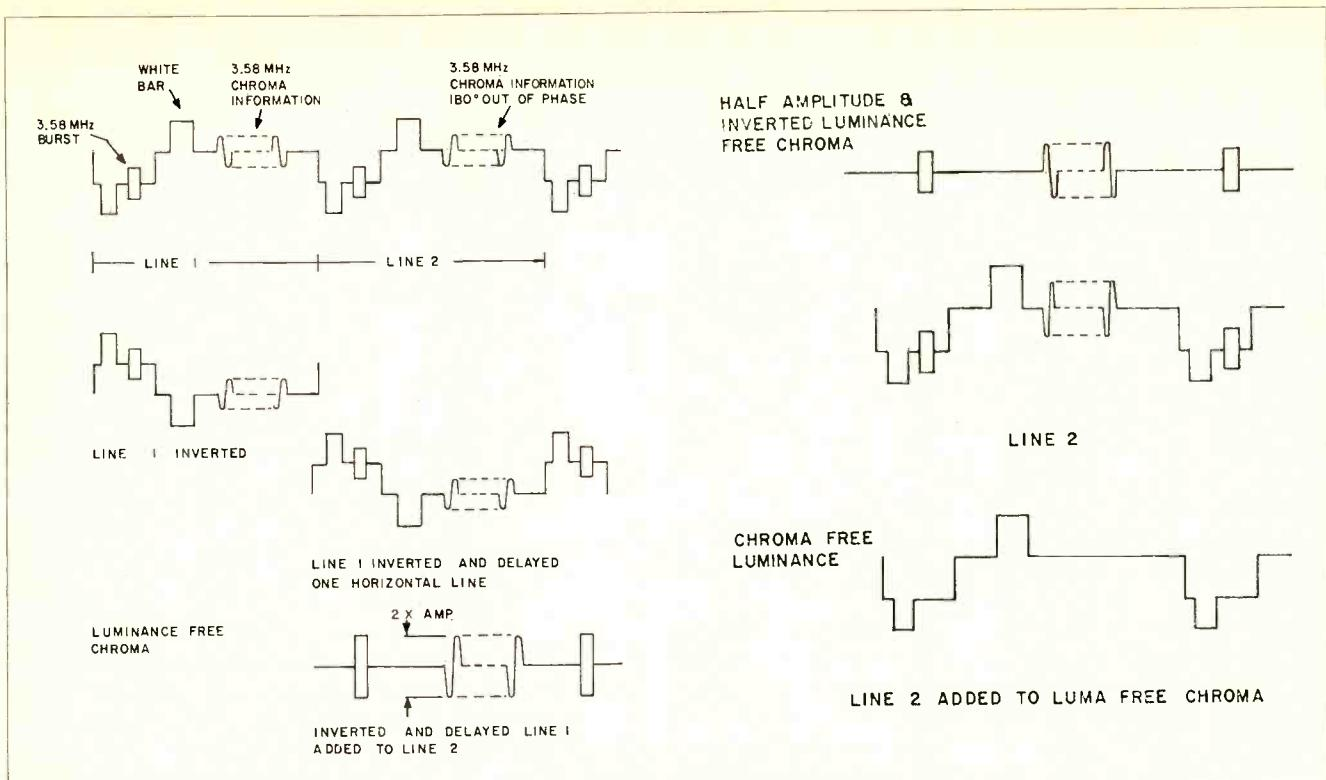
Fig. 4 & 5 How the comb filter works. Two separate functions, the separation of luminance from the chroma information (figure 4), and the separation of chroma from the luminance channel, are performed by the comb filter and delay line circuitry.
