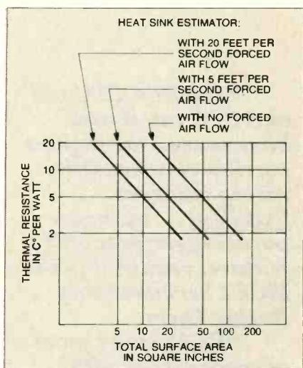
Fig. 1 Heat Sink Estimator: a useful graph for estimating a heat sink's ability. This chart is applicable to a single flat aluminum plate at least 1/16 inch thick. A black finish would improve the heat sink's performance by about 10 per cent.
