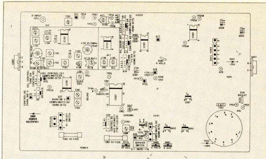
*Fig. 7 The main component location chart for Quasar's newest 19-inch chassis.*
