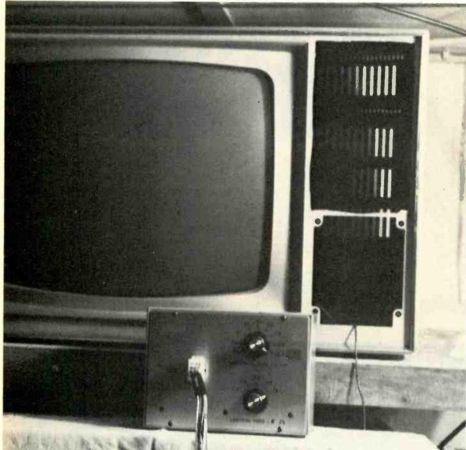
The 10J107 Test Jig Adapter and the defunct TV set that was converted. For information Circle No. 150 on the Reader Service Card.
