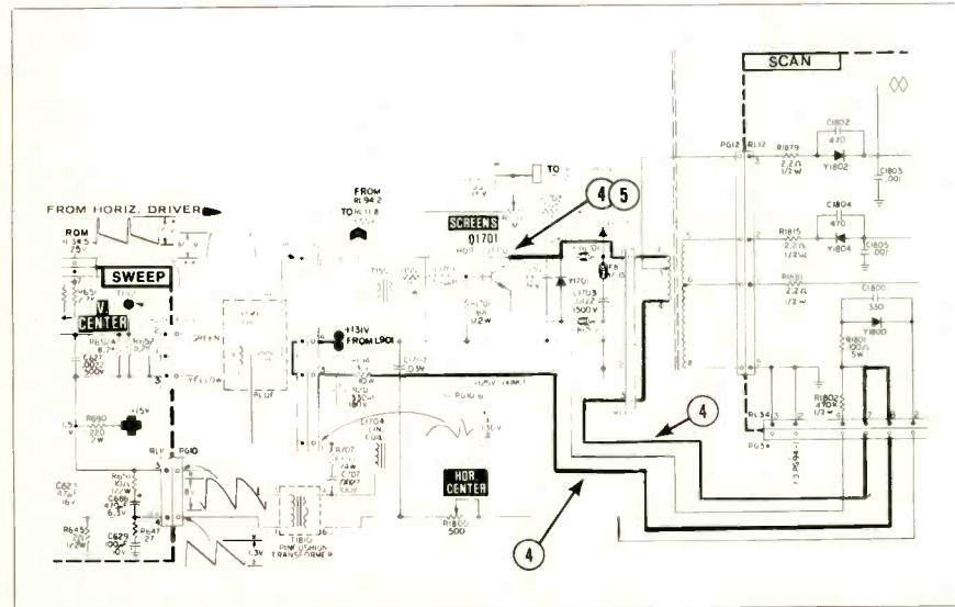
*Fig. 4. Horizontal output circuit.*
