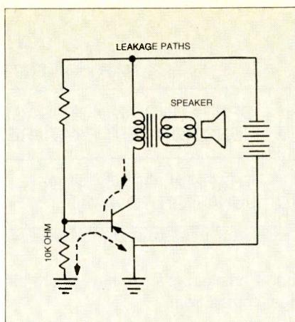
Fig. 2 A basic transistor circuit with typical leakage paths indicated by the dotted lines.
