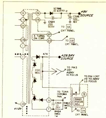
Fig. 1 A new flyback transformer, all solid state, is part of the new E51 and 53 chassis. A special high voltage sensing circuit causes automatic shutdown when the latter exceeds specified limits.
