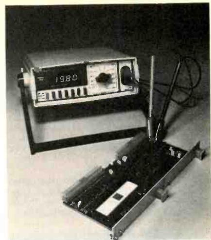
power line, 2 Amp input and a 3 Amp high energy type. Forty-eight-inch long insulated safety test leads with screw-on insulated alligator clips, combination carrying handle/bench stand, plus a 3-wire detachable long line cord are also furnished. Power requirements are 50/60Hz, 120 or 240 Vac with internal change. Optional accessories include miniature clip leads for high density circuits and a 30 amp dc current shunt. The price is \$235.
