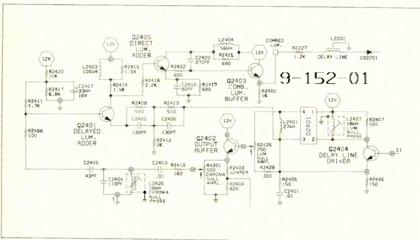
Fig. 3 The schematic diagram for Zenith's comb filter circuitry.
