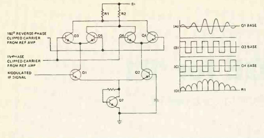
Fig. 8 GE has replaced all diode detectors with synchronous versions in the video, sound and AFT circuits.
