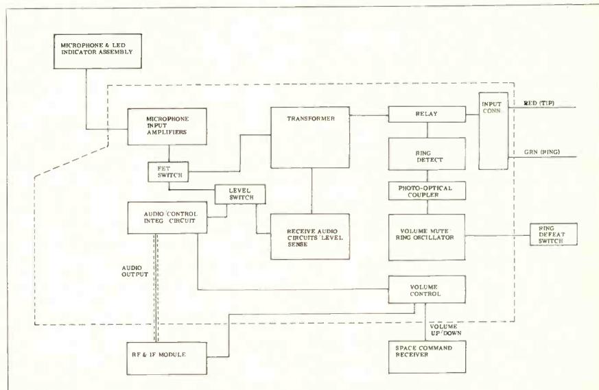
Fig. 6 The block diagram of Zenith's new "Space Phone" telephone answering and transmitting system.
