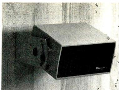
pattern, the unit has an LED umbilical wire "walk test" feature that tucks away inside the sensor during normal operation. The self-contained unit operates from 16.5 volt ac power and has a back-up battery if primary power fails. Electrical interference problems are said to have been eliminated by enclosing the sensor in a metal die cast case. The Model 20000-04 is offered with a one year limited factory warranty.
