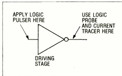
Fig. 18. Using a logic probe and a current tracer.
