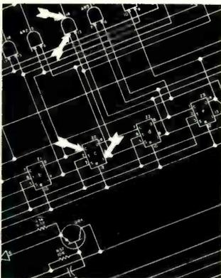
**On the cover:** Digital troubleshooting—in simplest terms, pulsing the input of a gate with a logic pulser and monitoring the output with a logic probe or a current probe—is the subject of our cover and our major feature.
