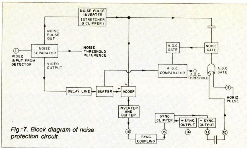
Fig. 7. Block diagram of noise protection circuit.
