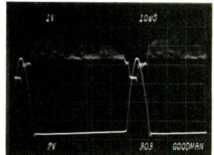
Fig. 9. Dual-trace scope indicates correct timing of the horizontal keying pulse.
