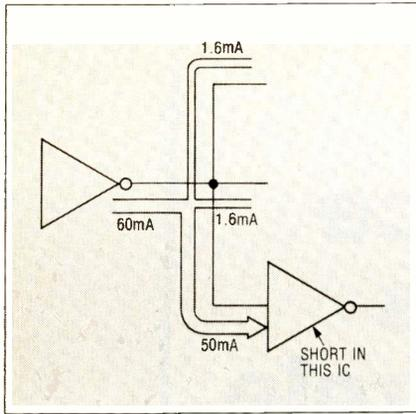
Fig. 15. Current tracing to a short circuit
