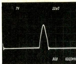
Fig. 3. Horizontal keying pulse.
