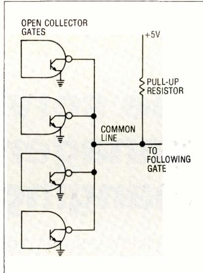
Fig. 17. The "Wired OR" circuit.
