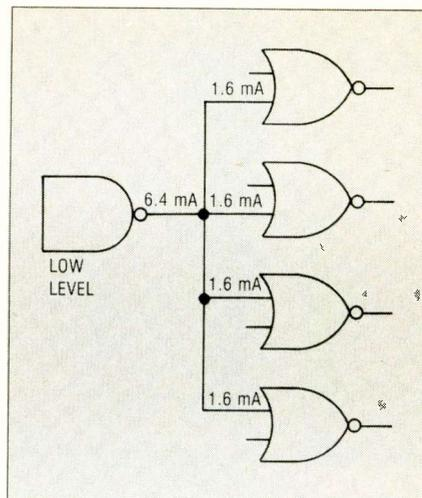
Fig. 13. Output current in a TTL circuit
