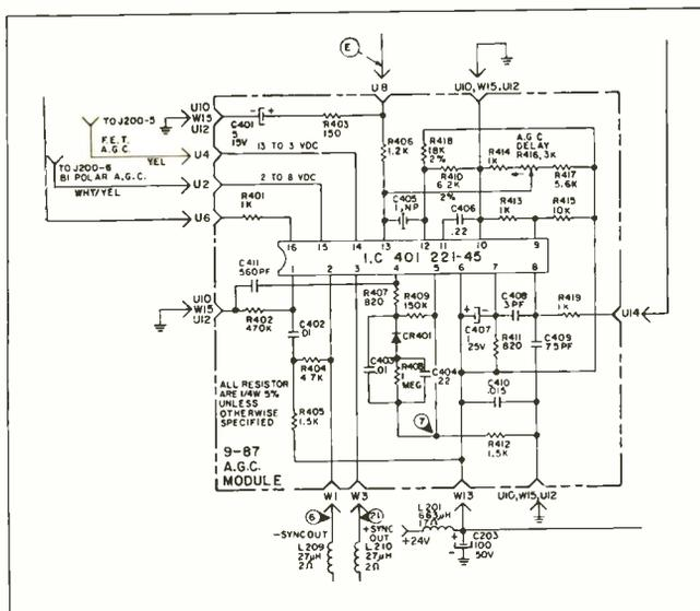
Fig. 2. The 9-87 module circuit.
