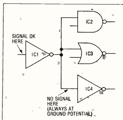
Fig. 14. Problems in isolating a short circuit.
