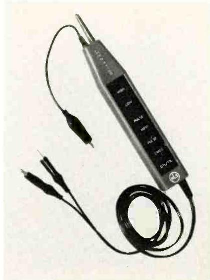
Fig. 6. A logic probe by Non-Linear Systems.
