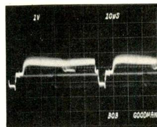
Fig. 4. Composite video signal.
