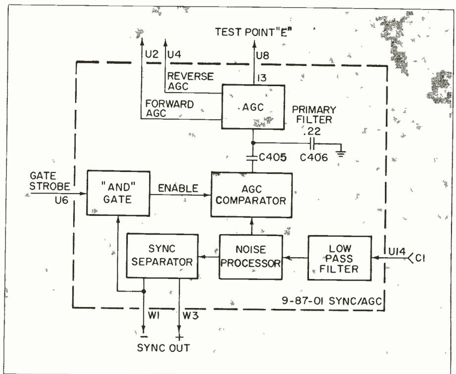
Fig. 1. Functional block diagram of the 9-87 module.
