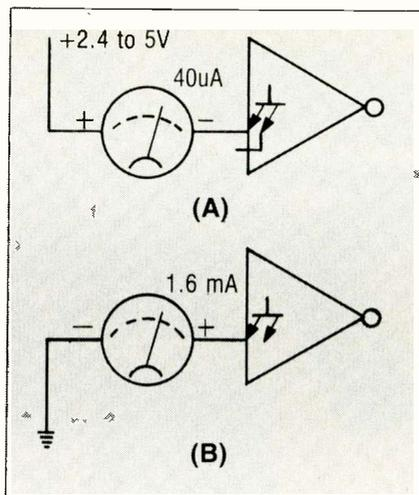
Fig. 12. Currents in TTL input circuits.
