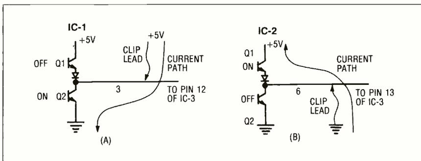
Fig. 4. Problems in trying to force an IC pin high or low.
