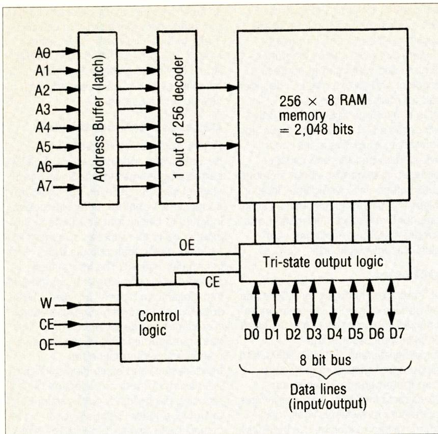
Fig. 2. Block diagram of a memory with full decoding and tri-state logic outputs. Note: "W" denotes read/write input; "CE" is chip enable input; and "OE" is tristate output enable input.
