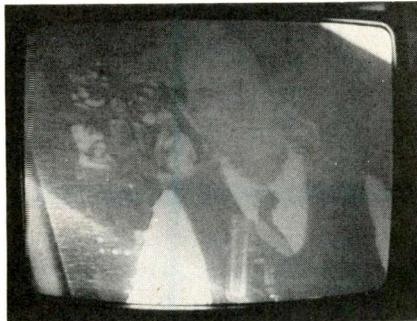
Fig. 11. Picture weave and roll symptoms found only on local cable channels received via satellite.
