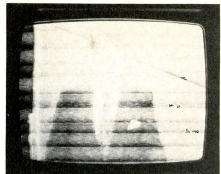
Fig. 8. Streaks caused by open filter capacitor at +24 volt input at pin W13.
