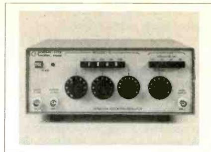
vernier to provide total dynamic range of 90dB. Precise frequency selection is possible with the 3 digit tuning selector. Simultaneous inverted (180°) and quadrature (90°) outputs also are provided. Each output is 7V RMS with 600 ohm source impedance. When combined with a distortion analyzer, such as the Krohn-Hite 6800 series, it provides a complete distortion measurement system. The 4400 is priced at \$550; availability is 60 days.
