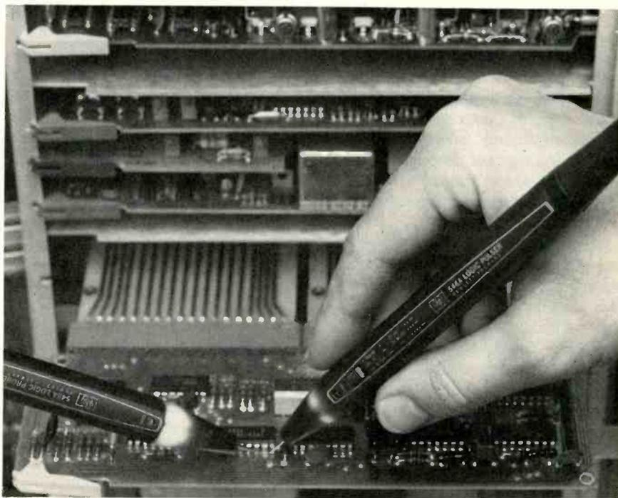
Fig. 1. Using a logic pulser and a logic probe (courtesy of Hewlett-Packard).
