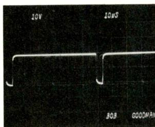
Fig. 5. Horizontal sync pulses.
