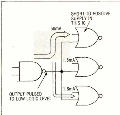
Fig. 16. Locating a short to the positive supply line.
