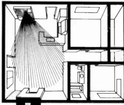
Fig. 1. The invisible, directional microwave beam is adjustable up to 50 feet for large area protection in the home.
