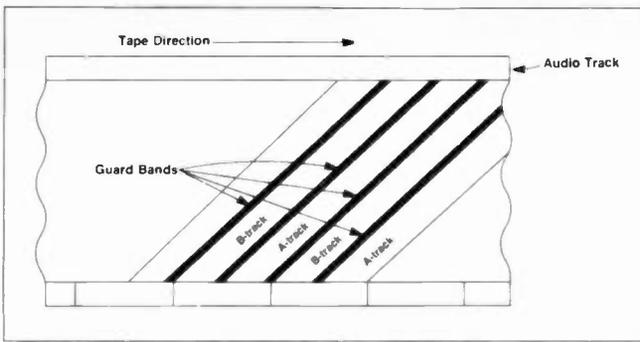
The helical scan recorder records alternate A- and B-tracks separated by guard bands. These guard bands prevent the signals recorded on one track from interfering with those recorded on a neighboring track. Interference between tracks is called crosstalk.
