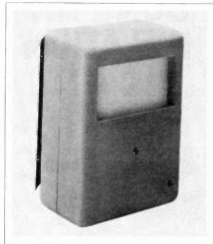
walking under the pattern is prevented. The no. 651 has its main zone reaching to 100 feet, two intermediate zones to 60 feet and three short zones out to 12 feet. Both models are reportedly designed so that temperature and incidental infrared energy does not set off the alarm. Both models provide multi-function LED, memory, silent relay and high LED disable functions when combined with the appropriate controls. **ETD**
