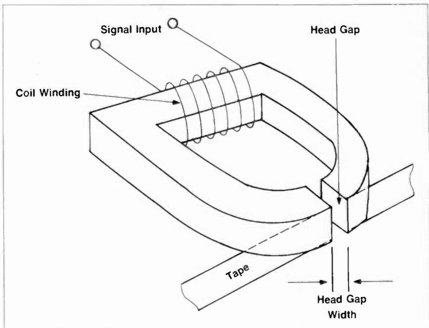
*A recording head resembles a split u-ring in shape. The split in the u-ring is called the head gap. During recording, the head becomes an electromagnet. Magnetic flux lines develop at the head gap and magnetize the ferro-magnetic particles in the recording tape.*
