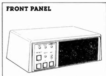
Fig. 3. The front panel with the push-button controls of the Midex-55 burglar alarm system.
