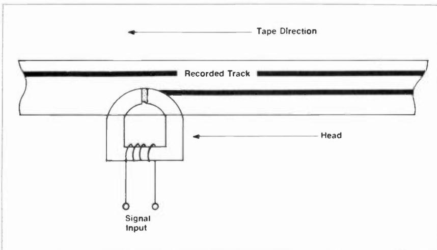
Audio recorders record signals parallel to the tape edges and along the entire length of the tape. This is longitudinal recording.
