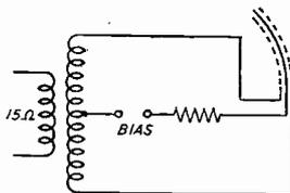
Theoretical representation of a push-pull electrostatic loudspeaker.
