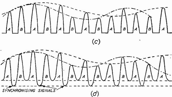
Fig. 2: Basic waveforms of the system. (a) Sampled audio wave A, (b) sampled audio wave B, (c) complex signal waveform obtained as a result of adding the two sampled audio waves A and B, (d) filtered complex signal waveform with synchronisation pulses.
