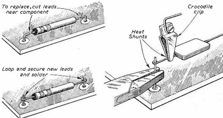
Fig. 2: Details of removing and reconnecting components, as described in the text.
