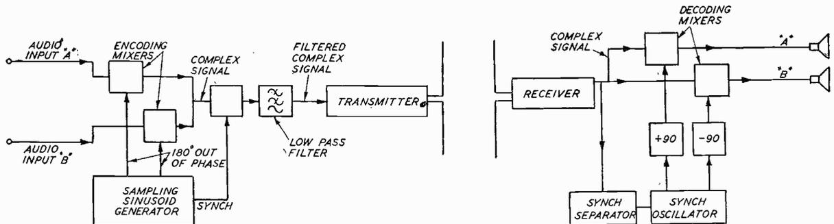
Fig. 1: Block schematic diagrams of the time multiplex system. On the left, the transmitter arrangement. On the right, the receiver arrangement.
