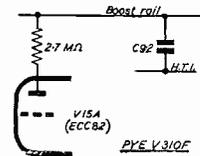
Investigation found that the capacitor C92 (0.05μF) was short circuit. Replacing C92 restored the boost rail to 500V and with it normal frame amplitude. This fault has occurred on several receivers of this type. C92 is easily replaced on removing the panel underneath the receiver.—G.B., Oxford (647).
