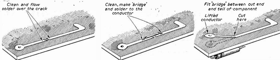
Fig. 1: Details of bridging breaks in conductors.
