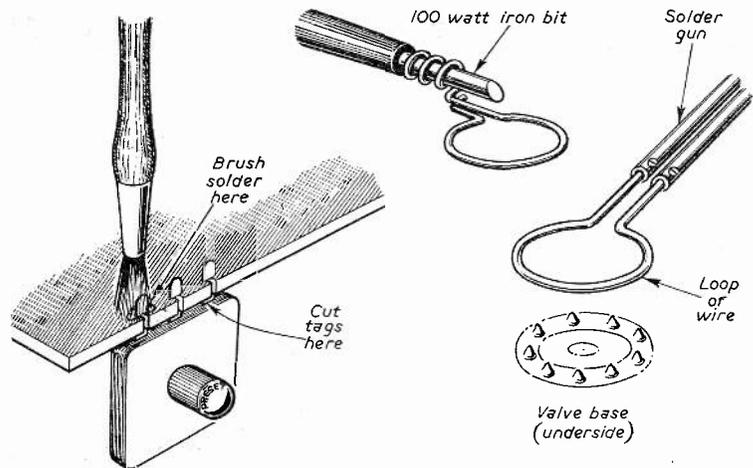
Fig. 3: Methods of removing tagged controls and valve bases.
