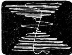
The trace started at the centre of the oscillatory period, damped down towards the centre of the screen with a single bright sinusoidal trace before starting to oscillate again. The trace ended at the point of maximum oscillator amplitude, followed by a very bright S-shaped flyback from bottom to top of screen (see diagram).
