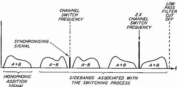
Fig. 3 (left): Spectral content in the complex signal.
