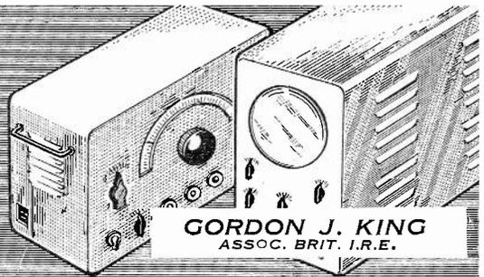
**I**N addition to the signal generator, which was dealt with last month, life is made much easier for the practicing service technician if he has available, for immediate action, a generator for producing a locked pattern on the screen of a television receiver.
