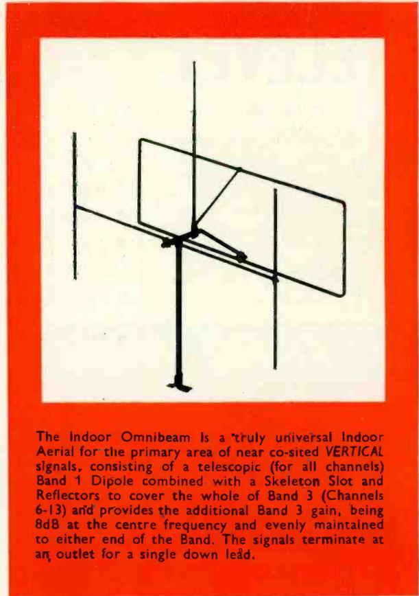
The Indoor Omnibeam is a "truly universal Indoor Aerial for the primary area of near co-sited VERTICAL signals, consisting of a telescopic (for all channels) Band 1 Dipole combined with a Skeleton Slot and Reflectors to cover the whole of Band 3 (Channels 6-13) and provides the additional Band 3 gain, being 8dB at the centre frequency and evenly maintained to either end of the Band. The signals terminate at an outlet for a single down lead.
