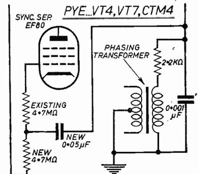
A positive cure for this is to change the grid resistor to the sync separator for two 4.7M $\Omega$  resistors in series, instead of one single 4.7M $\Omega$  resistor. The junction of the two resistors is taken via an additional 0.05 $\mu$ F capacitor to the junction of the 0.001 $\mu$ F capacitor and 2.2M $\Omega$  resistor which are across the phasing transformer. All other components remain as before.
