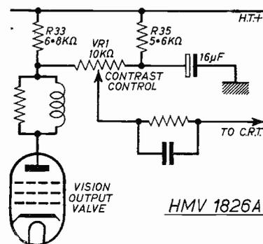
contrast control in a rather complex arrangement around the video amplifier stage. The anode voltage for this valve was checked and thought to be somewhat low, but this was dismissed as of little consequence.
