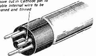
To effect a repair, a small groove was carefully filed into the cathode pin at a position approximately one third of the length from the tube end. This exposed the internal connecting wire, which was carefully cleaned and the complete groove filled in with solder and finally cleaned to the original pin diameter. This effected a complete cure.—J.E.R., Nottingham (921).
