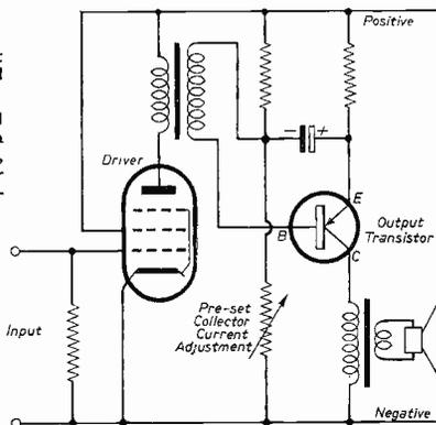
The emitter in this case can be likened to the cathode of a triode, the base to the control grid and the collector to the anode.
